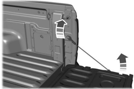
3. Raise the tailgate slightly to allow slack in the tailgate cables and unlatch them.
