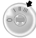
3. Turn the key to position III and wait until the engine stops cranking.
