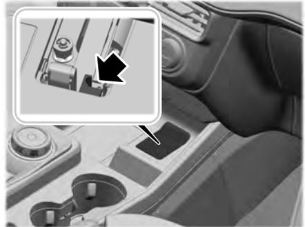
1. Once it is safe to do so, reconnect the negative battery cable to the battery.
