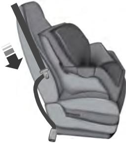
2. After positioning the child restraint in the proper seating position, pull down on the shoulder belt and then grasp the shoulder belt and lap belt together behind the belt tongue.
