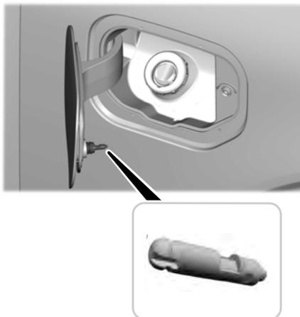
Using the emergency opening tool can cause the tappet to temporarily dislodge from the fuel filler door and remain attached to the fuel filler door opening. If you press the fuel filler door release button after using the emergency opening tool, locate the tappet and reinsert it into the fuel door.
