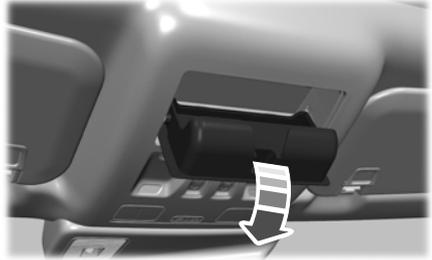
The glasses holder is in the overhead console. Press near the rear edge of the door to open.
