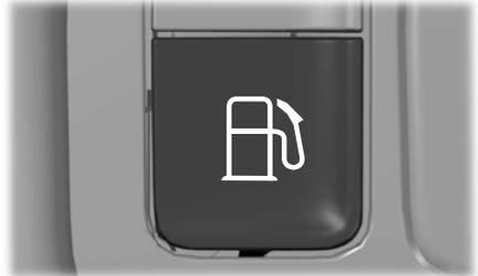
2. Press the button on the left side of the instrument panel next to the headlamp switch to open the fuel filler door. The fuel filler door can take up to 15 seconds to open before you can insert a fuel filler nozzle.
