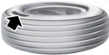
Tire Quality Grades apply to new pneumatic passenger car tires. The Quality grades can be found where applicable on the tire sidewall between tread shoulder and maximum section width. For example: **Treadwear 200 Traction AA Temperature A.**
