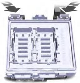
4. Pull both latches toward you and remove the fuse box.
