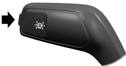
To activate the system, press the button on the turn signal lever.
