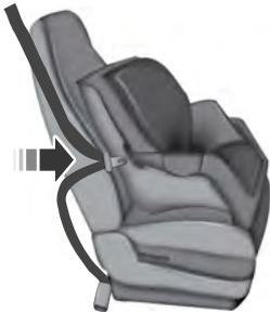
3. While holding the shoulder and lap belt portions together, route the tongue through the child restraint according to the child restraint manufacturer's instructions. Make sure that you did not twist the belt webbing.
