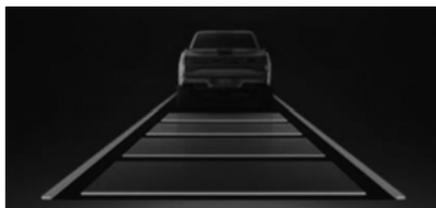
The selected gap appears in the instrument cluster display as shown by the bars in the image.
