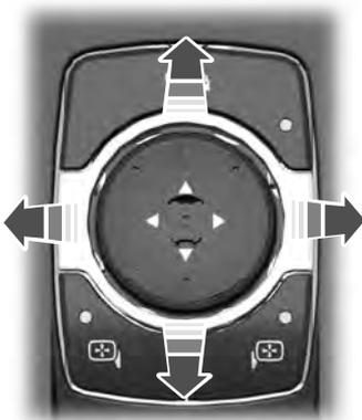
To adjust your mirrors, switch your vehicle on, with the ignition in accessory mode or the engine running.
