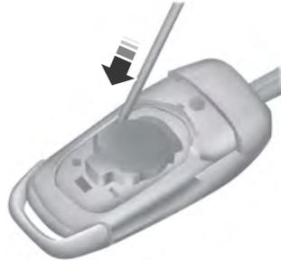
4. Insert a screwdriver as shown to release the battery.
