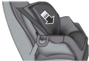
5. To put the retractor in the automatic locking mode, grasp the shoulder portion of the belt and pull downward until you pull all of the belt out.
