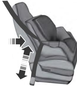
10. Before placing the child in the seat, forcibly move the seat forward and back to make sure the seat is securely held in place. To check this, grab the seat at the belt path and attempt to move it side to side and forward and back. There should be no more than 1 in (2.5 cm) of movement.
