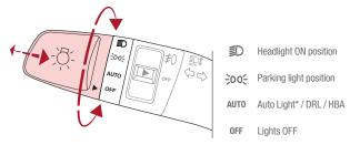
**AUTO Light\*** — When the light switch is in the AUTO Light position, the tail lights and headlights will turn ON/OFF automatically, depending on the amount of light outside the vehicle.
