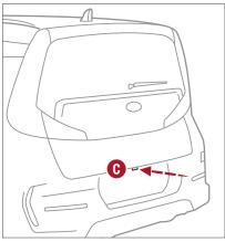
(Button is located underneath the Liftgate lid)
