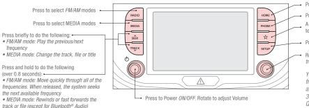
Audio System Setup Options - Press the SETUP key, then using the touchscreen, press the menu item to enter (Display, Sound, Clock/ Calendar, Phone, System Info). Adjust the available settings for each equipped audio system setup option by pressing the onscreen buttons/arrows. Audio system setup options may include the following:
