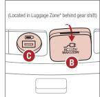
**AUX/Multimedia USB Port**  — Use the AUX port to connect audio devices and the Multimedia USB port to connect USB audio devices and smartphones.
