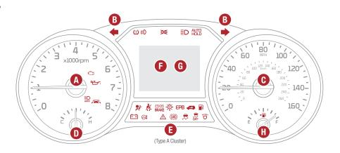
Your vehicle's instrument cluster & indicator light locations may differ from those in the illustrations. For more information on the instrument cluster, the LCD Warning Messages and the function of all indicator and warning lights, please refer to section 2 in the Owner's Manual.
