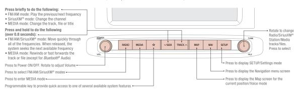
**Sound Settings:** To adjust the sound settings (Fader/Balance, Tone, Touch-Screen Beep ON/OFF and Speed-Dependent Volume Control ON/OFF) from any audio mode:
