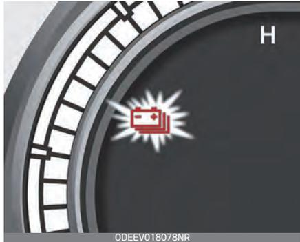
2. When the warning lamp turns ON, the vehicle can drive an additional 12~18 miles (20~30 km) depending on the driving speed, heater / air conditioner, weather, driving style, and other factors. Charging is required.
