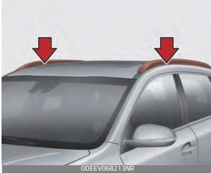
Crossbars and fixing components can be installed on the roof rack to carry cargo. Those may be obtained from an authorized Kia dealer or other qualified shop.
