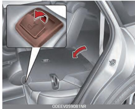
5. To use the rear seat, lift and pull the seatback backward by lifting up seatback. Pull the seatback firmly until it clicks into place. Make sure the seatback is locked in place.
