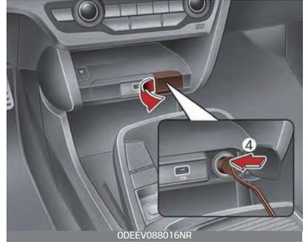
7. Connect between compressor and the vehicle power outlet (4) using the cable and connectors.
