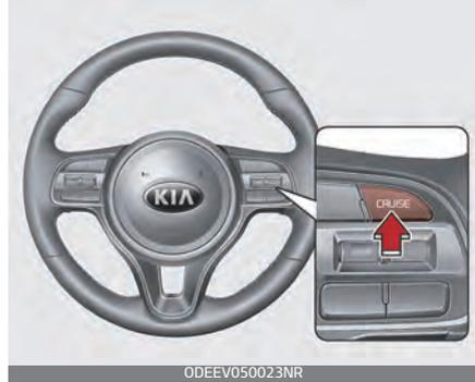
2. Accelerate to the desired speed. Smart Cruise Control speed can be set as follows:
