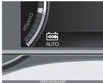
If the front radar recognizes the vehicle in front, 'AUTO' is displayed in blue. The regenerative braking level is automatically controlled
