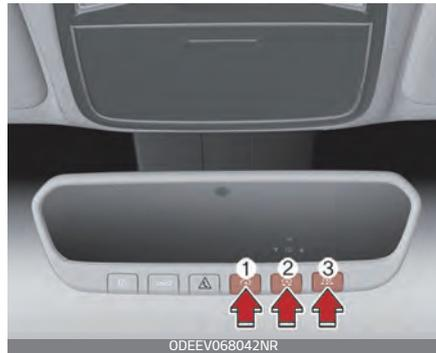
4. Once the garage door is stopped, press and release the "Lean" or "Smart" button on the Garage door opener within 1 minute from the time of pressing the programmed HomeLink button on mirror.
