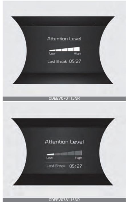
The driver's attention level is displayed on the scale of 1 to 5. The lower the level is, the more inattentive the driver is.
