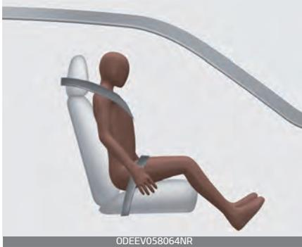
When an adult is seated in the front passenger seat, if the PASSENGER AIR BAG "OFF" indicator is on, change POWER button to the OFF position and ask the passenger to sit properly (sitting upright with the seatback in an upright position, centered on the seat cushion with their seat belt on, legs comfortably extended and their feet on the floor). Restart the vehicle and have the person remain in that position. This will allow the system to detect the person and to enable the passenger air bag.
