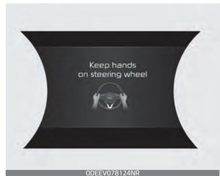
If the driver keeps hands off the wheel even with the hands-off warning on, the steering assist is temporarily released automatically.
