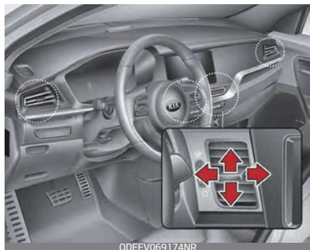
The outlet vents can be opened or closed separately using the thumb-wheel. (if equipped)
