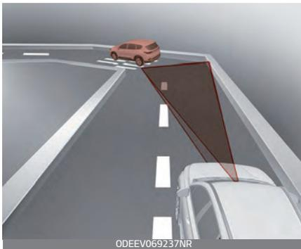
On curves, Smart Cruise Control may not immediately detect a moving vehicle in your lane, and then your vehicle could accelerate to the set speed. Also, the vehicle speed
