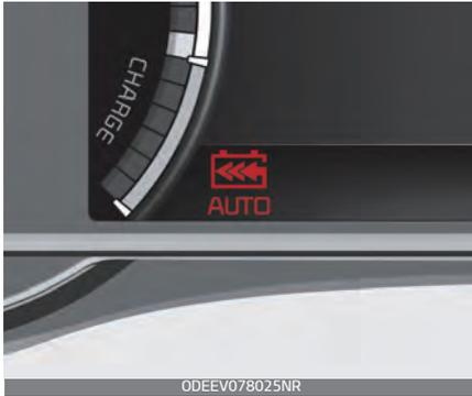
However, current regenerative braking level is maintained if the driver depresses the brake pedal while the system is in activation. Also, the system is cancelled temporarily if the accelerator pedal is depressed.
