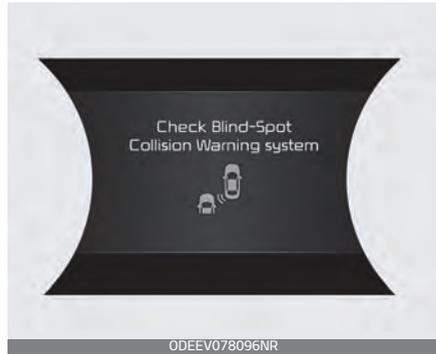
If there is a problem with BCW, a warning message will appear and the light on the button will turn off. The function will turn off automatically. RCCW will not operate also if BCW turns off due to malfunction. Have your vehicle inspected by an authorized Kia dealer.
