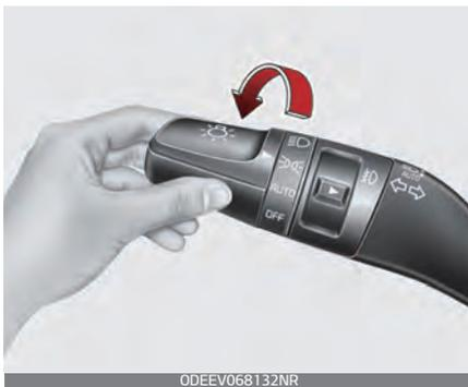
When the light switch is in the parking light position, the tail, license and instrument panel lights will turn ON.
