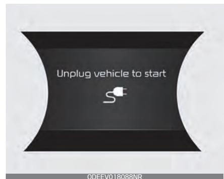
This message is displayed when you start the vehicle, without unplugging the charging cable, and will not shift out of park. Unplug the
