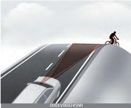
The performance of Forward Collision-Avoidance Assist may be decreased while driving upward or downward on a slope. The front camera or front radar sensor recognition may not detect the vehicle, pedestrian or cyclist in front.
