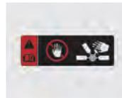
The electric motor (cooling fan) is controlled by coolant temperature, refrigerant pressure and vehicle speed. It may sometimes operate even when the vehicle is not operating. Use extreme caution when working near the blades of the cooling fan so that you are not injured by a rotating fan blades. As the coolant temperature decreases, the electric motor will automatically shut off. This is a normal condition.
