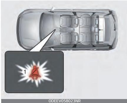
If the driver continues not to fasten the seat belt, the warning light will stay illuminated and the warning chime will sound for approximately 6 seconds until the belt is fastened each time the POWER button is in ON. This will happen every time the POWER button is in ON.
