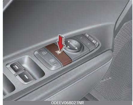
When the power window lock switch is pressed:
