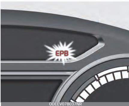
If the EPB malfunction indicator remains on, comes on while driving, or does not come on when the POWER button is changed to the ON position, this indicates that the EPB may have malfunctioned.
