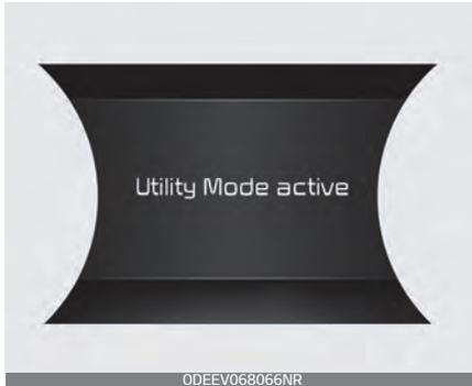
When driving is not necessary such as while camping or when stopping the vehicle for a long time, it is possible to use the electrical devices (audio, lights, etc.) for long hours.
