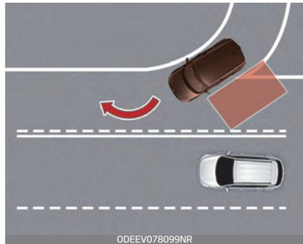
BCW may not operate properly when driving where the road is merging/dividing. In certain instances, the function may not detect the vehicle in the next lane.
