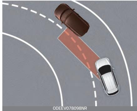
BCW may not operate properly when driving on a curved road. In certain instances, the function may recognize a vehicle in the same lane.
