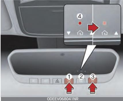
1. Press and hold the button (1) and (3) simultaneously.
