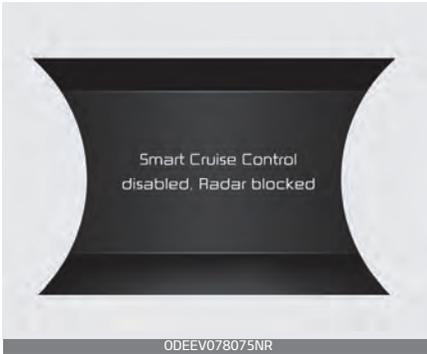
When the sensor cover is blocked with dirt, snow, or debris, Smart Cruise Control operation may stop temporarily. If this occurs, a warning message will appear on the LCD display. Remove any dirt, snow, or debris and clean the radar sensor cover before operating Smart Cruise Control. Smart Cruise Control may not properly activate, if the radar is totally contaminated, or if any substance is not detected after turning ON the vehicle (e.g. in an open terrain).
