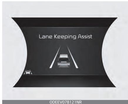
If the speed of the vehicle is over 40 mph (64 km/h) and the function detects lane markers, the color changes from gray to white.
