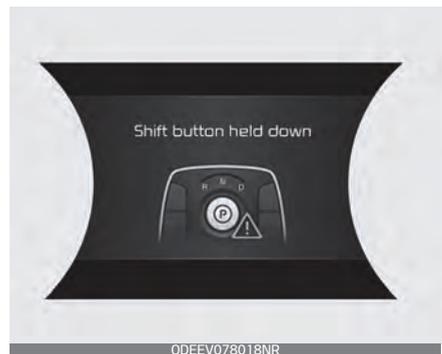
The message appears on the LCD display when the shifter button is continuously pressed or there is problem with the button.
