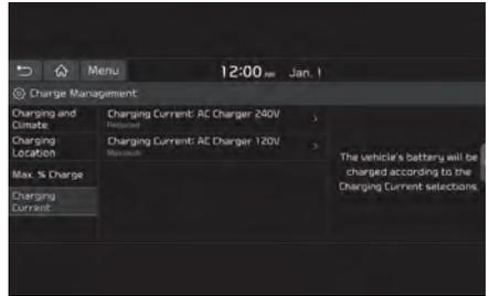
If the charging process does not start or abruptly stops in the middle, re-select another proper current and retry charging the vehicle.
