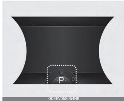
The shift indicator pop-up function can be activated or deactivated from the User Settings mode in the cluster LCD display.
