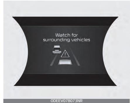
If the vehicle ahead (vehicle speed: less than 20 mph (30 km/h) moves to the next lane, the warning chime will sound and a message will appear. Adjust your vehicle speed for vehicles or objects that can suddenly appear in front of you by depressing the brake pedal according to the road and driving conditions.
