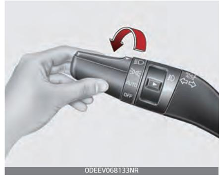
When the light switch is in the headlight position, the head, tail, license lights will turn ON.
