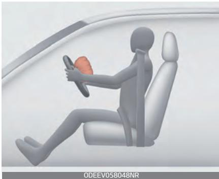
The front air bag modules are located both in the center of the steering wheel and in the front passenger's panel above the glove box. When the SRSCM detects a sufficiently severe impact to the front of the vehicle, it will automatically deploy the front air bags.
