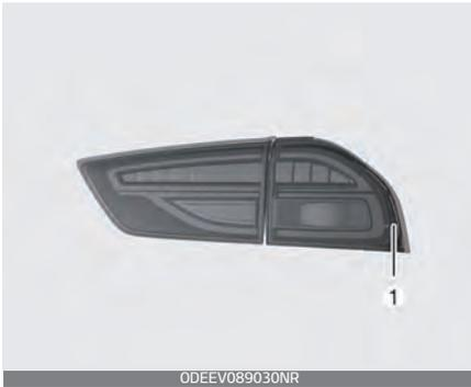
If the rear side marker (LED type) (1) does not operate, have the vehicle checked by an authorized Kia dealer.
