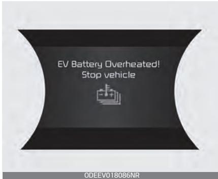
This warning message is displayed to protect battery and electric vehicle system when the high voltage battery temperature is too high.
