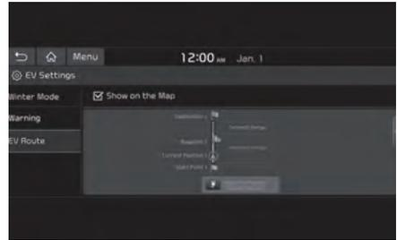
You can apply electric car-related functions for guiding the route. It allows you to check the distance that you can go with the current battery amount. Travelable and non-travelable sections on your way to the destination are displayed on the screen. The search station icon is also displayed so that you can find nearby stations immediately.
