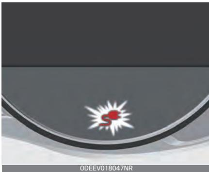
Charging does not occur when the charging indicator lamp is OFF. When the charging connector and charging plug are not connected properly, reconnect the charging cable to charge.
