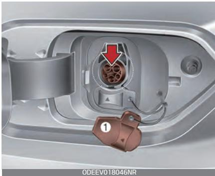
7. Open the protective cover of the charging connector and check if there is dust on the charging connector and charging inlet.
