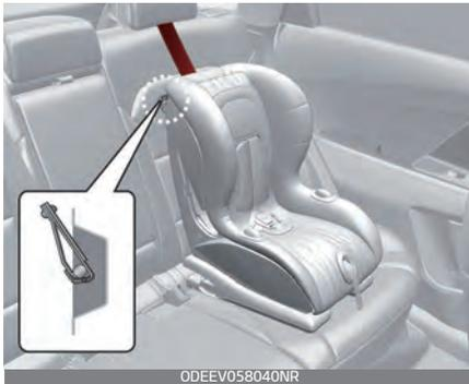
1. Route the child restraint tether strap over the child restraint seatback. Route the tether strap under the head restraint and between the head restraint posts, or route the tether strap over the top of the vehicle seatback. Make sure the strap is not twisted.
