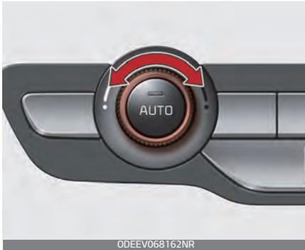
The temperature will increase to the maximum (82 °F) by turning the knob to the extreme right.
