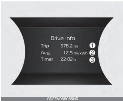
This display shows the trip distance (1), the average energy consumption (2), and the total driving time (3).
