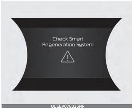
The message will appear when the system is not functioning normally. The system will be cancelled and the word 'AUTO' on the cluster will disappear and instead display regenerative braking level. Check for foreign substances on the front radar. Remove any dirt, snow, or foreign material that could interfere with the radar sensors. If the system still does not operate normally, take your vehicle to an authorized Kia dealer and have the system checked.
