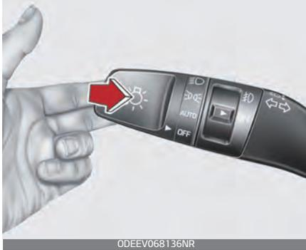
It will return to the normal (low beam) position when released. The headlight switch does not need to be on to use this flashing feature.
