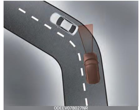
When driving on the curve, the system may not detect the vehicle in your lane and the regenerative braking level will reduce automatically, making you feel that the vehicle is accelerating.
