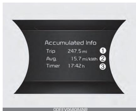
This display shows the accumulated trip distance (1), the average energy consumption (2), and the total driving time (3).
