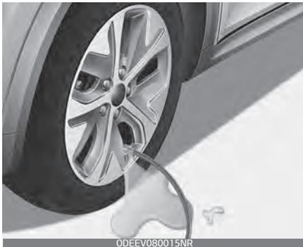
If the sealant is injected when the tire air pressure injection valve and sealant injection hose are not fully
