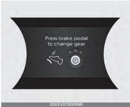
The message appears on the LCD display, when the brake pedal is not depressed while shifting the gear.
