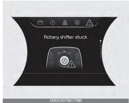
The message appears on the LCD display when the shifter dial is continuously stuck or there is problem with the shifter dial.
