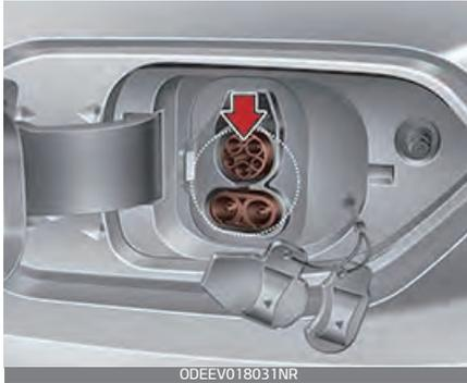
5. Check whether there is dust or foreign substances inside the charging connector and charging inlet.
