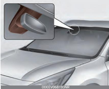
The auto defogging system operates when the heater or air conditioning is on.
