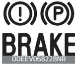
Before driving, be sure the parking brake is fully released and the brake warning light is off.
