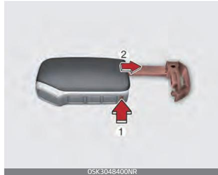
To reinstall the mechanical key, put the key into the hole and push it until a click sound is heard.
