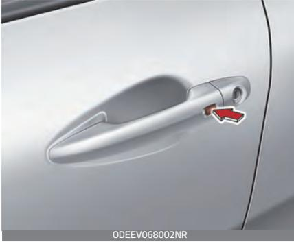
Pressing the button of the front outside door handles with all doors (and liftgate) closed and locked, locks all the doors (and liftgate).
