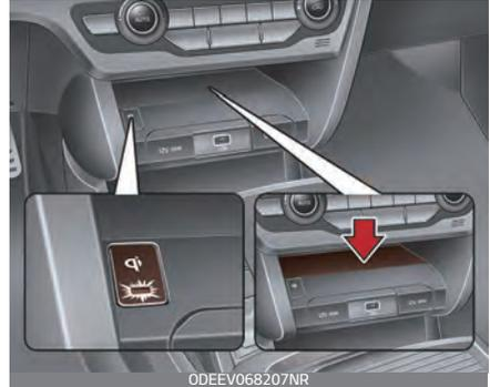
Firmly close all doors, and turn vehicle on. To start wireless charging, place the smart phone equipped with wireless charging function on the wireless charging pad.
