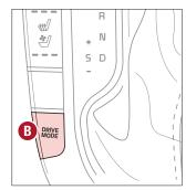
(Located on Center Panel next to Gear Shift)\*
