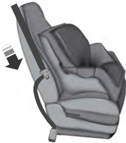
2. After positioning the child restraint in the proper seating position, pull down on the shoulder belt and then grasp the shoulder belt and lap belt together behind the belt tongue.
