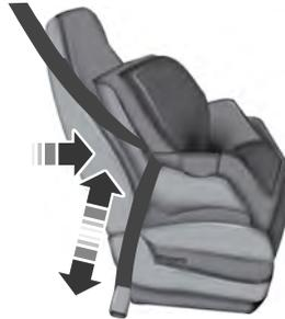
10. Before placing the child in the seat, forcibly move the seat forward and back to make sure you have the seat securely held in place. To check this, grab the seat at the belt path and attempt to move it side to side and forward and back. There should be no more than 1 in (2.5 cm) of movement for proper installation.
