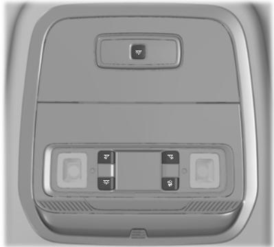
The front interior lamp switches are on the overhead console.
