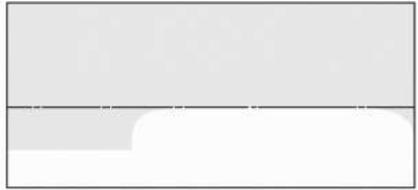
4. On the wall or screen you will observe a flat zone of high intensity light located at the top of the beam pattern. If the top edge of the flat zone of high intensity light is not on the horizontal reference line, adjust the aim of the headlamp beam.
