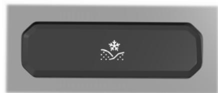
Press the drive mode button underneath the information display to select or change a drive mode.
