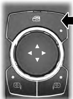
Press the control to lock or unlock the rear window controls. It illuminates when you lock the rear window controls.
