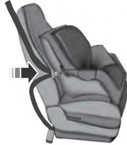
3. While holding the shoulder and lap belt portions together, route the tongue through the child restraint according to the child restraint manufacturer's instructions. Make sure you do not twist the belt webbing.
