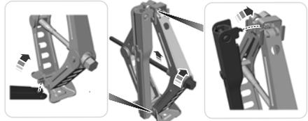
1. To store the folded wrench on the jack, engage the bracket of the jack base and the lug wrench pin, swing the wrench upwards, adjust jack height until the wrench hook engages the hole on jack. Tighten the hex nut clockwise by hand until secure.
