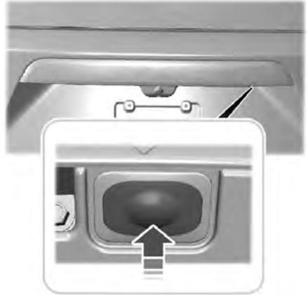
Press the control button to the right of the rear view camera to unlatch the liftgate and then lift to open.
