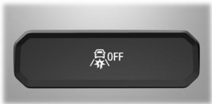
You can switch the entire system off at any time by pressing the button below the display screen.
