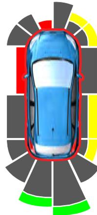
The system provides an image of your vehicle and the sensor zones. The zones highlight green, yellow and red when the parking aid sensors detect an object in the coverage area.
