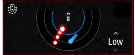
Once the system detects approaching objects crossing the selected range perimeter, the vehicle sounds a tone, and may roll up the windows and lock the doors.
