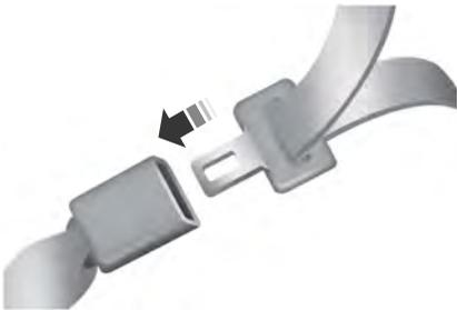
1. Insert the belt tongue into the proper buckle (the buckle closest to the direction the tongue is coming from) until you hear a snap and feel it latch. Make sure that you securely fasten the tongue in the buckle.
