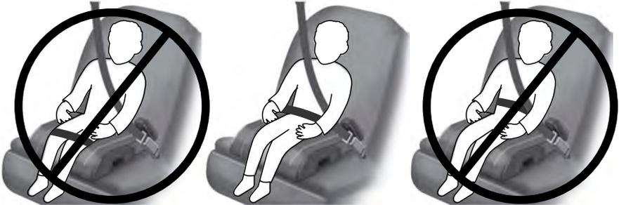
If the booster seat slides on the vehicle seat upon which it is being used, placing a rubberized mesh sold as shelf or carpet liner under the booster seat may improve this condition. Do not introduce any item thicker than this under the booster seat. Check with the booster seat manufacturer's instructions.
