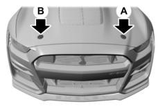
2. Press the driver side hood pin (A) first, then the passenger side hood pin (B).
