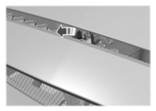
4. Release the hood latch by pushing the secondary release lever to your left-hand side and open the hood.
