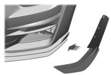
Locate the splitter wicker to the vehicle. The face of the splitter wicker with the three attaching holes should be aligned to the wheel liner bracket.
