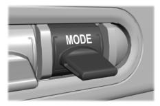
Toggle the mode switch on the center stack under the display screen to change the drive mode.
