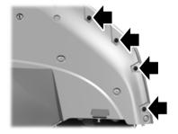
3. Remove the four M6 screws from the outboard corner of the splitter.
