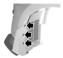
6. Loosely install 3 of the bolts removed in step 2 to the wheel liner bracket.
