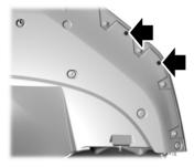
4. Install the two M4.2 push nuts into the bottom of the front splitter.
