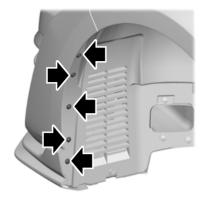
2. Remove the five bolts from the wheel liner.
