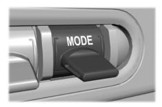
To change the drive mode setting, press the mode button on the instrument panel under the display. The first press illuminates the selected mode, subsequent presses change the selected mode. **Note:** Mode changes are not available when the ignition is off or when the transmission is in reverse (R). Some modes may be unavailable when the transmission is in drive (D) or sport (S).
