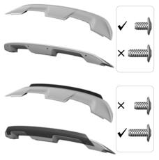
**Note:** The Gurney flap comes with longer size bolts to install it onto the rear spoiler. **Do not use the longer size bolts without the Gurney flap attached or damage to the spoiler may occur.**
