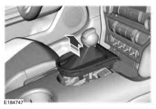
Using a flat head screwdriver or similar tool, remove the chrome bezel and gearshift bracket at the base of the gearshift lever.
