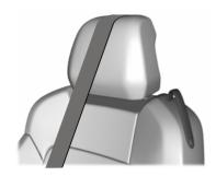
For standard front seats without rear seats, route the tether strap over the top of the seat.
