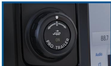
Press the center button on the knob located to the right of the steering wheel to begin setting up the system.
