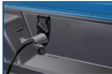
Plug in the wiring harness to the sensor and the vehicle. When you plug in the wiring harness to the 12-way connector, the red seal on the connector should not be visible when the connector is fully plugged in.
