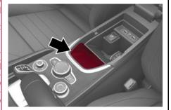
If the smartphone is removed from the charging pad, the charge will immediately be interrupted.
