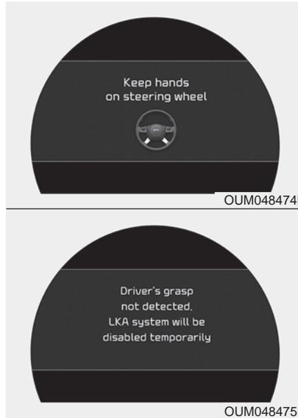
If the driver takes hands off the steering wheel for several seconds while the LKA is activated, the system will warn the driver.
