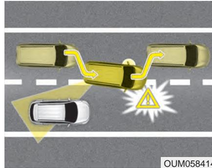
The BCA detects the front lane through the camera installed on the upper front windshield and detects the side/rear areas through radar sensors.
