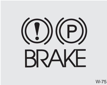
Check the brake warning light by turning the ignition switch ON (do not start the engine). This light will be illuminated when the parking brake is applied with the ignition switch in the START or ON position.
