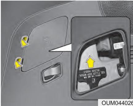
If the fuel filler door does not open using the remote fuel filler door release, you can open it manually. Remove the panel in the cargo area. Pull the handle out slightly.
