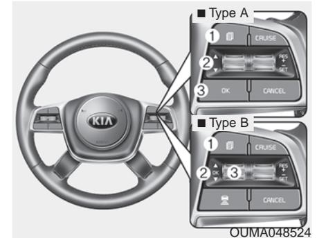
The LCD display modes can be changed by using the control buttons on the steering wheel.
