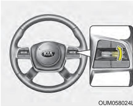
If any method other than the CRUISE button was used to cancel cruising speed and the system is still activated, the cruising speed will automatically resume when you move the lever up/down (to RES+ or SET-).
