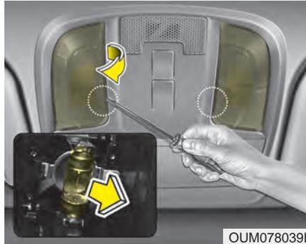
1. Using a flat-blade screwdriver, gently pry the lens cover from lamp housing.
