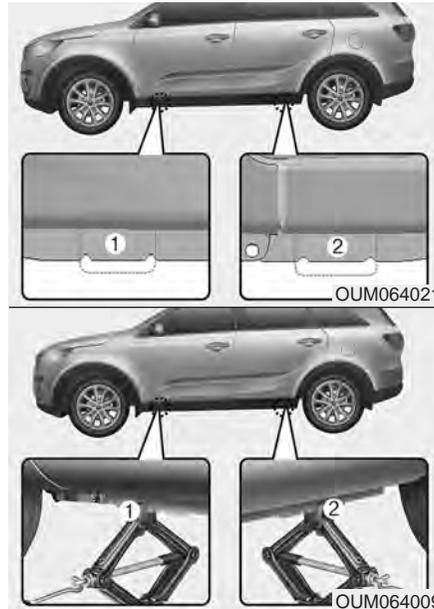
7. Place the jack at the front (1) or rear (2) jacking position closest to the tire you are changing. Place the jack at the designated locations under the frame. The jacking positions are plates welded to the frame with two tabs and a raised dot to index with the jack.
