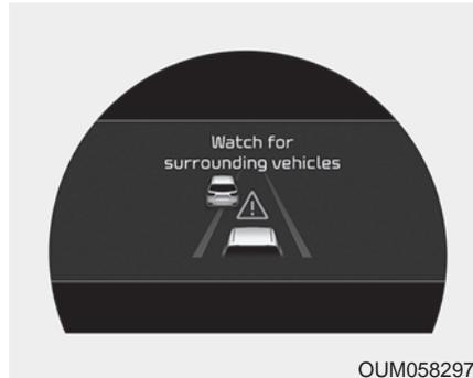
If the vehicle ahead (vehicle speed: less than 20 mph (30 km/h)) moves to the next lane, the warning chime will sound and a message will appear.
