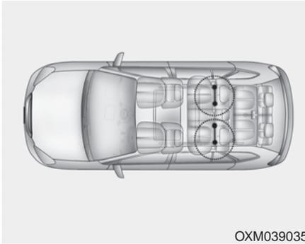
Some child seat manufacturers make child restraint seats that are labeled as LATCH or LATCH-compatible child restraint seats. LATCH stands for "Lower Anchors and Tethers for Children". These seats include two rigid or webbing mounted attachments that connect to two LATCH anchors at specific seating positions in your vehicle. This type of child restraint seat eliminates the need to use seat belts to attach the child seat in the rear seats.
