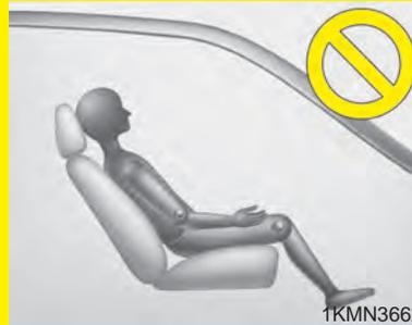
The driver must advise the passenger to keep the seatback in an upright position whenever the vehicle is in motion. If a seat is reclined during an accident, the occupant's hips may slide under the lap portion of the seat belt, applying great force to the unprotected abdomen.
