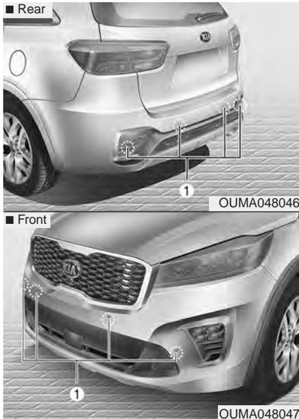
The Parking Distance Warning assists the driver during movement of the vehicle by chiming if any object is sensed within the distance of 39 in. (100 cm) in front and 47 in. (120 cm) behind the vehicle.
