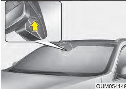
The Lane Keeping Assist System detects the lane markers on the road with a front view camera at the front windshield, and assists the driver's steering to help keep the vehicle in the lanes.
