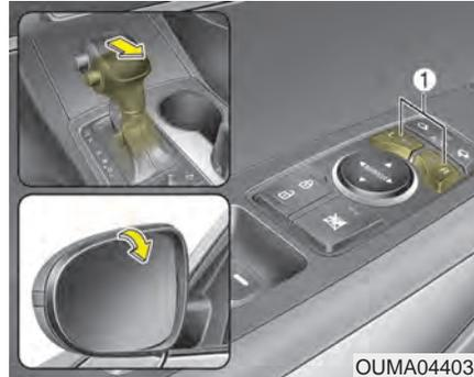
While the vehicle is moving rearward, the outside rearview mirror(s) will move downward to aid reverse parking. According to the position of the outside rearview mirror switch (1), the outside rearview mirror(s) will operate as follows:
