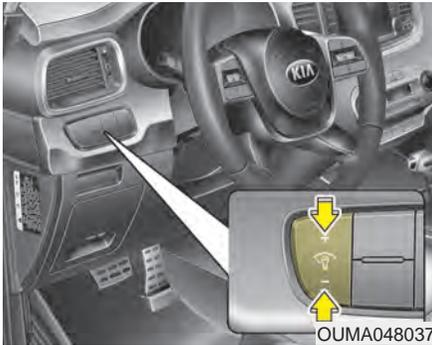
The brightness of the instrument panel illumination is changed by pressing the illumination control button (“+” or “-”) when the ignition switch or Engine Start/Stop button is ON, or the tail lights are turned on.
