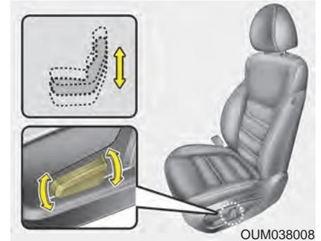
Pull the front portion of the control switch up to raise or press down to lower the front part of the seat cushion. Pull the rear portion of the control switch up to raise or press down to lower the rear part of the seat cushion. Release the switch once the seat reaches the desired position.
