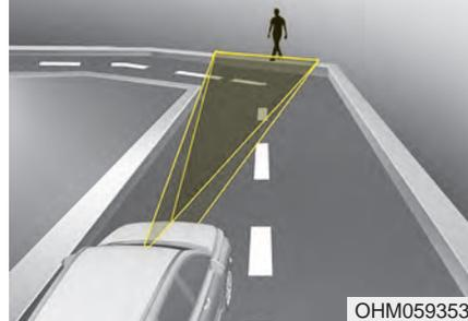
Forward Collision-Avoidance Assist system may recognize a vehicle or pedestrian in the next lane or outside the lane when driving on a curved road.
