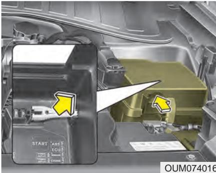
3. Pull the suspected fuse straight out. Use the removal tool provided on the engine compartment fuse panel cover.
