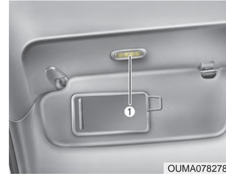
If the vanity mirror lamp (LED) (1) does not operate, have the vehicle checked by an authorized Kia dealer. The LED lamps cannot be replaced as a single unit because it is an integrated unit. The LED lamps has to be replaced with the unit. A skilled technician should check or repair the vanity mirror lamp (LED), for it may damage related parts of the vehicle.
