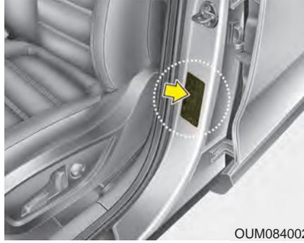
The tires supplied on your new vehicle are chosen to provide the best performance for normal driving. The tire label located on the driver's side center pillar gives the tire pressures recommended for your vehicle.
