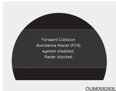
When the sensor cover or the sensor lens is smudged with the foreign substances, such as snow or rain, the FCA operation may temporarily stop. In this case, the warning message appears to warn the driver.
