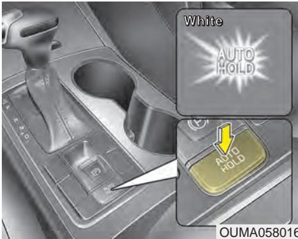
1. Depress the brake pedal, start the engine and then press the Auto Hold button. The white AUTO HOLD indicator will come on indicating the system is in standby. Before the Auto Hold will engage, the driver's door, engine hood and trunk must be closed and the driver's seat belt must be fastened.
