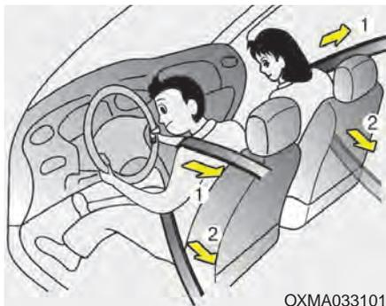
Your vehicle is equipped with driver's and front passenger's pre-tensioner seat belts (retractor pretensioner and EFD (Emergency Fastening Device)). The pre-tensioner seat belts may be activated, when a frontal collision is severe enough, together with the air bags.
