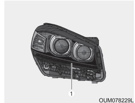
If the position lamp (LED) (1) does not operate, have the vehicle checked by an authorized Kia dealer. The LED lamps cannot be replaced as a single unit because it is an integrated unit. The LED lamps has to be replaced with the unit.
