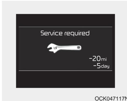
When Service Required is set, the remaining distance/period to drive appears on the LCD screen.
