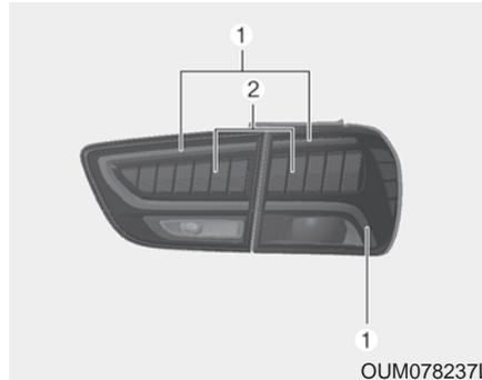
If the stop and tail lamp (LED) (1,2), does not operate, have the vehicle checked by an authorized Kia dealer. The LED lamps cannot be replaced as a single unit because it is an integrated unit. The LED lamps has to be replaced with the unit. A skilled technician should check or repair the stop and tail lamp (LED), for it may damage related parts of the vehicle.
