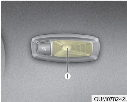
If the personal lamp (LED) (1), does not operate, have the vehicle checked by an authorized Kia dealer. The LED lamps cannot be replaced as a single unit because it is an integrated unit. The LED lamps has to be replaced with the unit.
