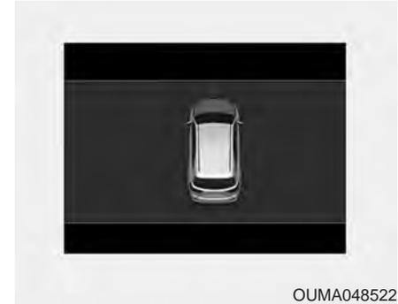
The warning message will appear on the LCD display when hood is open. The warning chime will operate when the vehicle is being driven above 3 mph (3 km/h) with the hood open.
