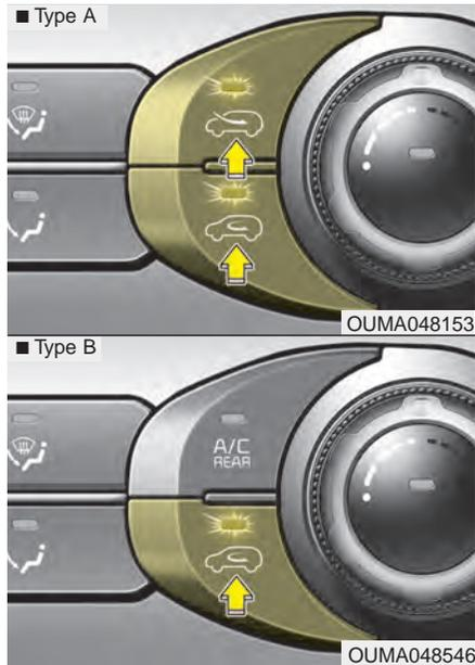
The air intake control is used to select the outside (fresh) air position or recirculated air position.
