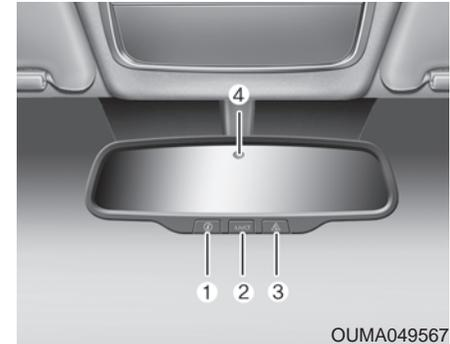
The electric rearview mirror automatically controls the glare from the headlights of the vehicles behind you in nighttime or low light driving conditions. The sensor (4) mounted in the mirror senses the light level around the vehicle, and automatically controls the headlight glare from the vehicles behind you.
