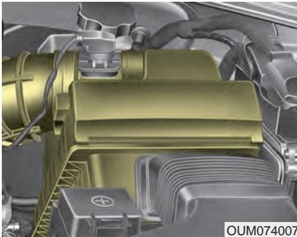
It must be replaced when necessary, and should not be washed.
