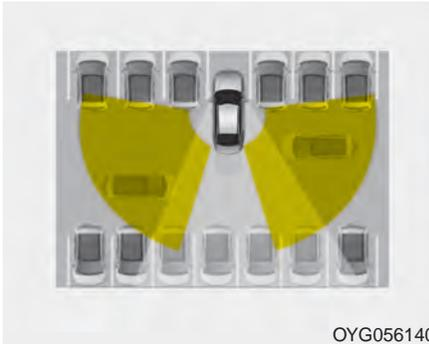
The RCCW uses radar sensors to monitor the approaching cross traffic from the left and right side of the vehicle when your vehicle is in reverse.
