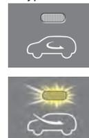
With the outside (fresh) air position selected, air enters the vehicle from outside and is heated or cooled according to the function selected.
