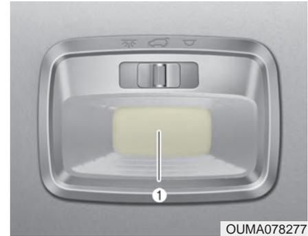
If the luggage lamp (LED) (1) does not operate, have the vehicle checked by an authorized Kia dealer. The LED lamps cannot be replaced as a single unit because it is an integrated unit. The LED lamps has to be replaced with the unit.
