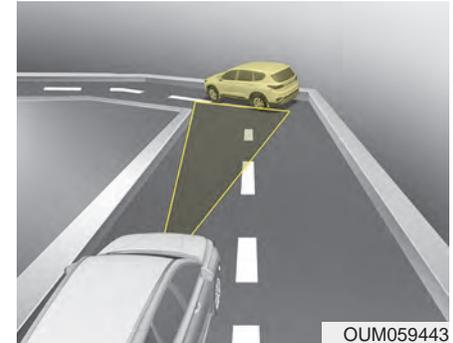
Forward Collision-Avoidance Assist system may recognize a vehicle in the next lane or outside the lane when driving on a curved road.
