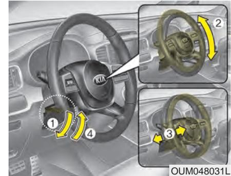
To change the steering wheel angle, pull down the lock-release lever (1), adjust the steering wheel to the desired angle (2) and height (3) then pull up the lock-release lever to lock (4) the steering wheel in place. Be sure to adjust the steering wheel to the desired position before driving.
