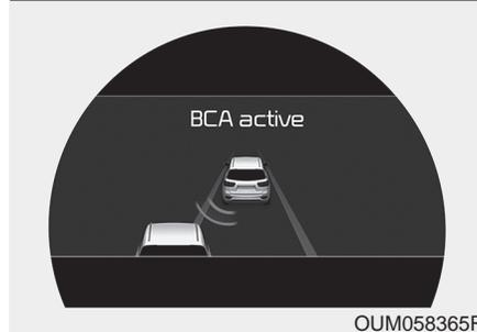
The Blind-Spot Collision-Avoidance Assist (BCA) system may apply braking power, when an approaching vehicle is detected within a certain distance next to/behind your vehicle.
