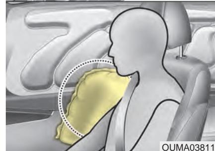
Your vehicle is equipped with a side air bag in each front seat. The purpose of the air bag is to provide the vehicle's driver and/or the front passenger with additional protection than that offered by the seat belt alone.
