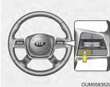
This function allows you to program the vehicle to maintain relative distance to the vehicle ahead without depressing the accelerator pedal or brake pedal.
