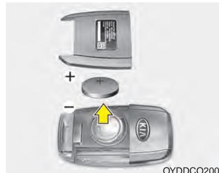
The transmitter uses a 3 volt lithium battery which will normally last for several years. When replacement is necessary, use the following procedure.
