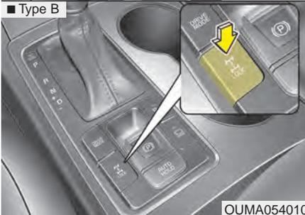
Engine power can be delivered to all front and rear wheels for maximum traction. AWD is useful when extra traction is required, such as, when driving on slippery, muddy, wet, or snow-covered roads.
