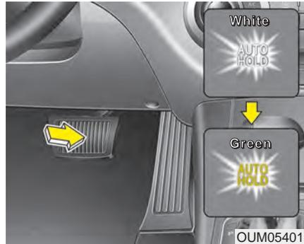
2. When coming to a complete stop by depressing the brake pedal, the AUTO HOLD indicator changes from white to green indicating the AUTO HOLD is engaged and EPB is applied. The vehicle will remain at a standstill even if you release the brake pedal.
