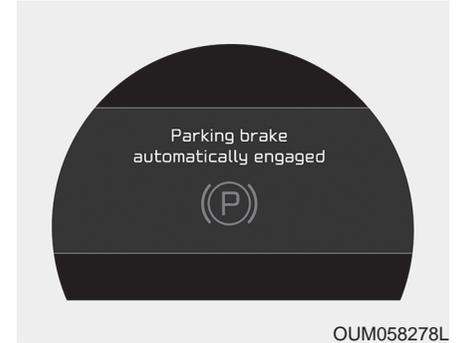
If the EPB is applied while Auto Hold is activated because of ESC (Electronic Stability Control) signal, a warning will sound and a message will appear.
