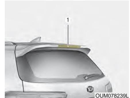
If the high mounted stop lamp (LED) (1) does not operate, have the vehicle checked by an authorized Kia dealer. The LED lamps cannot be replaced as a single unit because it is an integrated unit. The LED lamps has to be replaced with the unit. A skilled technician should check or repair the high mounted stop lamp (LED), for it may damage related parts of the vehicle.
