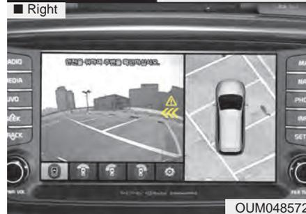
If the vehicle detected by the sensors approaches from the rear left/right side of your vehicle, the warning chime will sound, the warning light on the outside rearview mirror will blink and a message will appear on the LCD display. If the rear view monitor system is in activation, a message will also appear on the 'Car Infotainment System'.
