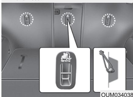
Child restraint hook holders are located on the back of the rear seat-backs.
