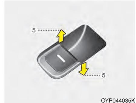
The driver's door has a master power window switch that controls all the windows in the vehicle.
