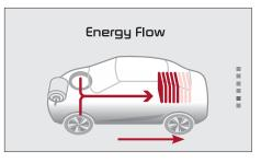
**Engine Generation/Regeneration** - The engine and the regenerative braking system are both recharging the Hybrid/Plug-In battery.
