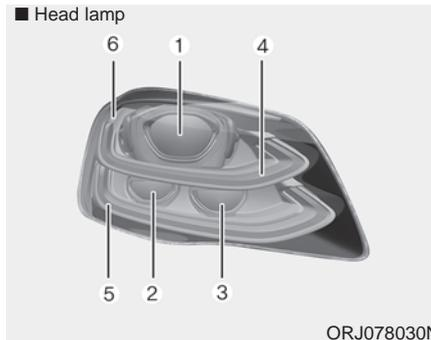
If the Low/High beam lamp, day time running lamp, position lamp, front turn signal lamp and side marker (1,2,3,4,5,6) do not operate, have the vehicle checked by an authorized K900 Kia dealer.
