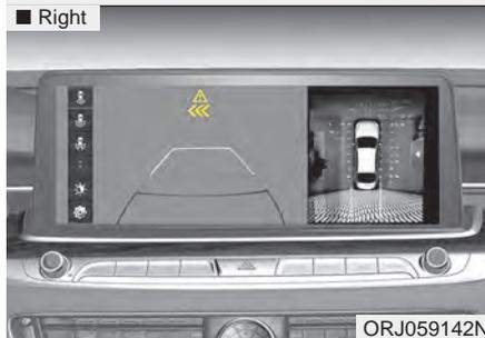
If the risk of collision is detected while RCCW system is generated, brake is controlled. The instrument cluster will inform the driver of the brake control. If the rear view monitor system is in activation, a message will also appear on the audio or AVN screen.
