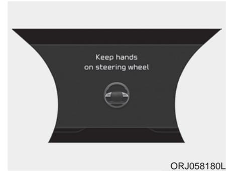
The hands-off warning appears when the system detects that the driver's hands are not on the steering wheel while HDA system is in work.
