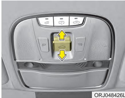
The sunshade will automatically open with the glass panel when the glass panel moves. Close it manually if you want it closed.
