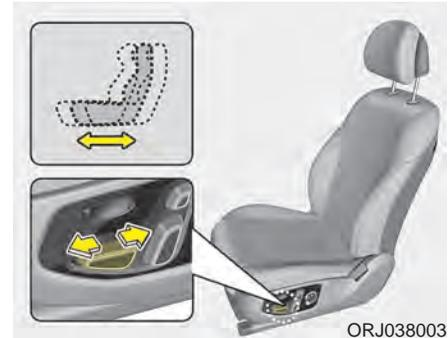
Push the control switch forward or backward to move the seat to the desired position.
