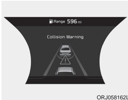
This warning message appears on the LCD display with a warning chime. Additionally, the engine management system intervenes to help decelerate the vehicle.
