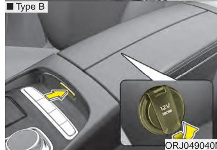
The power outlet is designed to provide power for mobile telephones or other devices designed to operate with vehicle electrical systems. The devices should draw less than 20 amps with the engine running.
