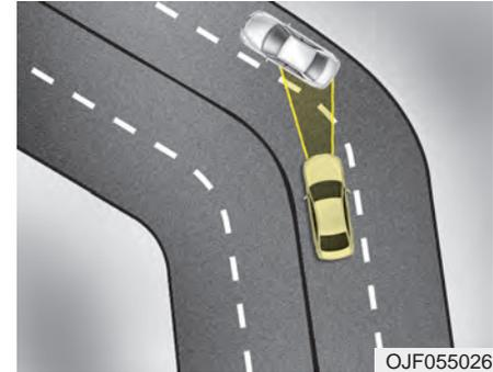
FCA system may recognize a vehicle in the next lane when driving on a curved road.
