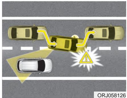
Blind-Spot Collision-Avoidance Assist (BCA) system detects the front lane through the camera installed on the upper front windshield and detects the side/rear areas through radar sensors.
