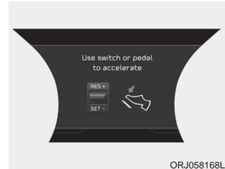
While the Smart Cruise Control (SCC) system is in operation, your vehicle stops behind the vehicle in front when it stops. The message is displayed on the cluster within 3 seconds after the stop and the system will be in the standby position.
