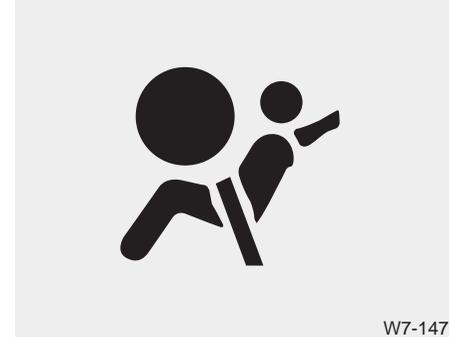
The purpose of the air bag warning light in your instrument panel is to alert you of a potential problem with your air bag system, which could include your side and/or curtain air bags used for rollover protection.
