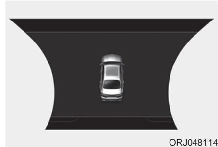
If the driver turns off the engine when the sunroof is not fully closed, the warning chime will sound for a few seconds and the above warning illustration will appear on the LCD display. Close the sunroof securely when leaving your vehicle.
