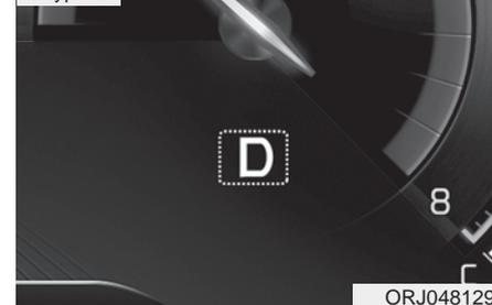
This indicator displays which automatic transmission shift lever mode is selected.
