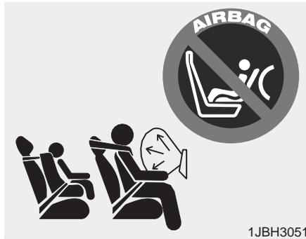
Never place a rear-facing child restraint in the front passenger's seat. If the air bag deploys, it would impact the rear-facing child restraint and could cause serious or fatal injuries to the child.
