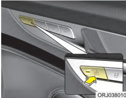
If you open the door with the DOOR switch on, the seat will be moved backwards. (However, this function does not work if the seat is already at its farthest rear position.) When the door is closed, the seat will move forward. The switch can be turned on and off.
