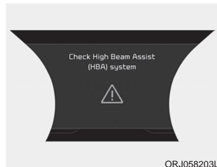
When the High Beam Assist is not working properly, a warning message will come on for a few seconds. After the message disappears, the master warning light (
