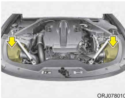
The air filter must be replaced when necessary according to the Maintenance Schedule, and should not be washed.
