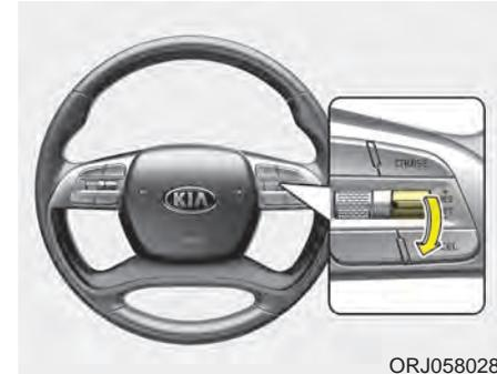
3. Push the toggle switch down (SET-). The Set Speed and Vehicle-to-Vehicle Distance on the LCD display will illuminate.
