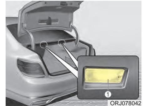
If the trunk lamp (1) does not operate, have the vehicle checked by an authorized K900 Kia dealer.
