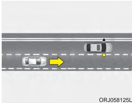
BCW system feature will alert you when a vehicle is approaching in an adjacent lane at a high rate of speed. If the driver activates the turn signal when the system detects an oncoming vehicle, the system sounds an audible alert.
