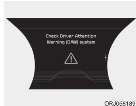
When the "Check System" warning message appears, the system is not working properly. If this occurs, have the system checked by an authorized K900 Kia dealer.
