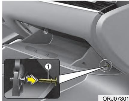
1. With the glove box open, remove the pin(1) from the support strap.
