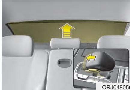
To fold the rear curtain, press the button. To unfold the rear curtain, press the button again.
