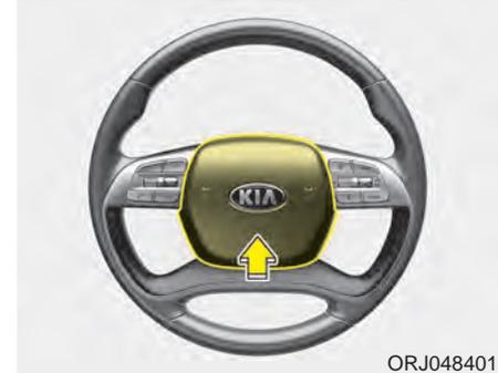
To sound the horn, press the horn symbols on your steering wheel. Check the horn regularly to be sure it operates properly.
