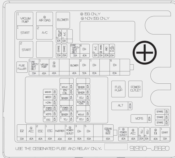
**Engine room compartment fuse panel**
