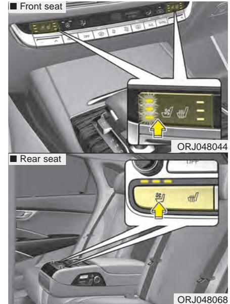
The temperature setting of the seat changes according to the switch position.
