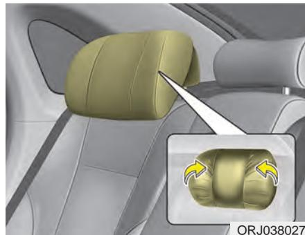
When you hold both sides of the headrest and try to bend it (pull it forward), you can adjust it as you want. It is a convenience device for supporting the head of the passenger.
