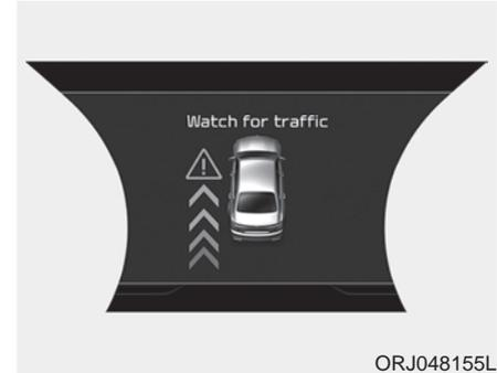
If a vehicle occupant opens a door and the system senses a car approaching from behind the opened door, the warning message “Watch for traffic” appears and the alarming sound will continue for five seconds.
