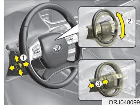
Adjust the steering wheel angle (2) and position (3) with the switch (1).
