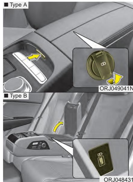
The USB charger is designed to recharge devices using a USB cable. The electrical devices can be recharged when the Engine Start/Stop button is in ACC/ON/START position.
