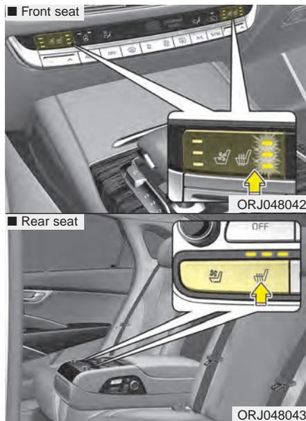
The seat warmer is provided to warm the front seats during cold weather. With the ignition switch in the ON position, press either of the switches to warm the driver's seat or the front passenger's seat.
