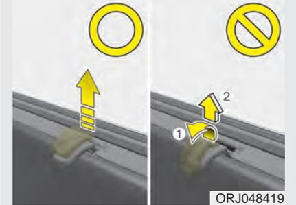
***To open up the flap on the door, lift the knob straight up. If the knob is pulled outward and lifted up, the flap will not open up. To close it, lower the knob down slowly.***
