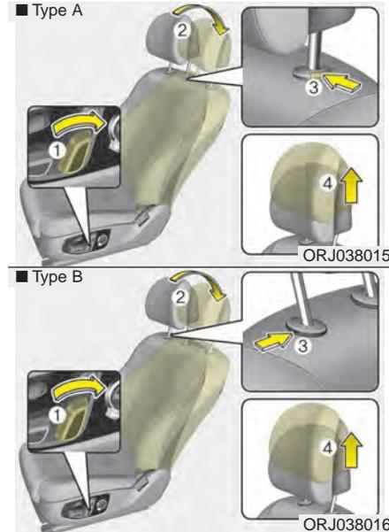
2. Type A (manual): Raise the headrest as far as it can go. Then Press the headrest release button (3) while pulling the headrest up (4). Type B (power, if equipped) : Raise the headrest to the end with the headrest height adjustment switch, then insert a pointed tool into the headrest adjustment hole (3). After inserting the tool, remove the headrest by pulling it all the way up (4).
