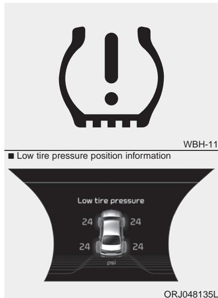
When the tire pressure monitoring system warning indicators are illuminated, one or more of your tires is significantly under-inflated.
