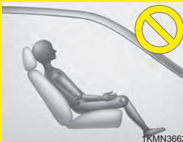
The driver must advise the passengers to keep the seatback in an upright position whenever the vehicle is in motion. If a seat is reclined during an accident, the restraint system's ability to restrain will be greatly impaired.
