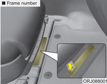
The vehicle identification number (VIN) is the number used in registering your vehicle and in all legal matters pertaining to its ownership, etc. The number is punched under driver or front passenger seat.
