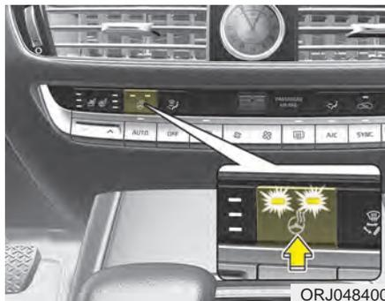
When the Engine Start/Stop Button is in the ON position, pressing the heated steering wheel button warms the steering wheel. The indicator on the button will illuminate.
