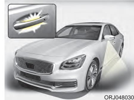
When all the doors (and trunk) are locked and closed, the pocket lamp and puddle lamp will come on for about 15 seconds if any of the below is performed.
