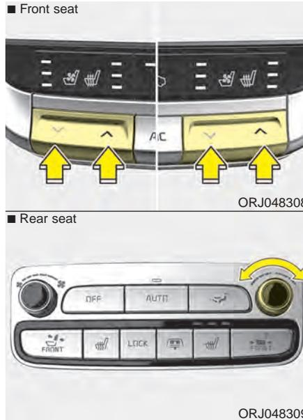
2. Press the temperature buttons or turn the temperature control knob to the desired temperature.
