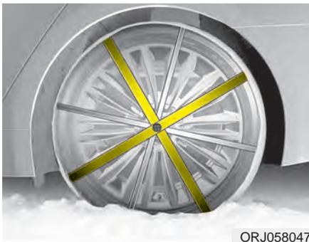
Since the sidewalls on some radial tires are thinner than other types of tires, they may be damaged by mounting certain types of tire chains on them. Therefore, the use of snow tires is recommended instead of tire chains. Do not mount tire chains on vehicles equipped with aluminum wheels; if unavoidable, use an AutoSock (fabric snow chain). Install the tire chain after reviewing the instructions provided with the tire chains.
