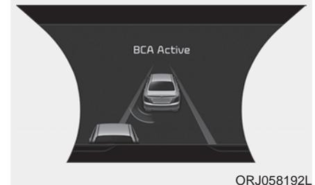
Blind-Spot Collision-Avoidance Assist (BCA) system may apply braking power when an approaching vehicle is detected within a certain distance next to/behind your vehicle.
