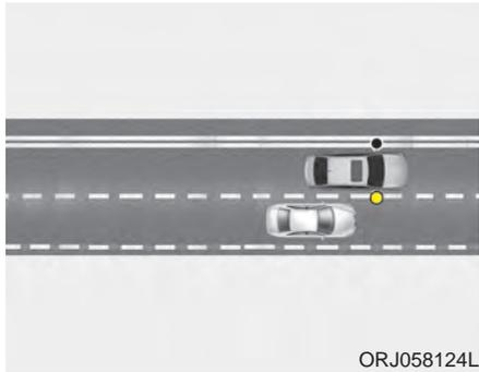
Blind-Spot Collision Warning (BCW) system uses radar sensors in the rear bumper to monitor and warn the driver of an approaching vehicle in the driver's blind spot area.
