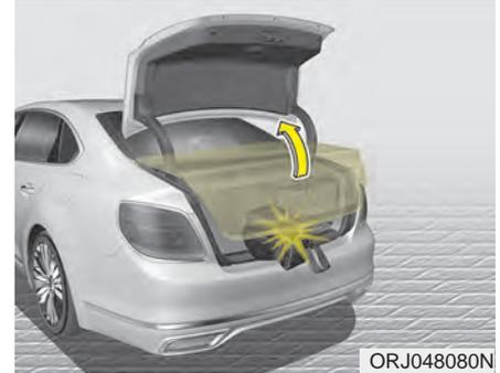
During power opening and closing if the power trunk is blocked by an object or part of the body, the power trunk will detect the resistance.
