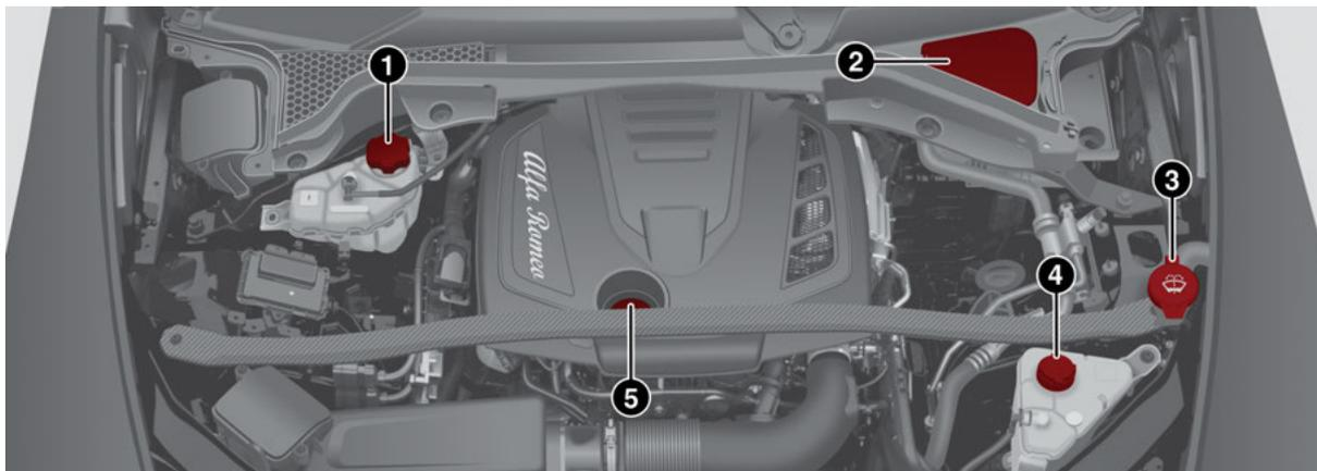
1 - Engine Coolant Reservoir Cap
