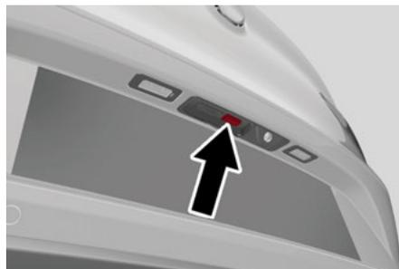
**External Liftgate Release Switch (Vehicles With Passive Entry)**
