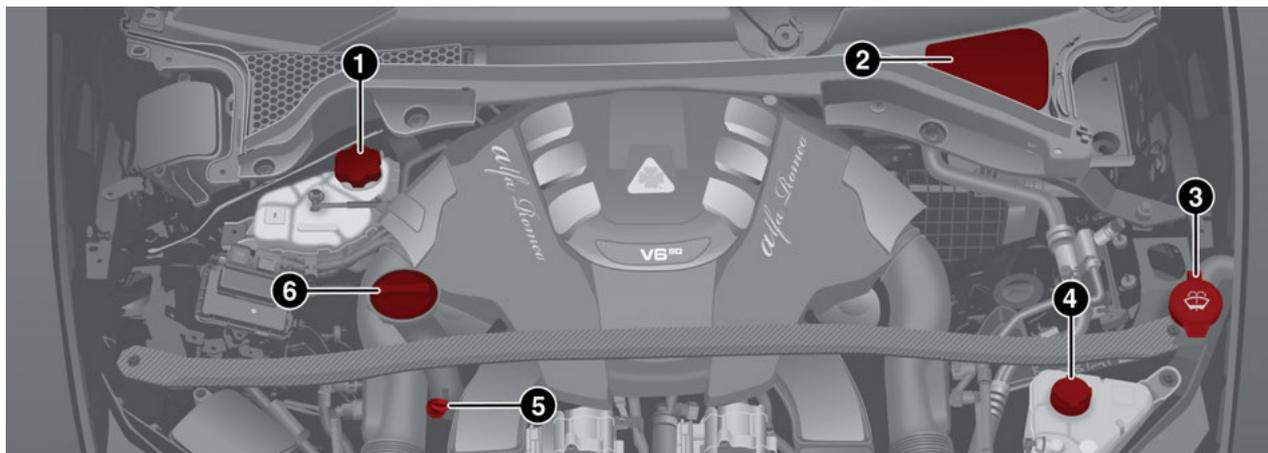
1 - Engine Coolant Reservoir Cap
