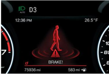
The audible and visual signals warn the driver before the system activates, depending on the vehicle speed.
