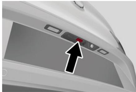
**External Liftgate Release Button (Vehicles With Passive Entry)**
