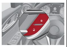
Door Lock And Unlock Switch Panel
