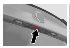
Exterior Trunk Lid Release Switch (Vehicles With Passive Entry)
