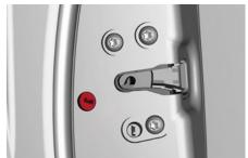
Door Lock Manual Release Lock Cylinder
