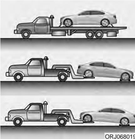
If emergency towing is necessary, we recommend having it done by an authorized K900 Kia dealer or a commercial tow-truck service. Proper lifting and towing procedures are necessary to prevent damage to the vehicle. The use of wheel dollies or flatbed is recommended.
