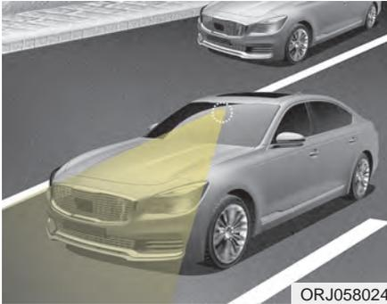
With the front camera mounted on the top of the windshield, the Lane Following Assist system is designed to ensure the vehicle stays in its lane by monitoring the lane ahead of the car and controlling over the direction of the steering wheel.
