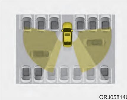
The Rear Cross-Traffic Collision Warning (RCCW) System uses radar sensors to monitor the approaching cross traffic from the left and right side of the vehicle when your vehicle is in reverse.
