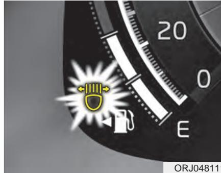
If the DBL malfunction indicator comes on, the DBL is not working properly. Drive to the nearest safe location and restart the engine. If the indicator continuously remains on, have your vehicle checked by an authorized K900 Kia dealer as soon as possible.
