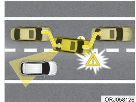
The Blind-Spot Collision-Avoidance Assist System (BCA) detects the front lane through the camera installed on the upper front windshield and detects the side/rear areas through radar sensors.
