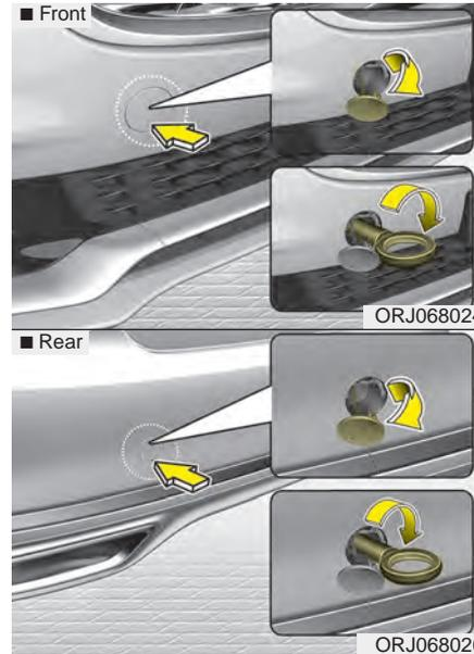
1. Open the trunk, and remove the towing hook from the tool case.
