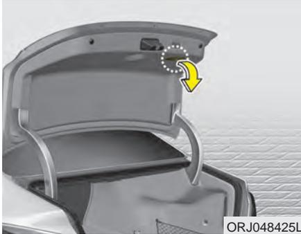
To close, lower the trunk lid, then press down on it until it locks. To be sure the trunk lid is securely fastened, always check by trying to pull it up again.
