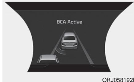
The Blind-Spot Collision-Avoidance Assist System (BCA) may apply braking power, when an approaching vehicle is detected within a certain distance next to/behind your vehicle.
