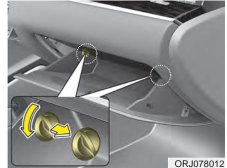
2. Open the glove box and remove the stoppers on both sides.
