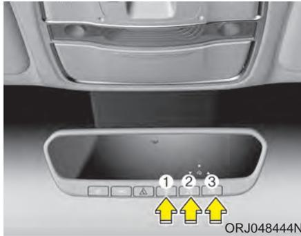
3. Press and release the programmed HomeLink button to activate the garage door.
