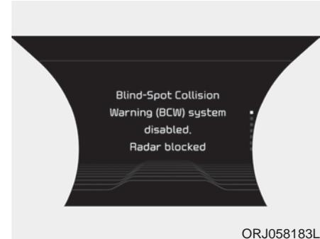
**Blind-Spot Collision Warning (BCW) system disabled.****Radar blocked**
