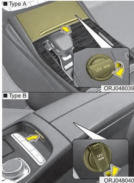
The power outlet is designed to provide power for mobile telephones or other devices designed to operate with vehicle electrical systems. The devices should draw less than 20 amps with the engine running.
