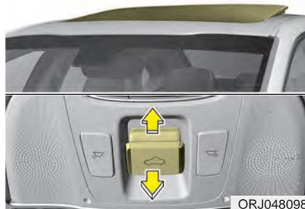
To tilt open the sunroof, push the sunroof control lever upward. To stop the sunroof tilting at any point, operate the control lever.
