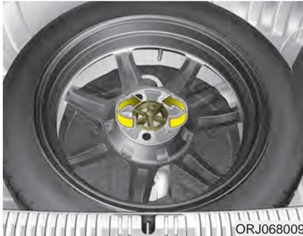
Turn the tire hold-down wing bolt counterclockwise.
