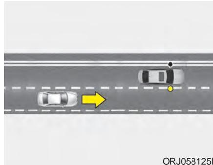
The Lane Change Assist feature will alert you when a vehicle is approaching in an adjacent lane at a high rate of speed. If the driver activates the turn signal when the system detects an oncoming vehicle, the system sounds an audible alert.
