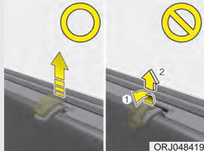
*To open up the flap on the door, lift the knob straight up. If knob is pulled outward and lift it up, the flap will not open up. To close it, lift the knob down slowly.*
