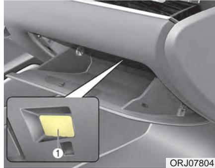
If the glove box lamp (1) does not operate, have the vehicle checked by an authorized K900 Kia dealer.
