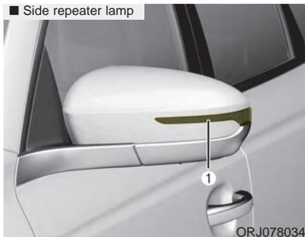
If the side repeater lamp (1) does not operate, have the vehicle checked by an authorized K900 Kia dealer.
