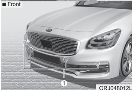
The parking distance warning assists the driver during movement of the vehicle by chiming if any object is sensed within the distance of 39 in. (100 cm) in front and 47 in. (120 cm) behind the vehicle.
