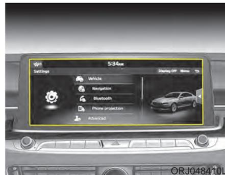
On this mode, you can change setting of the doors, lamps, and so on. You can change the modes on the Navigation touch screen in instrument panel.
