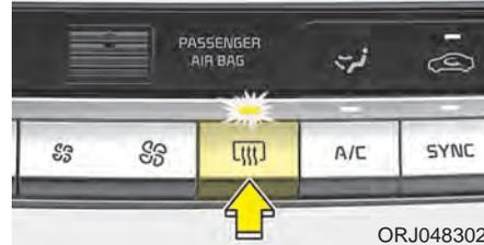
The defroster heats the window to remove frost, fog and thin ice from the rear window, while the engine is running.
