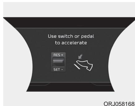
While the Smart Cruise Control (SCC) system is in operation, your vehicle stops behind the vehicle in front when it stops. The message is displayed on the cluster within 3 seconds after the stop and the system will be in the standby position.
