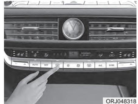
During night driving, if hands are near to touch the climate control system, button lighting will increase for better recognition. Switch lighting function can be selected or deselected on the audio display. Hands in gloves are not recognized for this function.
