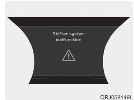
The warning message appears on the LCD display, when the transmission or the shift lever does not properly operate in the P (Park) position. In this case, have the vehicle inspected by an authorized K900 Kia dealer immediately.
