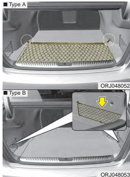
To keep items from shifting in the cargo area, you can use the holders located in the cargo area to attach the luggage net.
