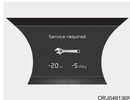
When Service Required is set, the remaining distance/time before service is required appears on the LCD screen.
