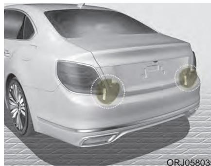
The rear radars are the sensors inside the rear bumper for detecting the side/rear areas. Always keep the rear bumper clean for proper operation of the system.
