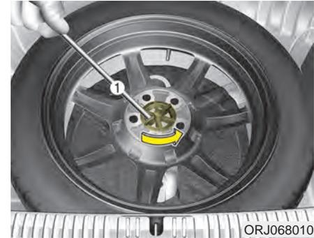
6. Insert the tool (1) into the hole and pull out the wheel cover.
