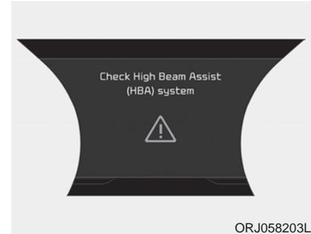
When the High Beam Assist is not working properly, a warning message will come on for a few second. After the message disappears, the master warning light (
