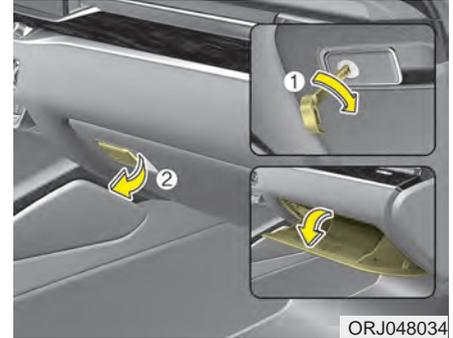
The glove box can be locked and unlocked with a master key (1). (if equipped)
