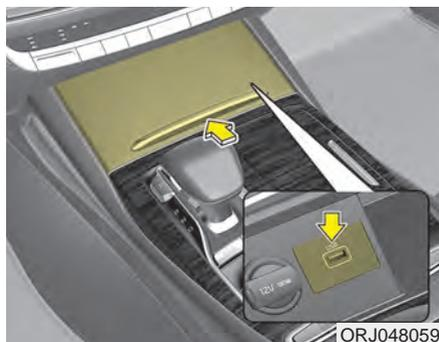
You can use a USB port to plug in a USB or iPod®.
