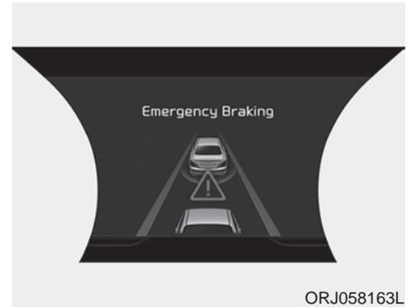
This warning message appears on the LCD display with a warning chime.
