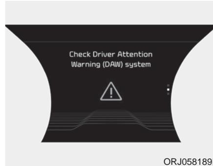
When the "Check System" warning message appears, the system is not working properly. In this case, have the system checked by an authorized K900 Kia dealer.
