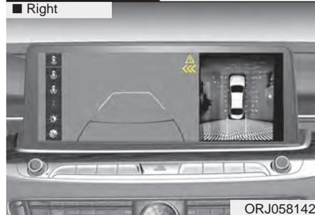
If the vehicle detected by the sensors approaches from the rear left/right side of your vehicle, the warning chime will sound, the warning light on the outside rearview mirror will blink and a message will appear on the LCD display. If the rear view monitor system is in activation, a message will also appear on the AVN screen.
