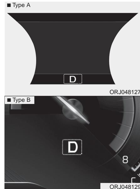
This indicator displays which automatic transmission shift lever is selected.
