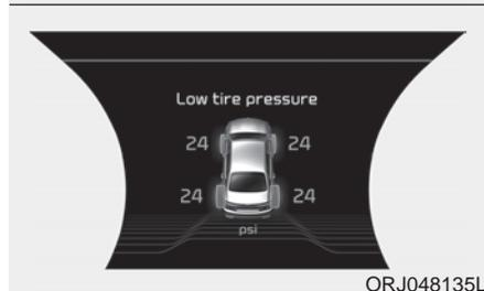
This mode displays the state of the lane safety systems (Lane Keeping Assist, Lane Following Assist), Smart Cruise Control, Lane Control, Driver Attention Warning and Tire pressure.
