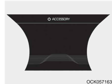
Press the engine start/stop button while it is in the OFF position without depressing the brake pedal.
