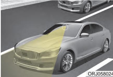
When the system detects the vehicle straying from its lane, it alerts the driver with a visual and audible warning, while applying a counter-steering torque, trying to prevent the vehicle from moving out of its lane.
