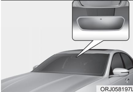
The Lane Keeping Assist (LKA) system is designed to detect the lane markers on the road with a front view camera at the front windshield, and assists the driver's steering to help keep the vehicle in the lanes.
