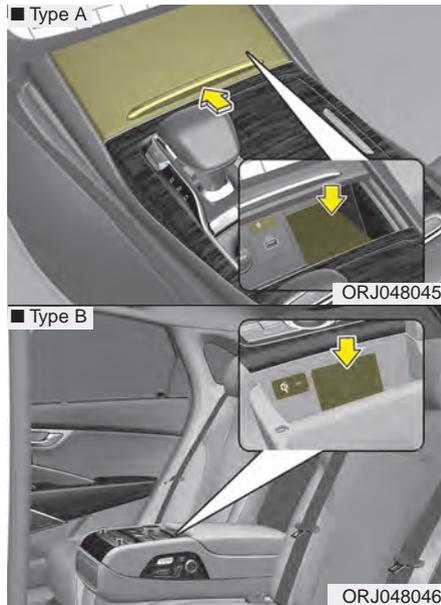
A wireless smart phone charging system is located in front of the center console.
