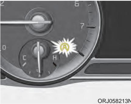
The system may not operate when an ISG related sensor or system error occurs.
