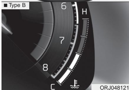
This gauge indicates the temperature of the engine coolant when the Engine Start/Stop button is ON.
