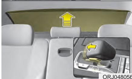
To fold the rear curtain, press the button. To unfold the rear curtain, press the button again.
