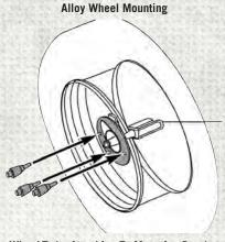
Wheel/Bolts Attaching To Mounting Bracket
