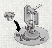
4. Position the tire vertically and lay the mounted adapter on the inner part of the rim. Using the supplied bolts, fasten the wheel to the adapter using the bolt install wrench. Tighten the bolts with the wrench extension and wrench handle.
