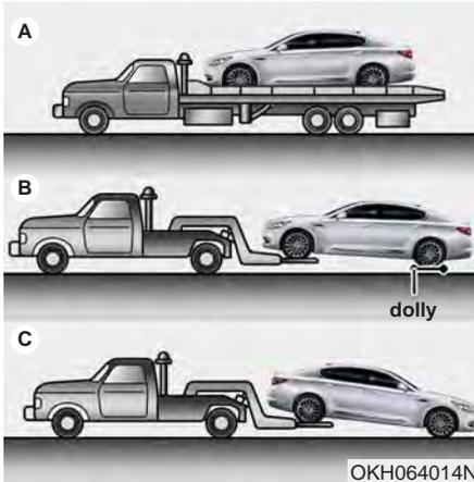
If emergency towing is necessary, we recommend having it done by an authorized K900 Kia dealer or a commercial tow-truck service. Proper lifting and towing procedures are necessary to prevent damage to the vehicle. The use of wheel dollies or flatbed is recommended.
