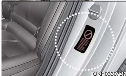
Air bag warning labels, some required by the U.S. National Highway Traffic Safety Administration (NHTSA), are attached to alert the driver and passengers of potential risks of the air bag system.
