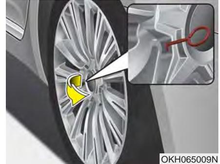
6. Insert the tool (1) into the hole and pull out the wheel cap.
