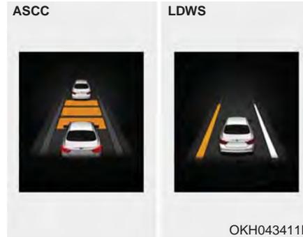
This mode displays the state of the Advanced Smart Cruise Control (ASCC) or Lane Departure Warning System (LDWS).
