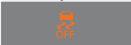
When the Engine Start/Stop button is pressed ON, the indicator light illuminates, then goes off if the ESC system is operating normally.
