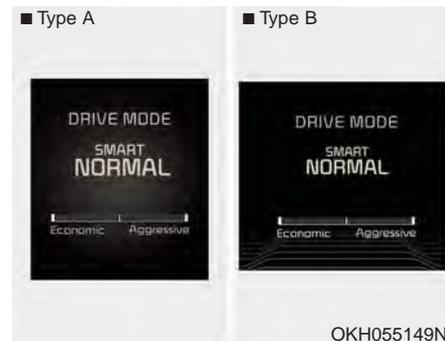
By selecting the drive mode screen, the driver can personalize the drive mode based on vehicle control preference and driving style.
