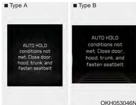
When you press the [AUTO HOLD] switch, if the driver door, engine hood and trunk are not closed or the driver seat belt is not fastened, the notice will illuminate on the LCD display. Also warning chime sounds once. In that time, press the [AUTO HOLD] button after closing the driver door, engine hood and trunk and fastening the seat belt.
