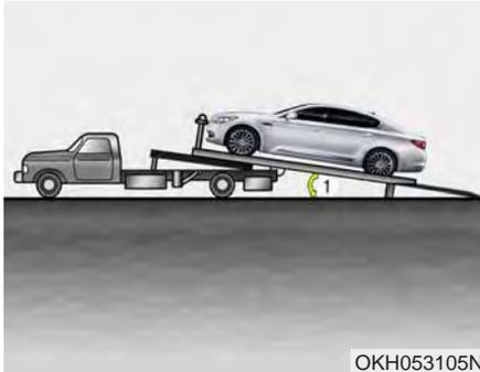
When you load the vehicle onto the tow truck, the loading angle(1) should be smaller than 6°.
