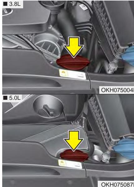
If the coolant level is low, add enough distilled (deionized) water. Bring the level to F, but do not overfill. If frequent additions are required, see an authorized K900 Kia dealer for a cooling system inspection.
