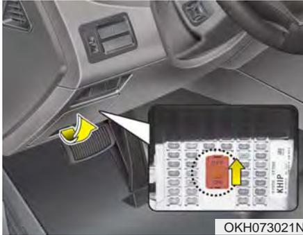
Always put the transportation fuse switch at the ON position.
