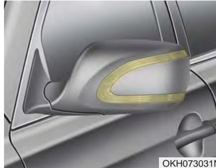
If the light bulb does not operate, have the vehicle checked by an authorized K900 Kia dealer. A skilled technician should check or repair the side repeater light, for it may damage related electrical parts and housing of outside mirror.
