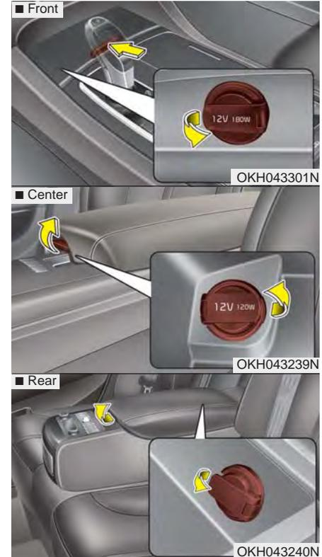
The power outlets provide power for mobile telephones or other devices designed to operate with the vehicle's electrical systems. These devices should draw less than 10 amps while the engine is running.
