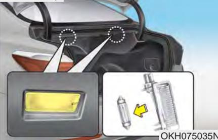
1. Using a flat-blade screwdriver, gently pry the lens from the interior light housing.
