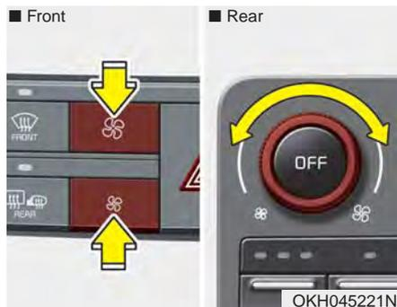
The fan speed can be set to the desired speed by pressing the fan speed control button (for front) or turning the fan speed control knob (for rear).
