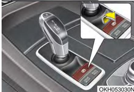
To apply the EPB (electric parking brake):
