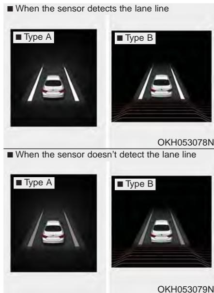
If the system detects that your vehicle is leaving the lane when the LDWS is operating and vehicle speed exceeds 38 mph (60 km/h), the warning operates as follows:
