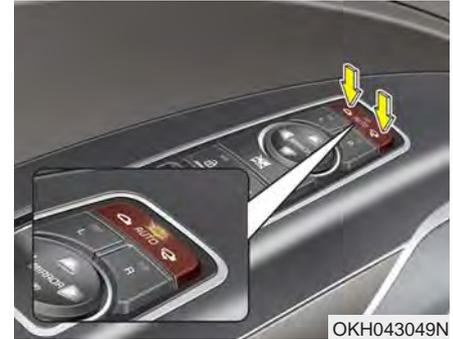
The outside rearview mirror can be folded or unfolded by pressing the switch as below.
