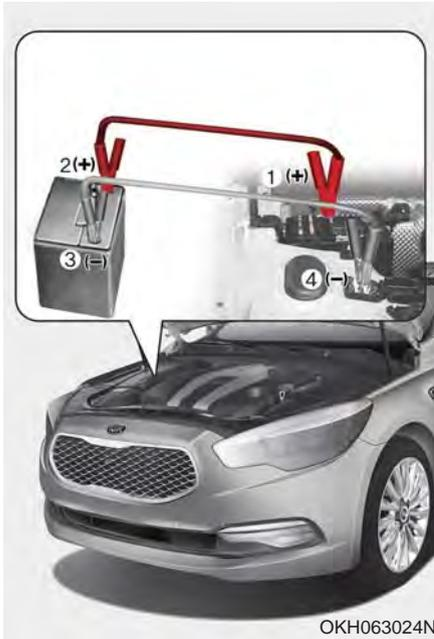
Connect cables in numerical order and disconnect in reverse order.
