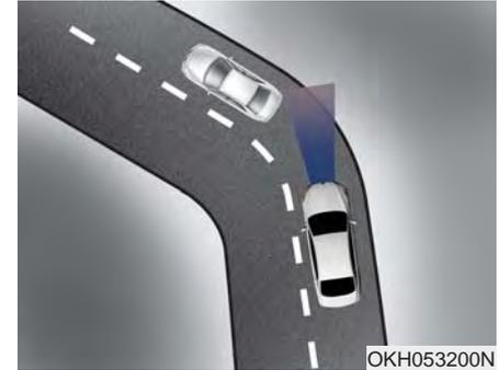
The ASCC may have limits to its ability to detect distance to the vehicle ahead due to road and traffic conditions.
