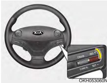
If any method other than the CRUISE lever was used to cancel cruising speed and the system is still activated, the cruising speed will automatically resume when you move the lever up/down (to RES+ or SET-).
