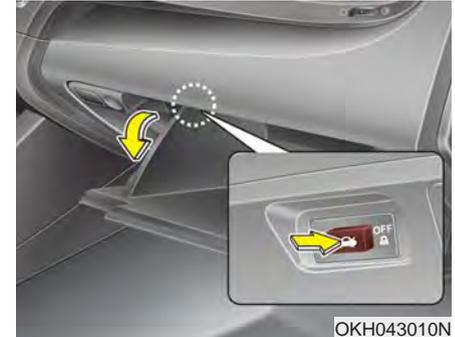
When leaving keys with parking lot and valet attendants, the following procedures will ensure your vehicle's trunk and glove box compartment can only be opened with the mechanical key.
