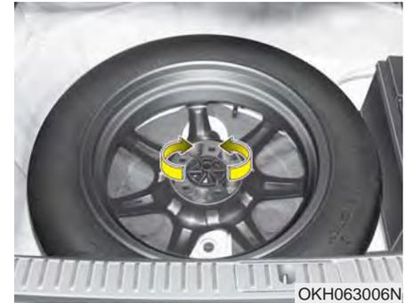
Turn the tire hold-down wing bolt counterclockwise.
