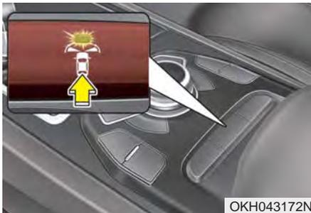
Front blind spot monitoring system is a supplemental system that shows blind spot in front of the vehicle through the AV monitor.
