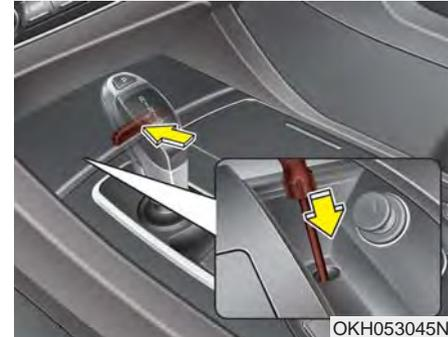
You can shift into [N] by using the driver if the jump starting is impossible to do.
