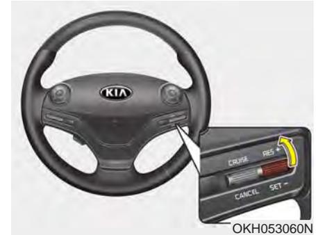
If any method other than the CRUISE lever was used to cancel cruising speed and the system is still activated, the most recent set speed will automatically resume when you move the lever up (to RES+).
