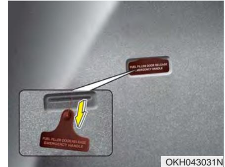
If the fuel filler lid does not open using the remote fuel filler lid release, you can open it manually by pulling the handle outward slightly.
