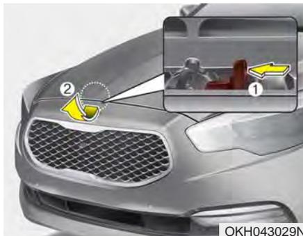
2. Go to the front of the vehicle, raise the hood slightly, push the secondary latch (1) left of the hood center and lift the hood (2).
