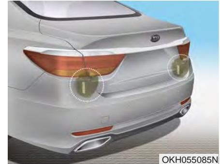
The sensors are located inside of the rear bumper.
