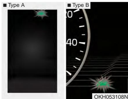
To operate the LDWS, press the button with the engine start/stop button in the ON position. The indicator (green) illuminates on the cluster. To cancel the LDWS, press the button again.
