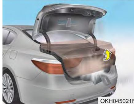
If, during power opening or closing, the trunk is blocked by an object or part of someone's body, the power trunk will detect the resistance and it will stop movement or move to the full open position to allow the object to be cleared.
