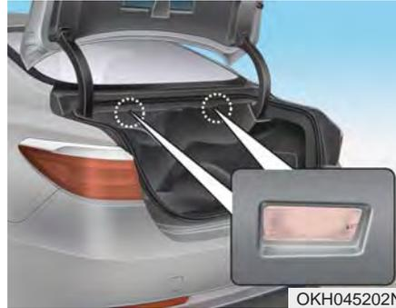
The trunk room lamp comes on when the trunk is opened. To prevent unnecessary charging system drain, close the trunk lid securely after using the trunk room.
