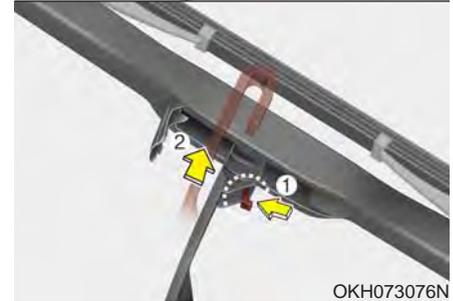
2.Turn the wiper blade clip. Then lift up the blade clip.
