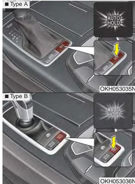
1. Depress the brake pedal and then press the Auto Hold button. The white AUTO HOLD indicator will come on and the system will be in the standby position.
