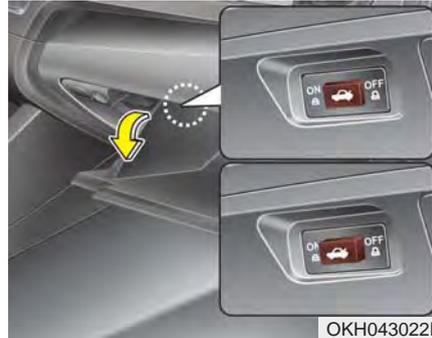
When the trunk lid control button is ON (depressed), the power trunk can be controlled with the power trunk main control button, power trunk open, close button, and the smart key.
