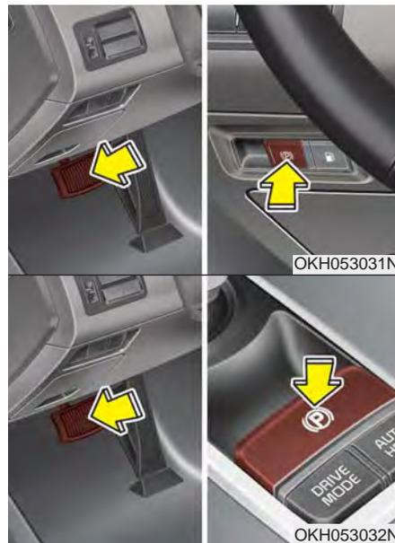
To release the EPB (electric parking brake), press the EPB switch in the following condition:
