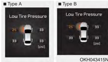
When the tire pressure monitoring system warning indicators are illuminated and warning message displayed on the cluster LCD display, one or more of your tires is significantly under-inflated. The low tire pressure position telltale light will indicate which tire is significantly under-inflated by illuminating the corresponding position light.
