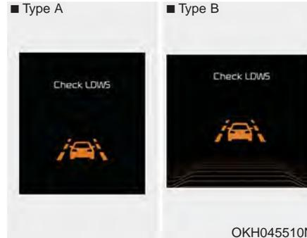
When the LDWS is not working properly, the warning light will illuminate and the warning message will come on for a few second.
