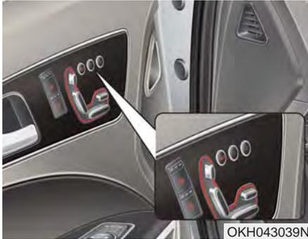
A driver position memory system is provided to store and recall the driver seat, outside rearview mirror, HUD\* (Head-Up Display), brightness of the instrument cluster illumination and steering wheel positions with a simple button operation.
