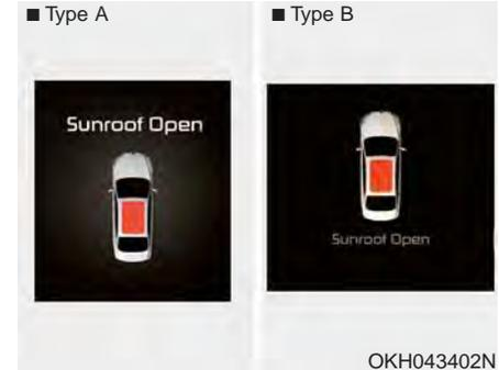
If the driver turns off the engine when the sunroof is not fully closed, the warning chime will sound for a few seconds and a warning message will appear on the LCD display.
