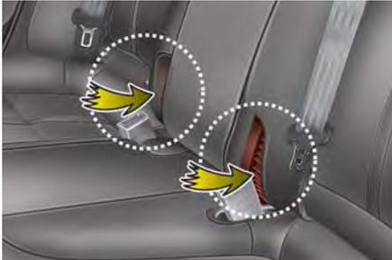
There is an air intake for the rear air ventilation at the lower part of the rear center seatback. If the air intake is blocked, efficiency of the rear air ventilation will be lower. Be careful not to block the air intake.
