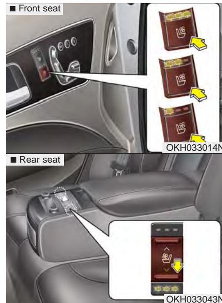
The air ventilation is provided to cool the seats during hot weather by blowing air through small vent holes on the surface of the seats and seat-backs. While the engine is running, press the switch to cool the seat.
