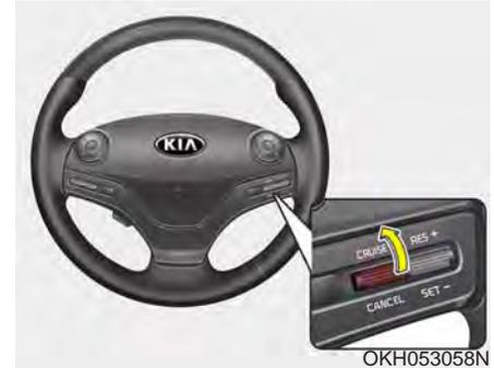
Move the lever up (to CRUISE). (the CRUISE indicator light in the instrument cluster will go off).
