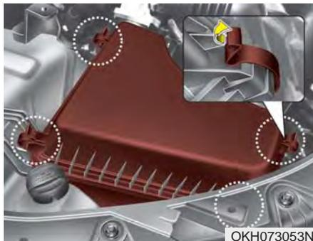
7. Loosen the air cleaner cover attaching clips and open the cover.
