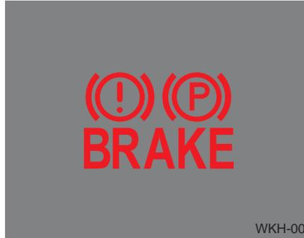
Check the brake warning light by placing the Engine Start/Stop button to the ON position. (do not start the engine). This light will be illuminated when the parking brake is applied with the Engine Start/Stop button in the START or ON position.
