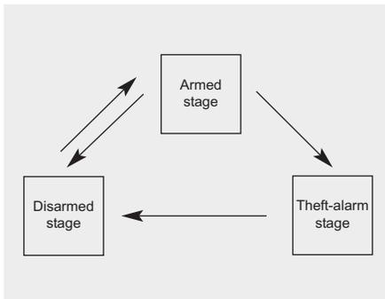
This system is designed to provide protection from unauthorized entry into the vehicle. This system is operated in three stages: the first is the "Armed" stage, the second is the "Theft-alarm" stage, and the third is the "Disarmed" stage. If triggered, the system provides an audible alarm with blinking of the hazard warning lights.
