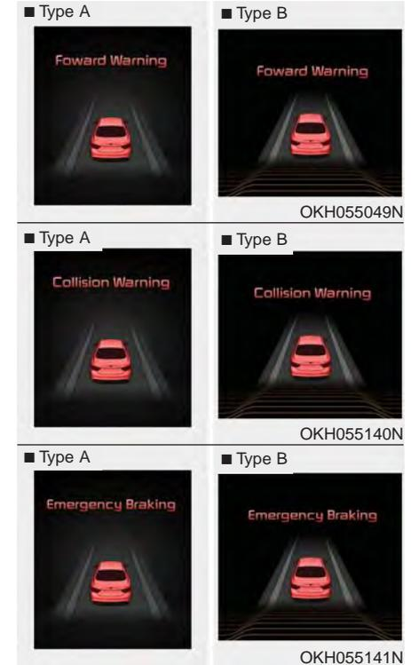
A warning message and chime will sound when you need to use the brake pedal or steering wheel due to a sudden stop or lack of distance with the vehicle ahead. The warning messages will vary according to the severity of the situation. Immediately reduce your speed to prevent a collision.
