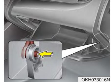
2. Open the glove box and remove the support strap.
