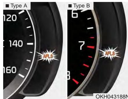
If the AFLS malfunction indicator comes on, the AFLS is not working properly. Drive to the nearest safe location and restart the engine. If the indicator remains on, have the system checked by an authorized K900 Kia dealer.
