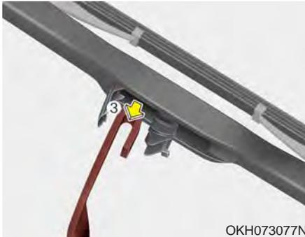
4. Push down the wiper arm (3) and install the new blade assembly in the reverse order of removal.
