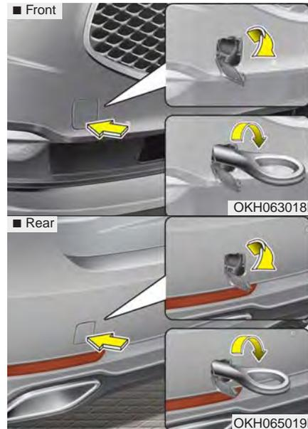
1. Open the trunk, and remove the towing hook from the tool case.
