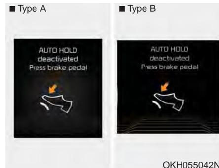
If you did not apply the brake pedal when you release the Auto Hold by pressing the [AUTO HOLD] switch, the notice will illuminate on the LCD display. Also, warning chime sounds once.
