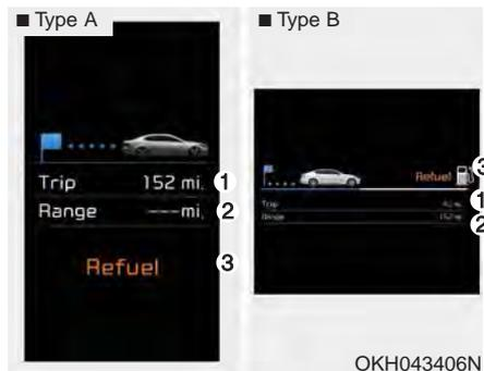
This display shows trip distance (1) and the vehicle can be driven with the remaining fuel (2).
