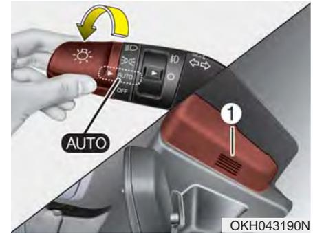
When the light switch is in the AUTO position, the taillights and headlights will be turned ON or OFF automatically depending on the amount of light outside the vehicle.
