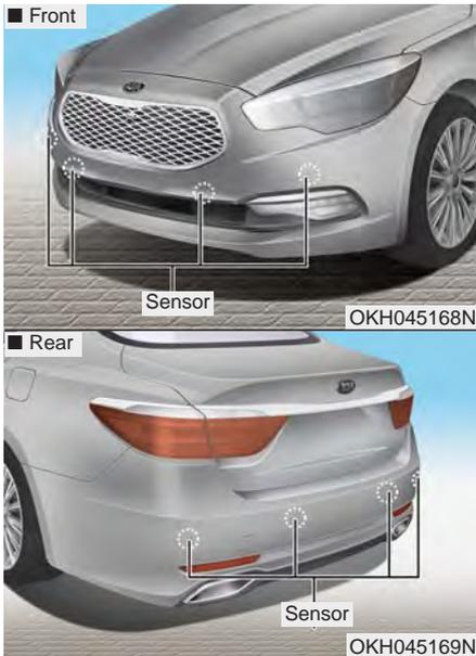
The Parking Assist System is not a substitute for proper and safe parking and backing-up procedures. Always drive safely and use caution when parking. The Parking Assist System may not detect every object behind or in front of the vehicle.
