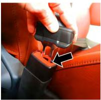
Inserting Latch Plate Into Buckle
