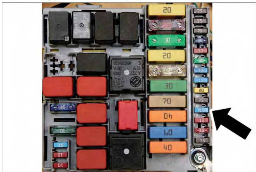
F15 Fuse 15 Amp Blue Cigarette Lighter/Power Outlet Front Console
