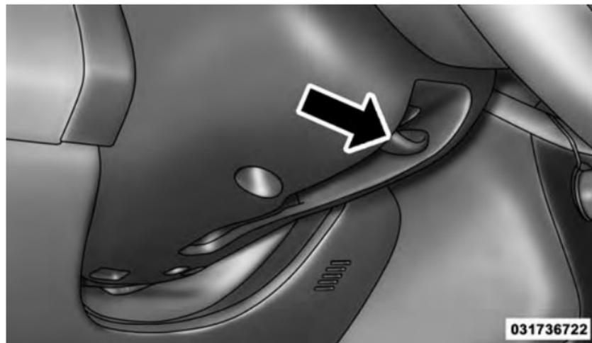
Tilt/Telescoping Steering Control Handle
