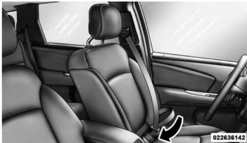
**Inserting Latch Plate Into Buckle**
