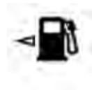
The arrow in this symbol is a reminder that the Fuel Filler Door is located on the left side of the vehicle.
