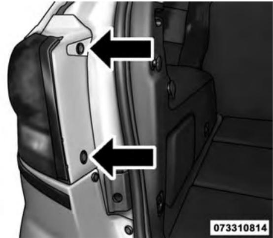
Inboard Tail Lamp Housing Fasteners
