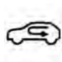
When outside air contains smoke, odors, or high humidity, or if rapid cooling is desired, you may wish to recirculate interior air by pressing the Recirculation control button. The recirculation indicator will illuminate when this button is selected. Push the button a second time to turn off the Recirculation mode and allow outside air into the vehicle.
