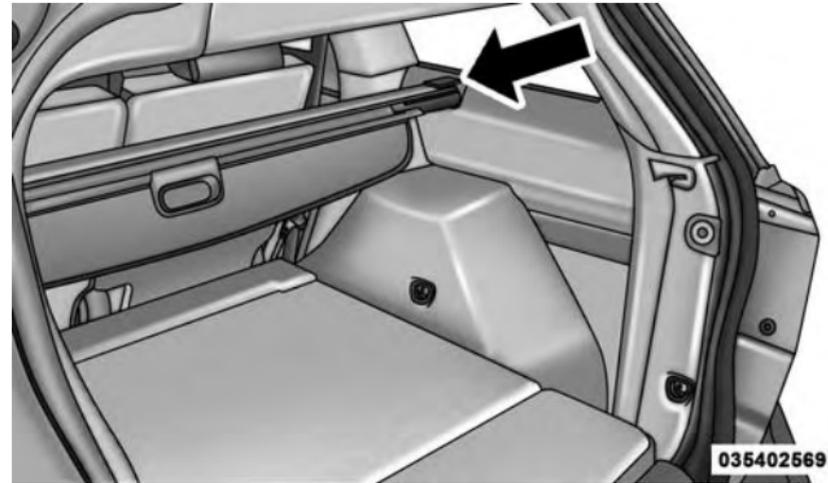
Installing Retractable Cargo Area Cover
