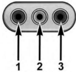
Audio/Video RCA Jacks (AUX Jacks) on the rear of the center console enable the monitor to display video directly from a video camera, connect video games for display on the screen, or play music directly from an MP3 player.
