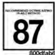
This engine is designed to meet all emissions regulations and provide excellent fuel economy and performance when using high-quality unleaded “Regular” gasoline having an octane rating of 87 as specified by the (R+M)/2 method. The use of higher octane “Premium” gasoline will not provide any benefit over “Regular” gasoline in these engines.
