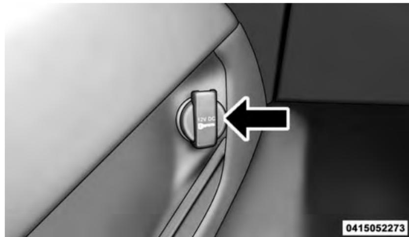
Power Outlet — Integrated Center Stack Front
