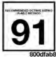
This engine is designed to meet all emission regulations, provide optimal fuel economy and performance when using high-quality unleaded "Premium" gasoline having a posted octane number of 91 as specified by the (R+M)/2 method. The use of 91 or higher octane "Premium" gasoline is required for in this engine.
