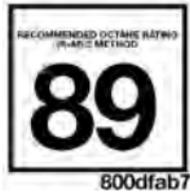
This engine is designed to meet all emissions regulations and provide satisfactory fuel economy and performance when using high quality unleaded gasoline having a posted octane number range of 87 to 89
