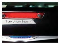
With a valid Keyless Enter-N-Go Key Fob located outside the vehicle and within 3 ft (1.0 m) of the deck lid, press the button on the located on the center of the light bar which is located on the deck lid above the license plate.
