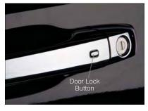
Both front door handles have LOCK buttons located on the outside of the handle. With one of the vehicle's Keyless Enter-N-Go Key Fobs located outside the vehicle and within 5 ft (1.5m) of the driver's or passenger front door handle, press the door handle LOCK button to lock all four doors and trunk
