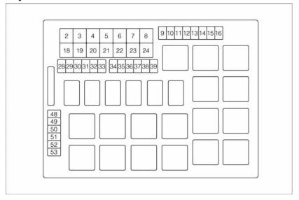
• The Integrated Power Module (fuses) is located in the engine compartment on the right hand side near the Washer Fluid Reservoir. This module contains fuses and relays.
