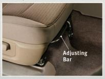
Lift up on the adjusting bar located at the front of the seat near the floor and release at the desired position, then release the handle to lock the seat into position.
