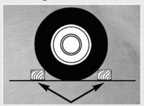
Block both the front and rear of the wheel diagonally opposite of the jacking position.
