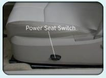
The power seat switch, located on the outboard side of the seat near the floor, controls forward/back, up/down, and tilt adjustment.
