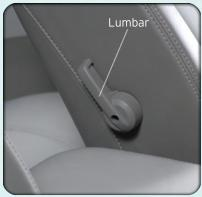
The lumbar control lever is on the inboard side of the seatback. Rotate the lumbar lever downward to increase the lumbar support or upward to decrease the lumbar support as desired.
