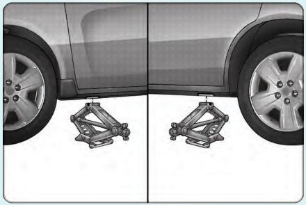
• Raise the vehicle by turning the jack screw clockwise. Raise the vehicle only until the tire just clears the surface and enough clearance is obtained to install the spare tire.
