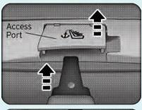
• Push the tether strap and hook through the access port and down into the trunk.
