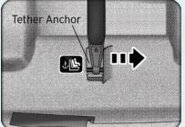
• Tighten all three straps as you push the child restraint rearward and downward into the seat.
