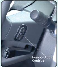
• The remote audio controls are located on the rear surface of the steering wheel.
