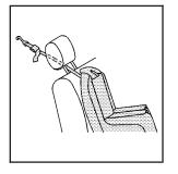
If the position you are using has an adjustable headrest or head restraint and you are using a single tether, route the tether under the headrest or head restraint and in between the headrest or head restraint posts.
