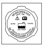
Remove the coolant surge tank pressure cap when the cooling system, including the coolant surge tank pressure cap and upper radiator hose, is no longer hot. Turn the pressure cap slowly counterclockwise. If you hear a hiss, wait for that to stop. A hiss means there is still some pressure left.
