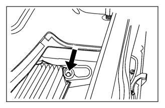
Then, insert a tool behind the push pin located on the inboard side of the air filter compartment to carefully pry the pin out.
