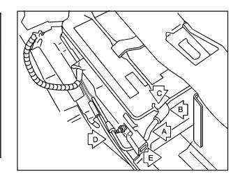
To be sure the vent hose (A) is properly attached, the vent hose connectors (B) must be securely reattached to the vent outlets (C) on each side of the battery and the vent assembly grommet (D) must be secured to the floor pan (E).
