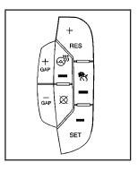
The FCA control is located on the steering wheel.
