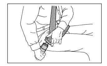
3. Push the latch plate into the buckle until it clicks. If the latch plate will not go fully into the buckle, check if the correct buckle is being used.
