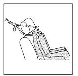
If the position you are using has a fixed or adjustable headrest or head restraint and you are using a dual tether, route the tether around the headrest or head restraint.
