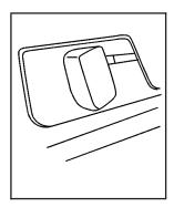
The adjustment lever is located on the left side of the steering column.
