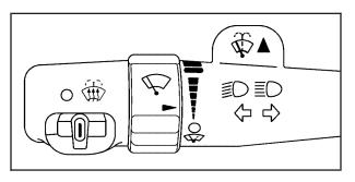
The windshield wiper lever is located on the left side of the steering column.
