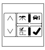
The DIC buttons are located on the instrument panel to the left of the steering wheel.
