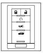
Press to unlock the driver door. Press again within five seconds to unlock all remaining doors.
