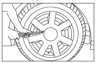
2. For models having aluminum wheels with a center wheel cover, use the flat end of the wheel wrench to gently pry the wheel covers off. Store the wheel cover and lug nut caps in the trunk until you have the flat tire repaired or replaced. Be careful not to scratch the aluminum wheel edge and do not try to remove it with your hands. Then loosen the wheel nuts with the wheel wrench. Do not remove them yet.
