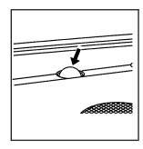
The solar sensor, located in the defrost grille, middle of the instrument panel, monitors the solar radiation. Do not cover the solar sensor or the system will not work properly.
