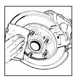
Remove any rust or dirt from the wheel bolts, mounting surfaces, and spare wheel. 11. Place the spare tire on the wheel-mounting surface.
