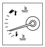
This gage shows the engine coolant temperature.
