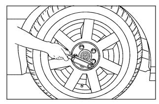
3. For models with exposed lug nuts, loosen them using the wheel wrench. Do not remove them yet.
