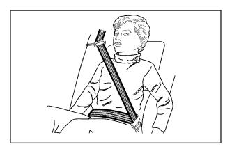
Buckle, position, and release the safety belt as described earlier in this section. Make sure that the shoulder belt crosses the shoulder.
