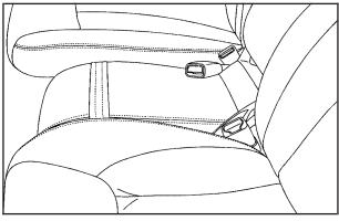
The vehicle may have a front center seat. This seat can be converted to a storage area by lowering the seatback. See *Center Flex Storage Unit on page 3-56*.
