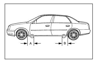
Find the jacking location from the diagram above and use the corresponding cutouts located in the plastic molding.
