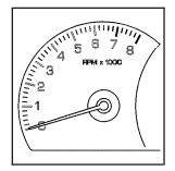
This gage indicates the engine speed in revolutions per minute (rpm).
