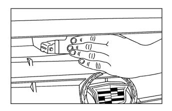
Then go to the front of the vehicle and find the secondary hood release lever, located near the center of the hood. Move the release lever up and to the right to raise the hood.
