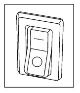
The valet lockout switch is located inside the glove box.
