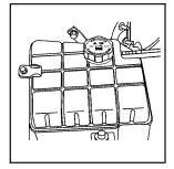
3. Fill the coolant surge tank with the proper mixture to the FULL COLD mark on the side of the coolant surge tank.
