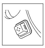
If the vehicle has this feature, the power tilt and telescope wheel control is located on the outboard side of the steering column.
