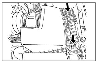
Remove the two screws on the top of the engine air cleaner/filter cover.
