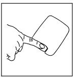
Press the area at the front of the handle located on the cover so that the back edge raises.
