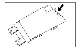
To access the fuse block, pull out and lift up on the cover latch, located at the end of the fuse block, near the battery cable.
