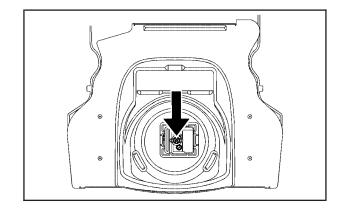
3. Turn the retainer clockwise and remove the tire sealant and compressor kit.
