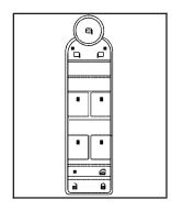
On vehicles with power windows, the switches are on the driver door armrest. Each passenger door has a switch that controls only that window.
