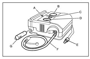
When using the tire sealant and compressor kit during cold temperatures, warm the kit in a heated environment for 5 minutes. This will help to inflate the tire faster.
