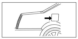
To open the fuel door, push the rearward center edge in and release and it will open.
