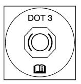
The brake master cylinder reservoir is filled with DOT 3 brake fluid. See Engine Compartment Overview on page 6-12 for reservoir location and access.
