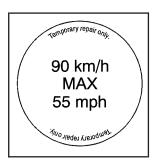
16. If the flat tire was able to inflate to the recommended inflation pressure, remove the maximum speed label from the sealant canister and place it in a highly visible location. The label is a reminder not to exceed 55 mph (90 km/h) until the damaged tire is repaired or replaced.
