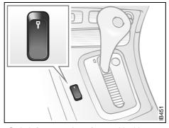
Switch for operation of central locking
