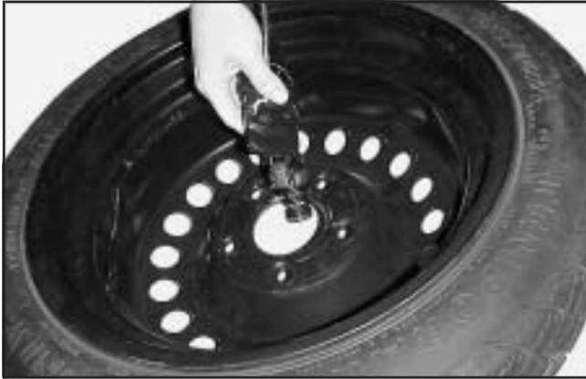
8. Tilt the retainer and slip it through the wheel opening to remove the compact spare tire from the cable.
