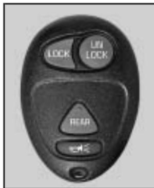
With this feature, you can lock and unlock your doors from about 3 feet (1 m) up to 30 feet (9 m) away using the remote keyless entry transmitter supplied with your vehicle.
