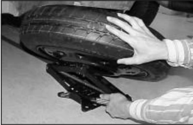
8. Disconnect the wrench from the jack and carefully remove the jack. Use one hand to push against the spare tire while firmly pulling the jack out from under the spare tire with the other hand.
