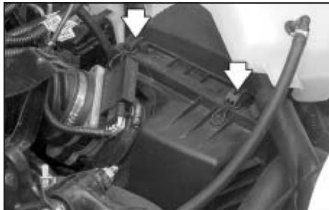
3. Unlatch the two hooks on top of the engine air cleaner/filter housing.
