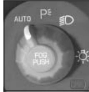
The control located to the left of the steering column operates the exterior lamps.
