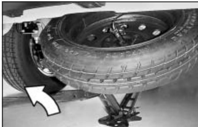
7. Lower the jack by turning the folding wrench counterclockwise. Keep lowering the jack until the spare tire slides off the jack.
