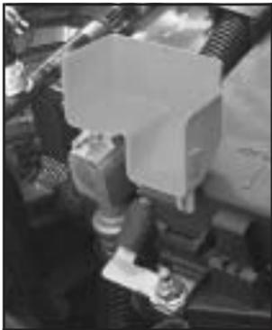
Pull up on the cap to access the remote positive (+) terminal. You should always use the remote positive (+) terminal instead of the positive (+) terminal on the battery.
