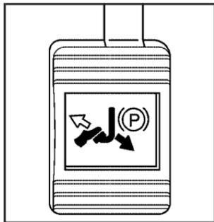
The parking brake is located under the instrument panel on the driver's side of the vehicle.
