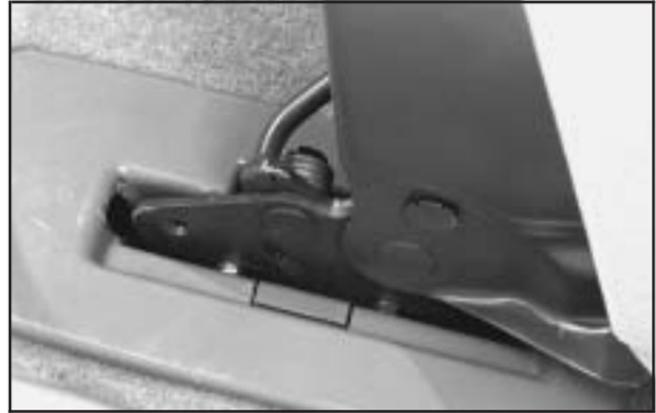
3. Firmly push the rear hooks onto the rear floor pins by pushing down on the rear of the seat.
