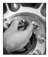
9. After mounting the spare, put the wheel nuts back on with the rounded end of the nuts toward the wheel.
