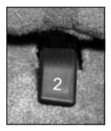
3. To unlatch the rear of the seat from the floor, pull up on the release lever labeled 2, at the rear of the seat, and lift the rear of the seat up from the floor.
