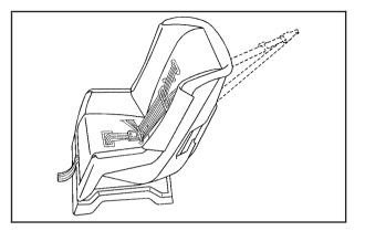
In Canada, the law requires that forward-facing child restraints have a top strap, and that the strap be anchored. In the United States, some child restraints also have a top strap. If your child restraint has a top strap, it should be anchored.
