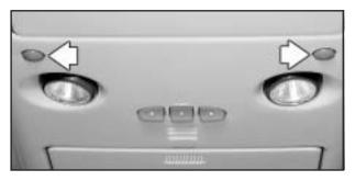
Your vehicle has reading lamps located in the overhead console. Press the button located next to the lamp to turn it on. The lamps can be adjusted to point in the direction you want.
