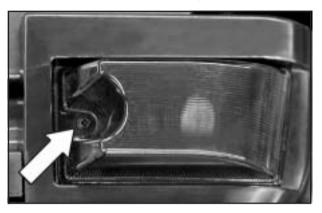
1. Remove the screw and lift off the lens.
