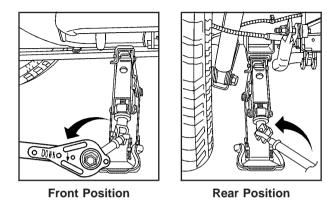
Lower the vehicle by turning the ratchet counterclockwise, with the DOWN mark facing you. Then lower the jack completely.
