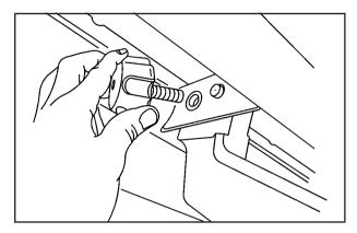
Thread the knob through the remaining hole — first into the rocker panel protector and then into the threaded hole in the side step bracket.
