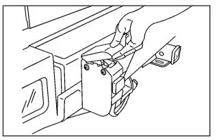
1. Lift the latch located on the left side of the tire carrier to release it.
