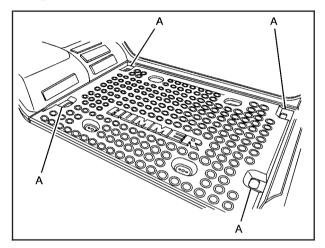
Your vehicle also has four cargo-area floor drains (a) located under the cargo mat, if equipped, near the sides of the cargo area. These drains should be cleaned periodically to allow water to exit the cargo area.
