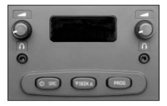
**(Power):** Press this button to turn the system on or off. The rear speakers will be muted when the power is turned on unless your vehicle is equipped with the Bose<sup>®</sup> audio system.
