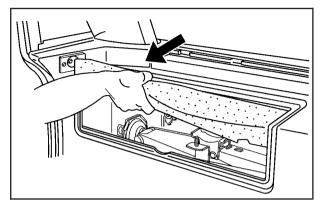
3. Pull the tool bag up and out from the front retention clip.
