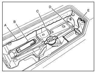
2. Place the jack (B) in the mounting bracket in the rear cargo compartment.
