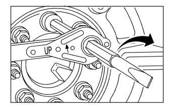
Tighten each wheel nut by hand. Then use the ratchet/wheel wrench to tighten the nuts, with the UP mark facing you, clockwise until the wheel is held against the hub.
