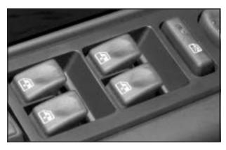
A power window switch is located on the armrest of each side door. The switches operate while the ignition is in RUN or ACCESSORY or while Retained Accessory Power (RAP) is active. See *Retained Accessory Power (RAP) on page 2-26.*
