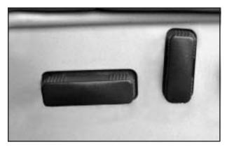
The power seat controls are located on the outboard edge of the front seats.
