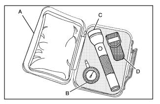
The tire pressure gage has a reset button in the gage stem. After taking a pressure reading, press the button to reset the gage to zero.
