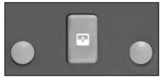
The vehicle may have a power sliding sunroof. To operate it, the ignition or RAP must be in the ON position. The switch used to operate the sunroof is located in the overhead console.
