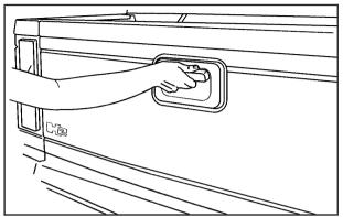
3. Open the tailgate by lifting the release handle while pulling the tailgate toward you.
