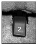
2. Unlatch the seat from the floor by pulling up on the lever labeled 2, located on the rear of the seat.
