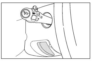
The tilt lever is located on the driver's side of the steering column under the turn signal lever.
