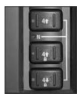
The transfer case buttons are located to the right of the instrument panel cluster. Use these switches to shift into and out of the different all-wheel drive modes. You can choose between four modes:
