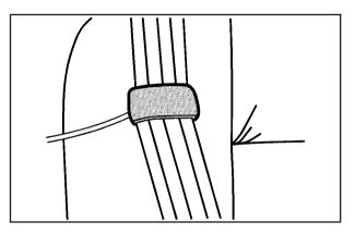
3. Be sure that the belt is not twisted and it lies flat. The guide must be on top of the belt.
