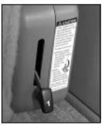
1. Pull up on the release lever labeled 1, located on the rear of the seatback, and push the seatback forward.
