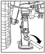
**Rear Flat Tire:** Place the jack under the curved rear axle pad. Make sure the jack head is positioned so that the rear axle pad is resting securely on the jack head.
