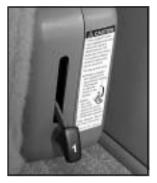
1. Pull up on the release lever labeled 1 and then pull up on the seatback until the seatback locks into the upright position.
