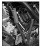
The remote positive (+) terminal is located near the engine accessory drive bracket. On some vehicles, the terminal may be covered by a red plastic cover. To access the remote positive (+) terminal, open the cover.
