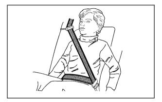
Buckle, position and release the safety belt as described in *Rear Seat Passengers on page 1-30*. Make sure that the shoulder belt crosses the shoulder.
