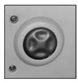
You can increase or decrease lumbar support in an area of the lower seatback with this control, located on the outboard sides of the front seat(s). You can also reshape the side wing area of the lower seatback for more lateral support.
