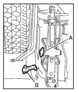
2. Turn the wingnut (A) counterclockwise to release the jack.
