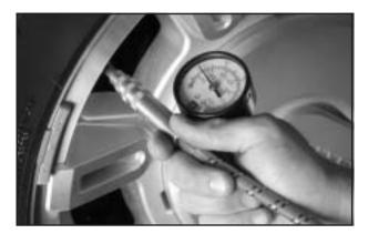
The accessory inflator hose also has a built-in air pressure gage. As soon as you start to inflate an object it will automatically read the current pressure.
