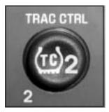
To enter this mode, press the TC2 button located on the instrument panel to the right of the steering wheel.
