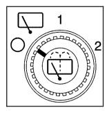
If your vehicle has a rear window washer/wiper, this knob is located on the instrument panel to the left of the steering wheel.
