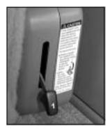
5. Pull up on the release lever labeled 1 and then pull up on the seatback until the seatback locks into the upright position.
