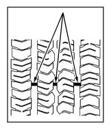
One way to tell when it's time for new tires is to check the treadwear indicators, which will appear when your tires have only 1/16 inch (1.6 mm) or less of tread remaining. Some commercial truck tires may not have treadwear indicators.
