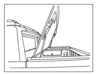
You will be able to open the cover by turning the cover release latch in a clockwise direction, which will allow you to lift the cover with the assistance of the struts.
