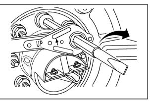
4. Use the ratchet and wheel wrench to tighten the nuts firmly. Try to move the tire back and forth slightly to be sure it is secure.
