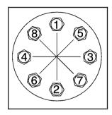
12. Tighten the nuts firmly in a crisscross sequence as shown by turning the ratchet clockwise, with the UP mark facing you.
