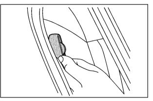
1. Remove the guide from its storage clip on the side of the seatback.
