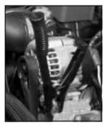
The remote negative (–) terminal is located on the engine accessory drive bracket and is marked GND.
