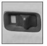
To unlock or lock the door from the inside, slide the manual lever forward or rearward.
