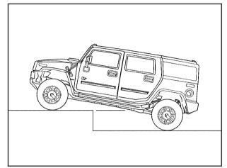
Your vehicle can climb a 16 inch (40.6 cm) vertical step. Step climbing is best done by approaching the step at an angle rather than straight on.
