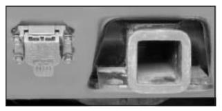
Your vehicle is equipped with a trailer towing harness. This harness with a seven-pin universal heavy-duty trailer connector is attached to a bracket on the hitch platform. The trailer towing harness contains the following trailer circuits:
