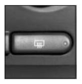
If the vehicle has heated mirrors, the button to turn this function on or off is located on the climate control panel.
