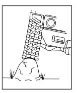
Do not straddle large rocks; drive over them, letting the tire envelop the rock. The tread of the tire is thicker and tougher than the sidewall of the tire and is more resilient to impact than underbody components.
