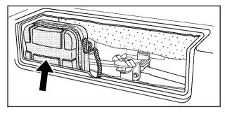
You will first need to remove the tool kit/first aid kit to allow you enough room to remove the tire changing equipment. Once removed, you will see the following tire changing equipment:
