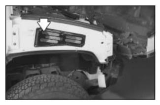
*Notice:* If you spray water into the engine air cleaner/filter intake and water enters the engine air cleaner/filter housing, as shown in the illustration, you could damage your vehicle's engine. The repairs would not be covered by your warranty. Do not spray water into the engine air cleaner/filter intake and/or housing.
