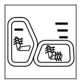
Your vehicle may have heated front seats. The buttons used to control this feature are located on the front doors. The engine must be running for the heated seat feature to work.
