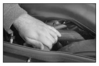
5. With the coolant surge tank pressure cap off, start the engine and let it run until you can feel the upper radiator hose getting hot. Watch out for the engine cooling fan.
