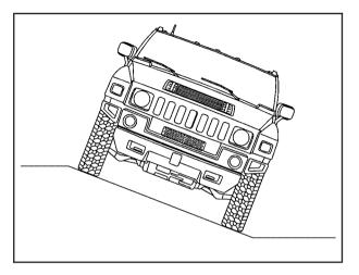
Also, your vehicle should be able to traverse a 40%  $(22^{\circ})$  side slope at 6 mph (9.7 km/h) while fully loaded on high friction surfaces.
