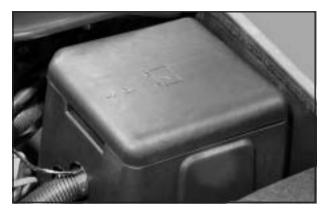
The underhood fuse block in the engine compartment is located on the driver's side of the vehicle near the battery. Lift the cover for access to the fuse/relay block.
