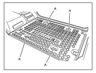
There are four oval shaped openings (A) in the cargo bed that allow access to four tie downs. You can use these tie downs to secure cargo.
