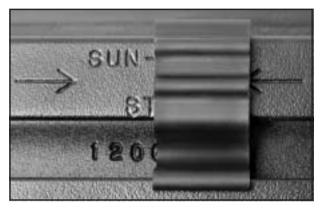
If your vehicle has a sunroof, it will have a crossrail stop tab placed in the siderail in the spot labeled SUN—ROOF STOP. This tab prevents you from moving the crossrails past the opening of the sunroof and loading cargo too far forward.
