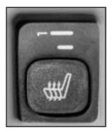
If your vehicle has this feature, the buttons used to control this feature are located on the back of the center console. The engine must be running for the heated seat feature to work. To heat the seat, press the button to cycle through the temperature settings of high and low. Press the button a third time to turn the feature off. An indicator light will glow for each heat setting when the feature is operating.
