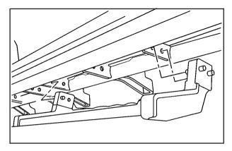
Guide the pins on the side step brackets into the holes in the vehicle's rocker panel protector brackets. If you have difficulty doing this, it may help to have someone hold up the step while you guide the pins into the holes.
