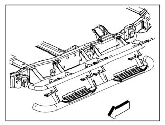
The driver's side of the vehicle is shown with the body removed for clarity. To remove a step:
