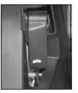
2. Pull the handle located inside the vehicle to the lower left of the steering wheel.
