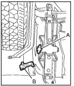
Tighten the wingnut (A) until the jack is securely fastened.
