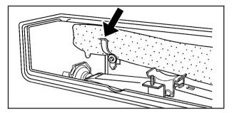
7. Push the front of the tool bag down into the front retention clip.
