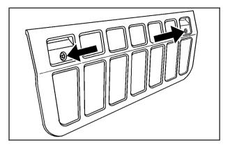
3. Press either one of the two power midgate latch release buttons. The midgate will move slightly forward from its closed position. The latch release buttons operate while the ignition is in RUN, ACCESSORY, in RAP mode, or up to ten minutes after removing the key. If necessary, press the global express-down button to reactivate the release buttons for an additional ten minutes.
