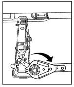
**Front Flat Tire:** Position the jack under the vehicle on the frame behind the flat tire where the frame sections overlap. See the graphic following for an approximate measurement of the jack location on the frame.
