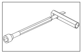
2. Place the flat end of the wheel wrench through the hole in the spanner wrench.
