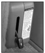
2. Fold the seatback forward onto the seat cushion by using the lever labeled 1. The seat cannot be removed unless the seatback is folded.
