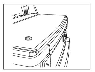
Your tonneau cover will have two lock cylinders on it. One lock cylinder is to secure the cover closed and the other lock cylinder will allow you to secure the tailgate close.
