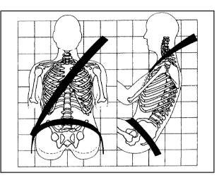
The lap part of the belt should be worn low and snug on the hips, just touching the thighs. In a crash, this applies force to the strong pelvic bones. And you would be less likely to slide under the lap belt. If you slid under it, the belt would apply force at your abdomen. This could cause serious or even fatal injuries. The shoulder belt should go over the shoulder and across the chest. These parts of the body are best able to take belt restraining forces.
