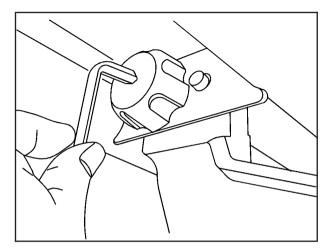
5. Hand-tighten the knob by turning it clockwise until it is seated against the rocker panel protector bracket and then tighten it to 10 lb ft (13.5 N•m) with the tool as shown.
