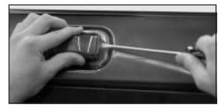
1. Push in on the notch with a flat tool and pull the lamp out.
