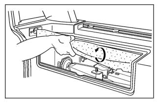
6. Slide the tool bag into the rear retention clip. It may help to twist the tool bag as you slide it into the rear retention clip.
