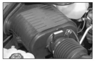
1. Loosen the screws on the engine air cleaner/filter cover.
