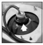
2. Turn the bulb/socket retainer counterclockwise to unlock the bulb/socket. You may prefer to unplug the electrical connector before removing the bulb/socket. If so. complete Step 4 before doing this step.
