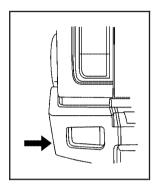
1. Locate the affected taillamp which is behind and under the bumper.
