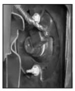
Locate the lamp assembly behind the front bumper. It is easiest to come in from the side of the vehicle through the wheel opening.
