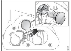
If a brake light bulb fails, the adjacent taillight will act as a brake light to ensure traffic safety. Change the broken bulb when possible.
