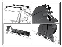
Mounting holes for roof carrier
