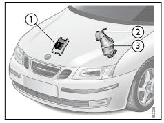
Engine management system with catalytic converter
