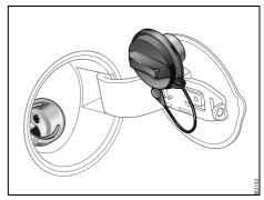
Filler cap removed for refueling
