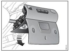
Hatch opened for replacement of center bulb
