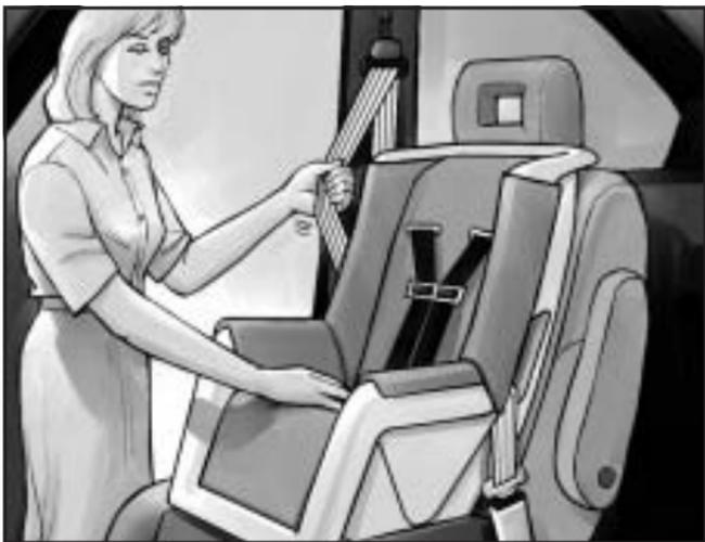
5. To tighten the belt, pull up on the shoulder belt while you push down on the child restraint. You may find it helpful to use your knee to push down on the child restraint as you tighten the belt.
