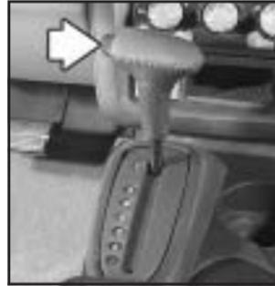
2. Move the shift lever into PARK (P). To do so, hold in the button on the lever, then push the lever all the way toward the front of the vehicle
