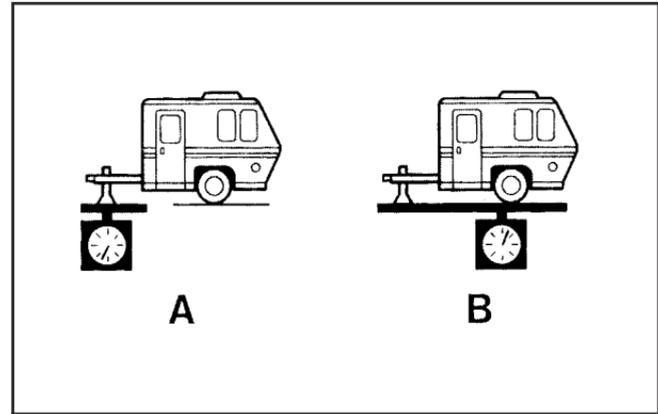
If you are using a weight-carrying or a weight-distributing hitch, the trailer tongue weight (A) should be 10 percent to 15 percent of the total loaded trailer weight (B). Do not exceed the maximum allowable tongue weight for your vehicle.
