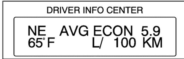
If your vehicle is equipped with the Driver Information Center (DIC), the display is located on the instrument panel cluster directly above the steering column. The DIC will show information about the vehicle and the surroundings.
