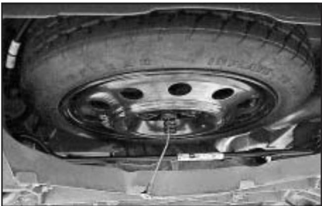
If the spare tire will not lower, the secondary latch may be engaged causing the tire not to lower. Do the following to check the cable:
