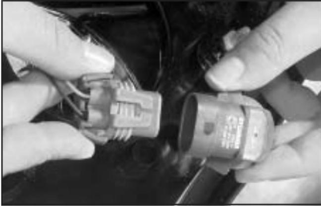
8. Unhook the electrical connector by lifting up the gray tabs and separate the connector from the bulb base.
