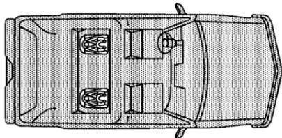
Your vehicle has the LATCH system. You will find anchors (A) in both rear seat outside passenger positions.
