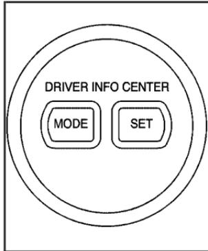
The DIC controls are located to the right of the instrument panel cluster.
