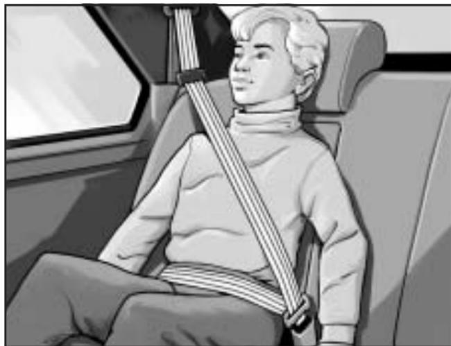
4. Buckle, position and release the safety belt as described in *Rear Seat Passengers* on page 1-28. Make sure that the shoulder belt crosses the shoulder.
