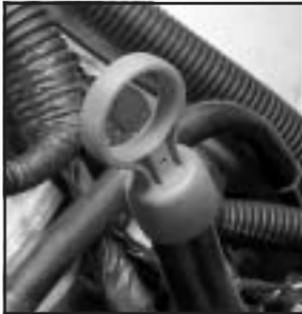
The dipstick is located toward the back of the engine compartment, next to the brake master cylinder.
