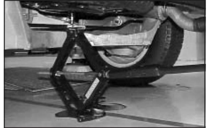
4. Turn the folding wrench clockwise to raise the jack until it lifts the secondary latch spring.
