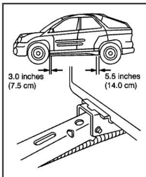
3. Near each wheel, there is a notch in the vehicle's body. Position the jack and raise the jack head until it fits firmly into the notch in the vehicle's frame nearest the flat tire.
