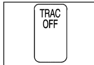
To turn the system off, press the TRAC OFF button located on the instrument panel switchbank.
