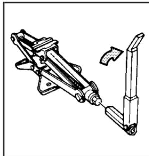
4. Attach the folding wrench to the jack, and turn the wrench clockwise to raise the jack head 3 inches (7.6 cm).
