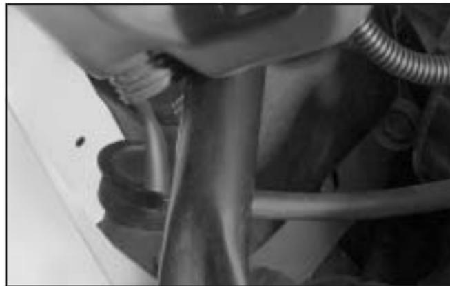
3. After the engine cools, open the coolant air bleed valves.
