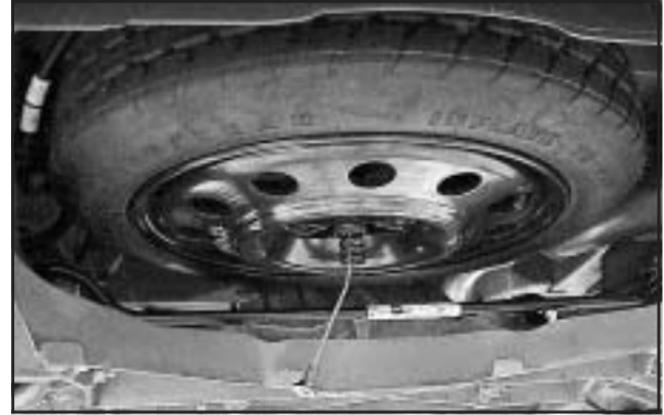
9. To remove the compact spare tire from the cable, tilt the retainer and slip it through the wheel opening.
