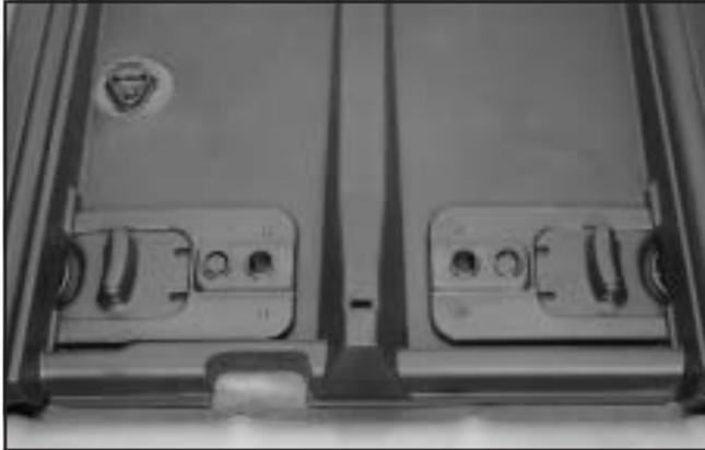
1. Feed the tethered ring through the rear lower sidewall loop on each side of the vehicle.
