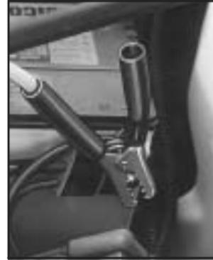
8. Now connect the black negative (-) cable to the negative (-) terminal of the good battery. Use a remote negative (-) terminal if the vehicle has one.
