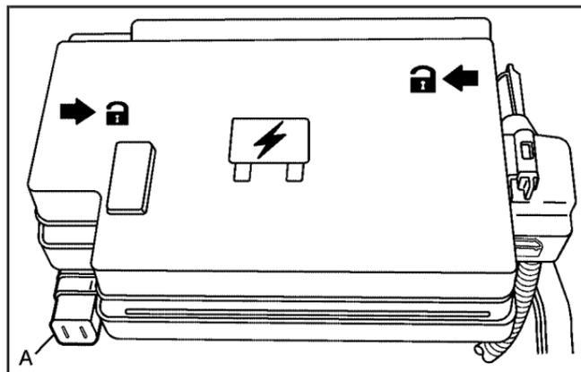
This fuse block is located in the engine compartment on the passenger's side of the vehicle. See *Engine Compartment Overview* on page 5-12 for more information on location.
