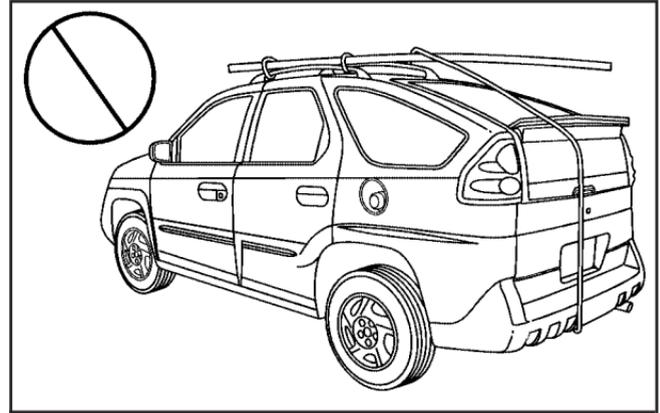
If you have the luggage carrier, you can load things on top of your vehicle. If you do load things on the top of your vehicle, you must load them on the luggage carrier crossrails. The luggage carrier has four tie-down loops on the inside of each right and left side rail. These let you secure cargo placed on the crossrails, as long as they are not wider or longer than the luggage carrier.
