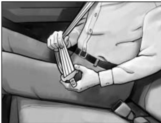
If the belt stops before it reaches the buckle, tilt the latch plate and keep pulling until you can buckle it. Pull up on the latch plate to make sure it is secure. If the belt is not long enough, see *Safety Belt Extender* on page 1-38.
