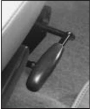
Pull up on the lever, located on the front of the seat, to unlock and move the seat.
