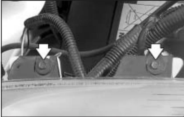
2. Remove the two inboard screws attaching the lamp to the fender bracket.
