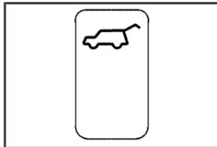
To open the liftgate from the inside of the vehicle, press the liftgate release button located on the instrument panel switchbank.
