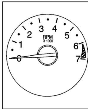
The tachometer displays the engine speed in revolutions per minute (rpm).
