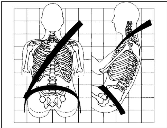
The lap part of the belt should be worn low and snug on the hips, just touching the thighs.
