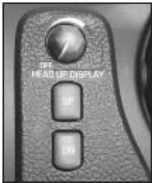
The HUD controls are located to the right of the instrument panel cluster.
