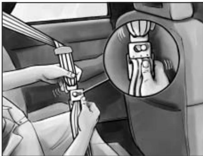
2. Insert the metal knob on the shoulder belt into the keyhole on the lap belt buckle as shown. Be sure to slide the shoulder belt part into the keyhole until it locks into place.
