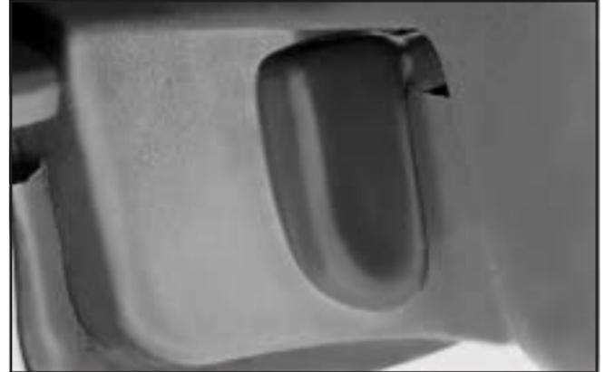
The lever that allows you to tilt the steering wheel is located on the left side of the steering column. To tilt the wheel, hold the wheel and pull the lever. Then move the wheel to a comfortable position and release the lever to lock the wheel in place.
