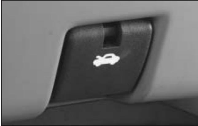
1. Pull the hood release handle, located under the instrument panel on the driver's side of the vehicle.
