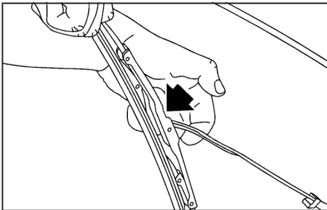
5. Push the release clip, located at the connecting point of the blade and the arm, in the up position. Then, pull the blade assembly down toward the glass to remove it from the wiper arm.
