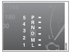
Selector-lever indicator on main instrument panel
