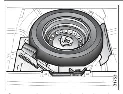
Stowage of spare wheel and tools under trunk floor
