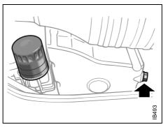
Drain plug and oil filter, 4-cylinder engine
