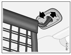
Attaching the cargo net to the roof
