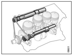
Balance shafts, 4-cyl. engine
