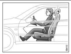
Correctly positioned safety belt
