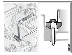
Correct position for battery clamp
