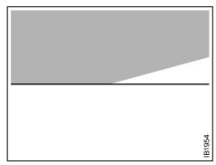
Correctly adjusted low beam
