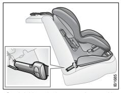
Semi-rigid 2-point lower attachment with top tether
