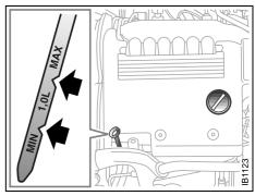
Engine-oil dipstick and filler cap, 3.0t V6
