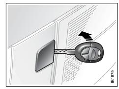
Use the key to pry out the cover plate covering the lock, 9-5 Wagon
