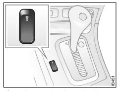
Switch for operation of central locking
