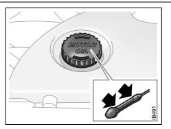
Engine-oil filler cap and dipstick, 4-cylinder engine
