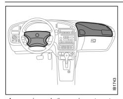
Accessories and other equipment must not be fitted to the surfaces marked as these are where the airbags inflate in the event of a crash.
