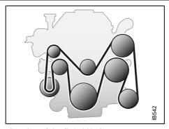
Routing of the Poly-V-belt: 4-cylinder engine
