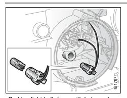
Parking-light bulb (cars with halogen low beam)
