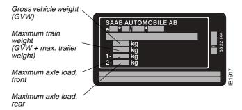
Permissible load (in addition to driver) = GVW minus curb weight
