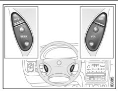
Audio System controls on steering wheel
