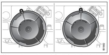
Make sure the cover is correctly fitted before locking it in place
