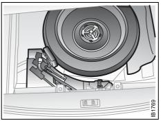
The car's ground clearance is reduced with the compact spare fitted. Note that only one compact spare wheel may be used at any time. Take care not to hit the curb and do not fit snow chains. Leave the wheel cover off, so that the warning text is readily visible.
