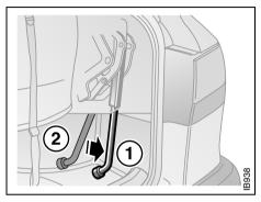
Tool fitted for manual unlocking (1) or locking (2) of the tonneau cover
