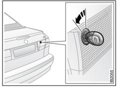
Unlocking the trunk lid with the key
