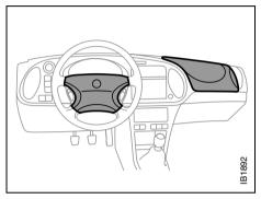
Accessories and other equipment must not be fitted to the surfaces marked as these are where the airbags may inflate in the event of a crash.
