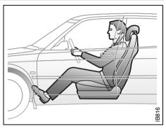
Correctly positioned safety belt.
