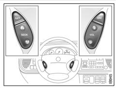
Audio System controls on steering wheel
