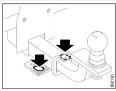
Attach the safety chains to the holes as illustrated.
