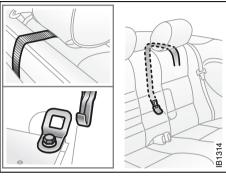
Attaching tether strap hook to anchorage. The tether strap is not a part of the tether child anchorage.
