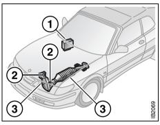
Engine-management system with catalytic converter
