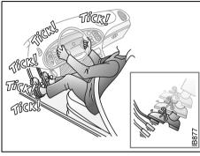
ABS braking - confirmation that the system is operating
