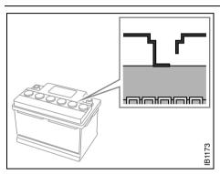
Correct fluid level in the battery
