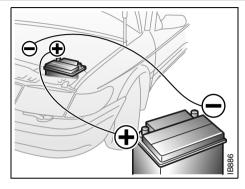
4 Open the hood and locate the battery. Find the positive (+) and negative (-) terminals on the battery.
