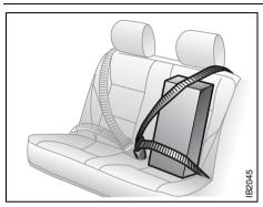
Securing a load on the rear seat
