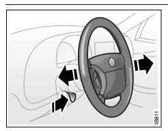
Lever for steering-wheel adjustment
