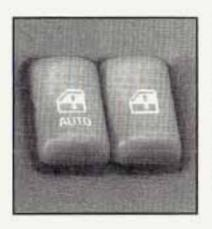
If your vehicle has this feature, the switches on the center console control each of the power windows when the ignition is on. In addition, on four-door models, each rear passenger door has a control switch for its own window.
