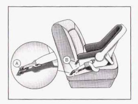
With this system, use the LATCH system instead of the vehicle's safety belts to secure a child restraint.
