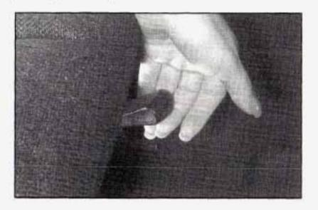
If your vehicle is not equipped with easy entry seats, your passenger seat adjuster looks like this. Slide the lever located under the passenger's seat to the right to unlock it. Slide the seat to where you want it and release the lever. Then try to move the seat with your body, to make sure the seat is locked into place.
