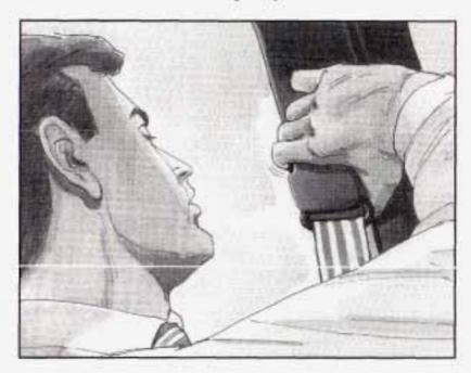
To move it down, squeeze the release button and move the height adjuster to the desired position. You can move the adjuster up just by pushing up on the shoulder belt guide. After you move the adjuster to where you want it, try to move it down without squeezing the release button to make sure it has locked into position.
