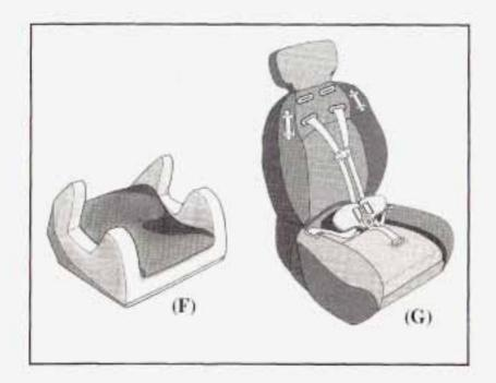
A booster seat (F-G) is a child restraint designed to improve the fit of the vehicle's safety belt system. Some booster seats have a shoulder belt positioner, and some high-back booster seats have a tive-point harness. A booster seat can also help a child to see out the window.
