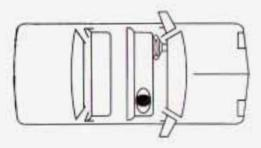
Your vehicle has a right front passenger air bag. Never put a rear-facing child restraint in this seat. Here's why:
