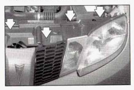
After opening the hood remove the plastic fasteners holding the shield. Use a tool to pry up the center of the fastener. Be careful not to break the fasteners that hold the shield in place.
