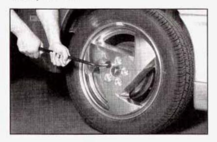
If your vehicle is equipped with wheel covers, use the wheel wrench to begin loosening the plastic wheel nut caps. Once you have loosened the plastic wheel nut caps with the wheel wrench you can finish loosening them with your fingers. Using the flat end of the wheel wrench, pry along the edge of the wheel cover until it comes off.
