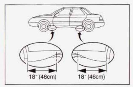
Near each wheel well is a notch in the frame which the jack head fits in. The front notch is 9 inches (23 cm) back from the front wheel well. The rear notch is 8 inches (20 cm) forward from the rear wheel well. As is shown by the diagram, if your vehicle has flared side moldings, both front and rear notches are 18 inches (46 cm) from the wheel wells.
