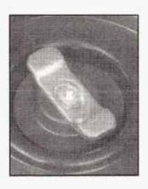
Turn the wing bolt counterclockwise and remove it. Then lift off the adapter and remove the compact spare tire.
