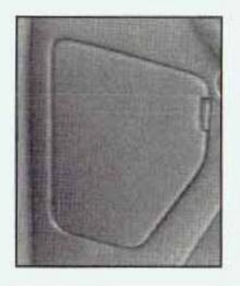
The instrument panel fuse block is located on the driver's side end of the instrument panel.
