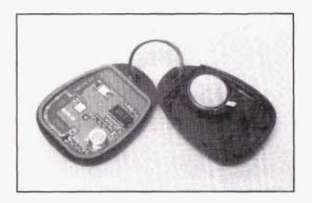
To replace the battery in the transmitter:
