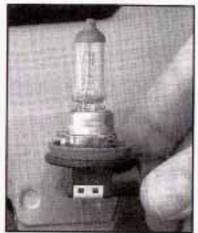
Disconnect the bulb base from the socket by lifting the plastic locking tab.
