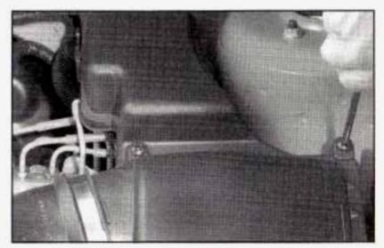
To check or replace the filter, remove the screws that hold the cover on and lift off the cover. Be sure to reinstall the cover tightly. Refer to the Maintenance Schedule to determine when to replace the air filter.
