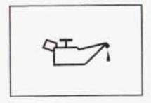
If the oil pressure light appears on the instrument cluster, it means you need to check your engine oil level right away.
