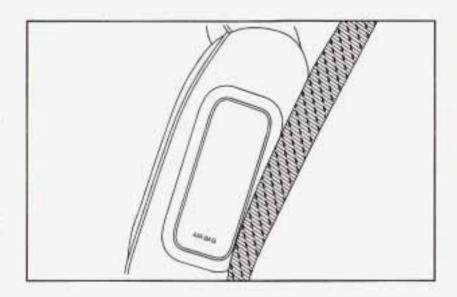
If your vehicle has a side impact air bag for the right front passenger, the words AIR BAG will appear on the air bag covering on the side of the right front passenger's seatback closest to the door.
