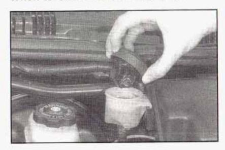
Refer to the Maintenance Schedule to determine how often you should check the fluid level in your master cylinder reservoir and for the proper fluid. See Part B: Owner Checks and Services on page 6-17 and Part D: Recommended Fluids and Lubricants on page 6-24.
