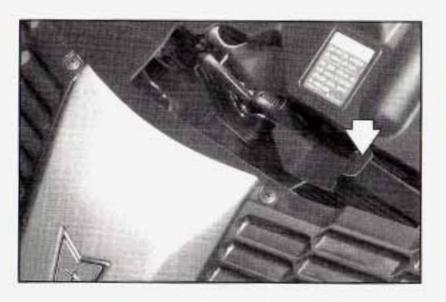
Then go to the front of the vehicle and lift up on the secondary hood release lever. The secondary hood release lever is located near the front center of the hood toward the driver's side.
