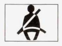
The safety belt light will also come on and stay on for several seconds, then it will flash for several more. If the air bag readiness light stays on after you start the vehicle or comes on when you are driving, your air bag system may not work properly. Have your vehicle serviced right away.
