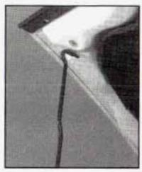
Lift the hood, release the hood prop from its retainer and put the hood prop into the slot in the hood marked by an arrow. Use the prop rod sleeve when handling the prop rod.
