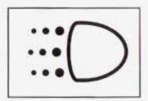
This indicator light on your instrument panel cluster will come on when the DRL are on. A flashing DRL telltale indicates a possible burned out headlamp, or that the vehicle may need service to repair a stuck DRL relay.
