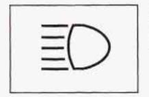
When the high beams are on, this light on the instrument panel cluster will also be on.
