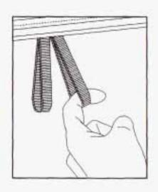
Pull the release straps located in the trunk. The right strap operates the passenger's side rear split seat. The left strap operates the driver's side rear split seat.
