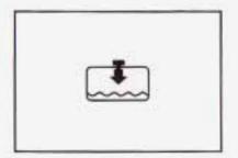
If the low coolant light comes on and stays on, it means you're low on engine coolant. See Low Coolant Warning Light on page 3-28.
