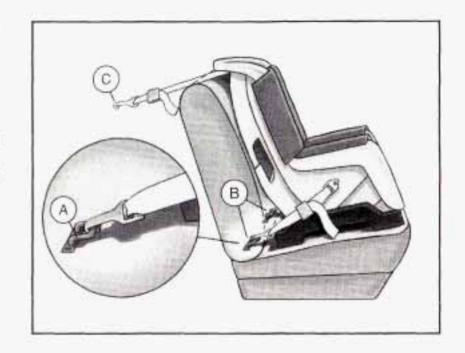
In order to use the system, you need either a forward-facing child restraint that has attaching points (B) at its base and a top tether anchor (C), or a rear-facing child restraint that has attaching points (B), as shown here.
