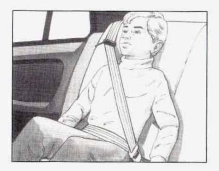
Buckle, position and release the safety belt as described in Rear Seat Passengers on page 1-23. Make sure that the shoulder belt crosses the shoulder.
