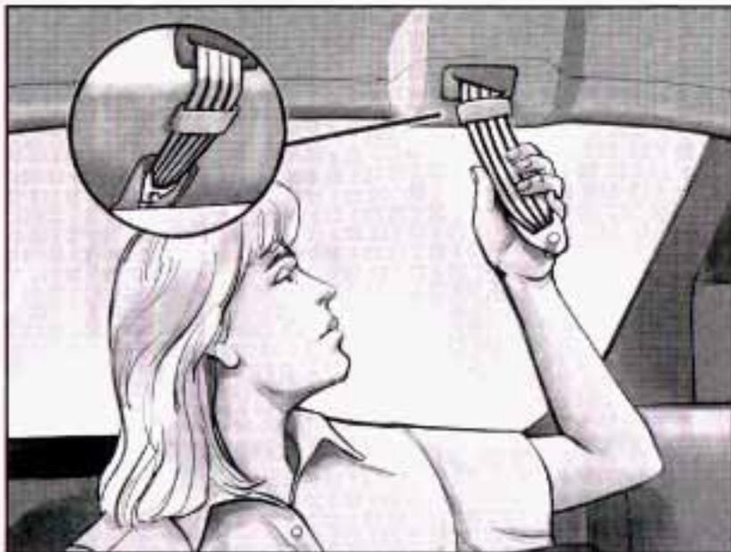
1. Remove the shoulder belt from its stowage location in the roof and pull it all the way down to the lap belt.
