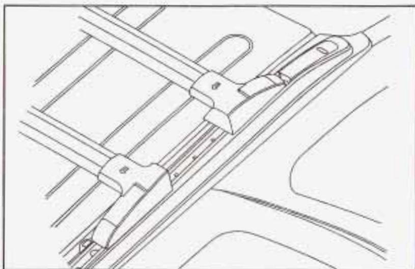
**Notice:** Loading cargo that weighs more than 220 lbs. (100 kg) on the luggage carrier may damage your vehicle.
