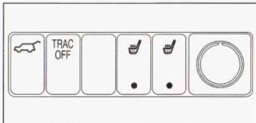
There is an instrument panel switchbank located below the comfort controls. It contains switches or blanks that will vary with the options that are on your vehicle and a cigarette lighter/accessory power outlet.
