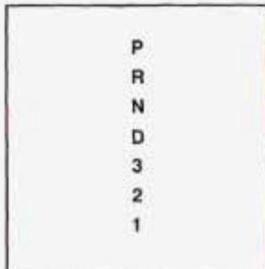
Maximum engine speed is limited when you're in PARK (P) or NEUTRAL (N), to protect driveline components from improper operation.
