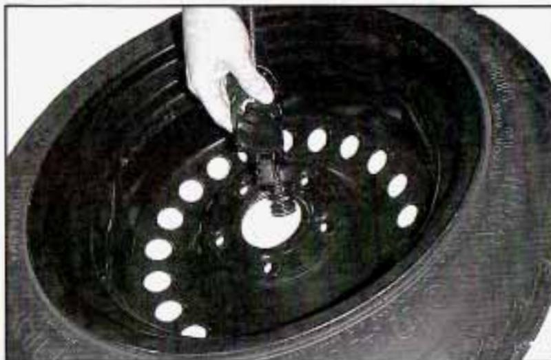
4. To remove the spare tire from the cable, tilt the retainer and slip it through the wheel opening.
