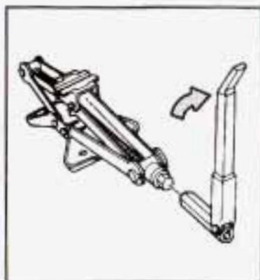
4. Attach the folding wrench to the jack, and turn the wrench clockwise to raise the jack head 3 inches (7.6 cm).
