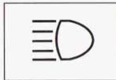
When the high beams are on, this light, on the instrument panel cluster and the HUD display, will also be on.
