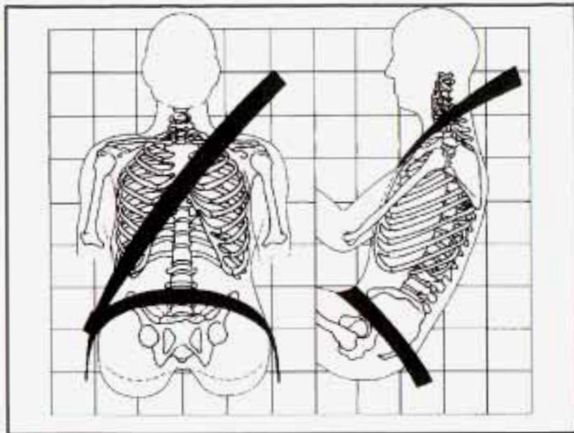
The lap part of the belt should be worn low and snug on the hips, just touching the thighs.
