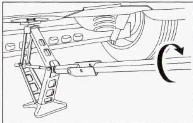
1. Turn the wrench counterclockwise until approximately 6 inches (15 cm) of cable is exposed.
