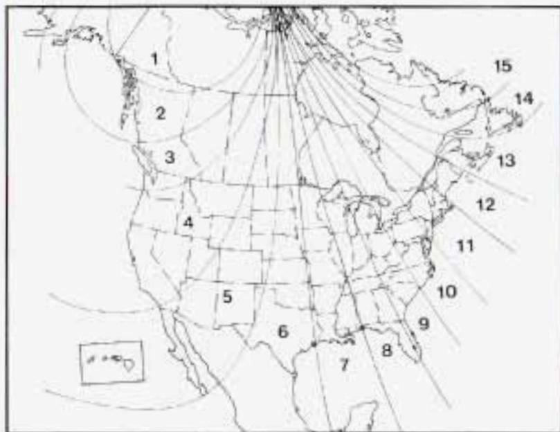
**ZONE # PRESS & HOLD SET TO CHANGE:** This display mode will be displayed when you are manually calibrating the system. The current zone number for compass variance will be displayed in place of the # symbol. Use the SET button to select the zone number from the graphic shown to select the current area of the country that you are driving in.
