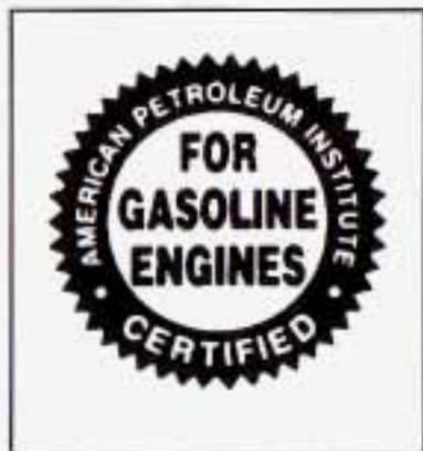
If you choose to perform the engine oil change service yourself, be sure the oil you use has the starburst symbol on the front of the oil container. If you have your oil changed for you, be sure the oil put into your engine is American Petroleum Institute certified for gasoline engines.
