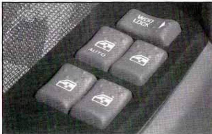
Switches on the drivers door armrest control each of the windows when the ignition is in ON, ACCESSORY, or when Retained Accessory Power is active. See "Retained Accessory Power (RAP)" under *Ignition Positions* on page 2-22 for more information. In addition, each passenger's door has a window switch.
