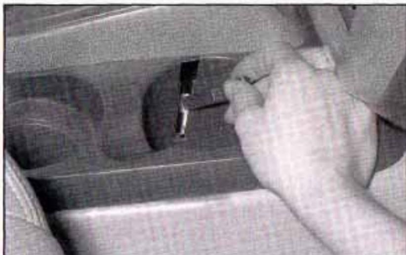
4. Push the shift lock release lever in with the access panel cover.
