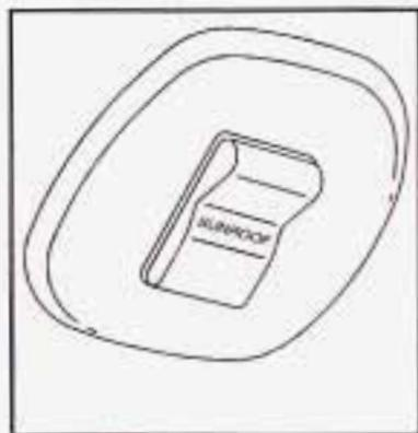
If your vehicle has a sunroof, the switch is located between the sun visors.
