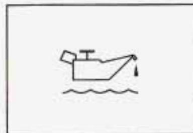
If the low engine oil level message appears on the instrument cluster, it means you need to check your engine oil level right away. For more information, see *Low Engine Oil Level Message* on page 3-43.
