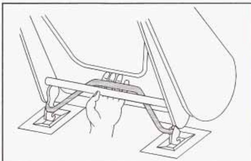
1. Squeeze the angled latch release bar toward the straight crossbar while placing the front hooks of the bench seat onto the front two floor pins.
