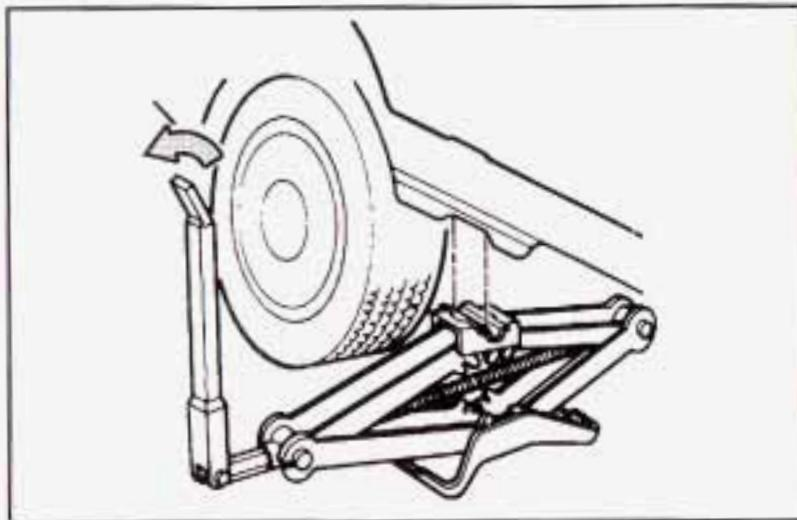
9. Lower the vehicle by attaching the folding wheel wrench to the jack and turning the wrench counterclockwise. Lower the jack completely.
