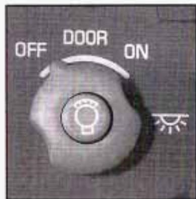
Your interior lamp control is located below the exterior lamp control.
