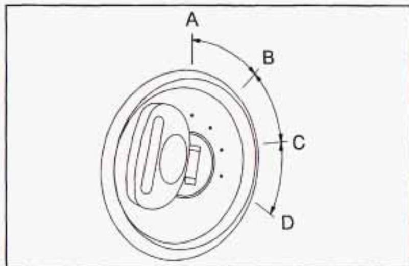
**A (OFF):** This is the only position in which you can remove the key. This position locks the steering wheel, ignition and transaxle.
