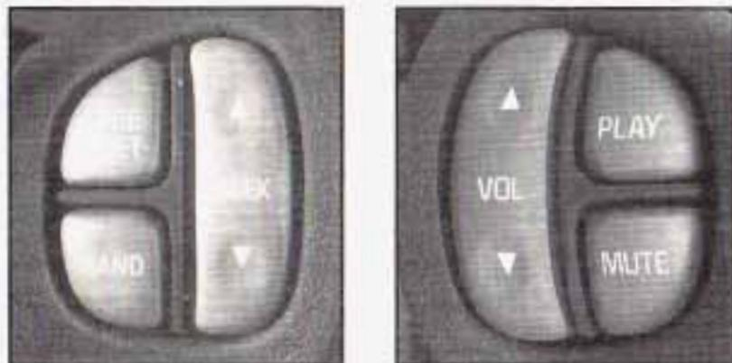
**PRESET:** Press this button to play a station you have programmed on the radio preset pushbuttons. The radio will go to a preset station, play for a few seconds, then go to the next station. Press this button again to stop scanning the preset stations. If a cassette tape is playing, press this button to play the other side of the tape.
