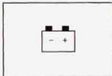
The charging system battery symbol will come on in the message center when you turn on the ignition as a check to show you it is working.
