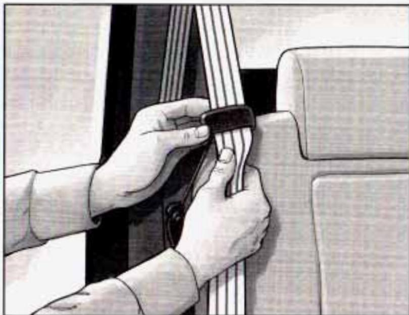
2. Place the guide over the belt and insert the two edges of the belt into the slots of the guide.
