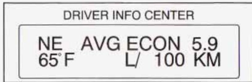
If your vehicle is equipped with the Driver Information Center (DIC), the display is located on the instrument panel cluster directly above the steering column. The DIC will show information about the vehicle and the surroundings.
