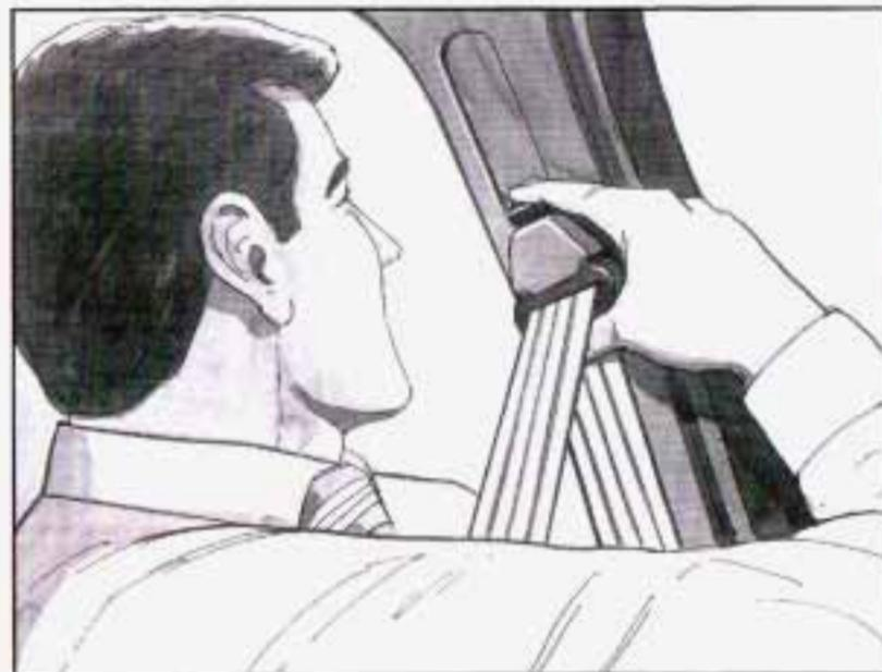
To move it down, push down on the button and move the height adjuster to the desired position.
