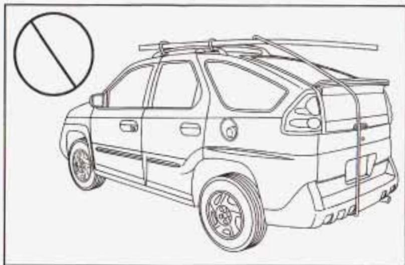
If you have the luggage carrier, you can load things on top of your vehicle. If you do load things on the top of your vehicle, you must load them on the luggage carrier crossrails. The luggage carrier has four tie-down loops on the inside of each right and left side rail. These let you secure cargo placed on the crossrails, as long as they are not wider or longer than the luggage carrier.
