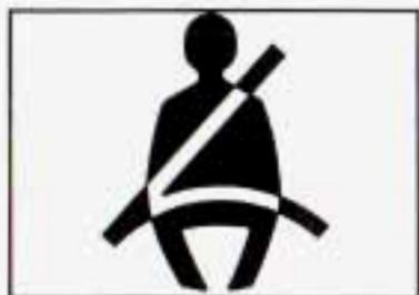
The safety belt light will also come on and stay on for several seconds. If the driver's belt is already buckled, neither the chime nor the light will come on.
