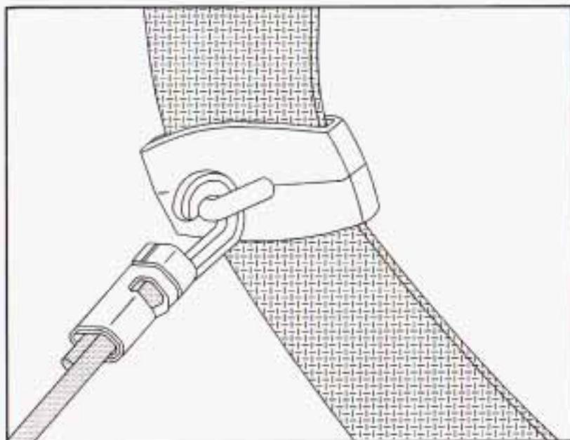
2. Attach the elastic cord to the comfort guide on the center passenger shoulder belt.
