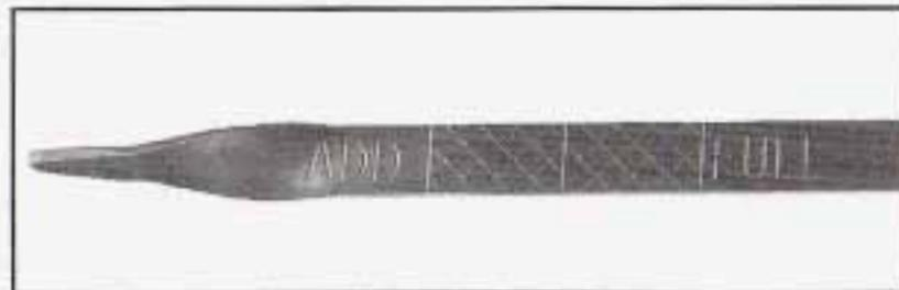
3. Check both sides of the dipstick, and read the lower level. The fluid level must be in the cross-hatched area.
