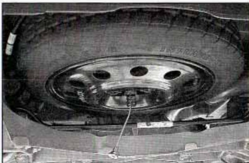
If the spare tire will not lower, the secondary latch may be engaged causing the tire not to lower. Do the following to check the cable:
