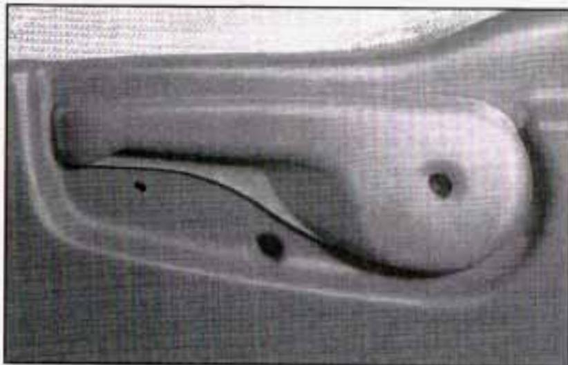
To adjust the seatback, pull up on the recliner lever located on the outboard sides of both the driver's and front passenger's seats.
