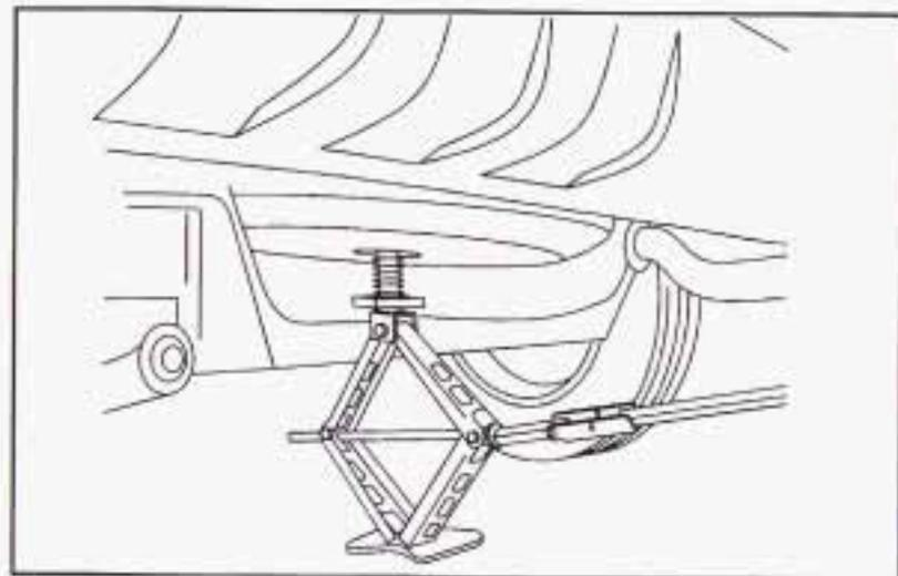
6. Lower the jack by turning the folding wrench counterclockwise. Keep lowering the jack until the spare tire is resting on the folding wrench.
