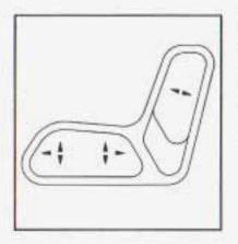
If your vehicle has this feature, the eight-way power seat controls are located on the outboard sides of both the driver's and the front passenger's seats.
