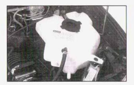
The coolant level should be at or above the FULL COLD mark. If it isn't, you may have a leak at the pressure cap or in the radiator hoses, heater hoses, radiator, water pump or somewhere else in the cooling system.
