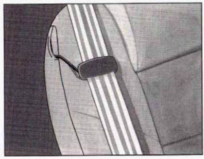
Be sure that the belt is not twisted and it lies flat. The guide must be on top of the belt.
