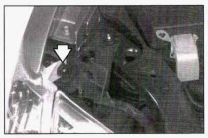
Remove the thumbscrew attaching the front turn signal/parking lamp assembly to the headlamp assembly. Pull the front turn signal/parking lamp assembly away from the vehicle.
