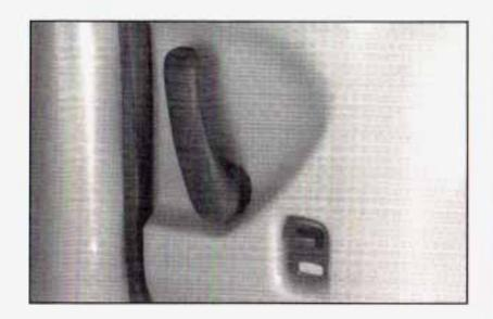
Lock either sliding door from inside the vehicle by moving the manual lever down. Unlock it by moving the lever up.
