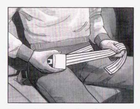
When you sit in the center position of the bench seat, you have a lap safety belt, which has no retractor. To make the belt longer, tilt the latch plate and pull it along the belt.
