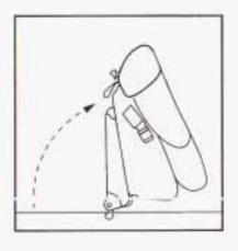
Release the rear set of hooks from the floor pins by pulling the nylon strap located at the base of the seat; hang on to the strap as the seat folds forward. To return the seat(s) to the normal position, do the following:
