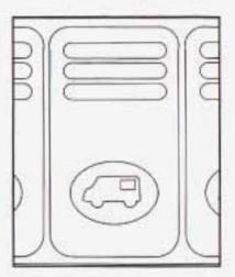
This switch, located in the overhead console switchbank, is used for opening and closing the power rear quarter windows.
