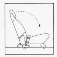
Fold the seatback flat on the seat, by either pulling on the nylon strap on the rear of the seat or lifting up on the lever located on the front of the seatback. If the seat adjusts, slide it all the way back.
