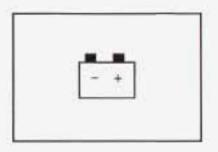
The charging system battery symbol will come on in the message center when you turn on the ignition as a check to show you it is working.
