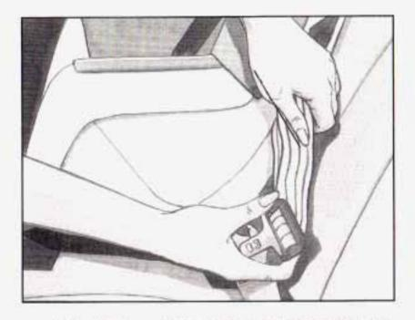
In the third row, tilt the latch plate to adjust the belt if needed.
