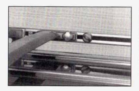
Notice: Loading cargo that weighs more than 150 lbs. (68 kg) on the luggage carrier may damage your vehicle.
