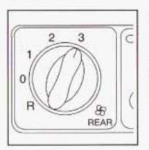
This knob is located below the main climate-control system on the instrument panel switchbank. Use this knob to adjust the fan speed for the rear-seat passengers, from the front-seating area.
