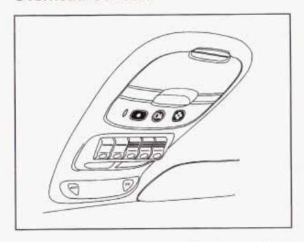
Your vehicle may have this feature. The front overhead console has reading lamps, a switchbank, storage compartments, OnStar® System buttons, Driver Information Center (DIC) and HomeLink® Transmitter buttons. For information on the features listed see each of them in the Index.
