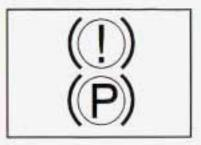
When your brake fluid falls to a low level, your brake warning light will come on. See Brake System Warning Light on page 3-44.
