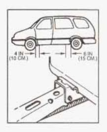
Near each wheel, there is a notch in the vehicle's body. Position the jack and raise the jack head until it fits firmly into the notch in the vehicle's frame nearest the flat tire. Do not raise the vehicle yet. Put the compact spare tire near you.
