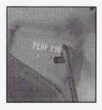
Put the end of the hood prop into the slot in the underside of the hood. Before closing the hood, be sure all the filler caps are on properly. Then follow these steps:
