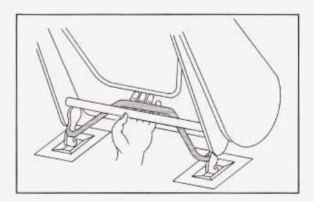
Squeeze the angled bar toward the solid crossbar while placing the front hooks of the bench seat onto the front two floor pins.
