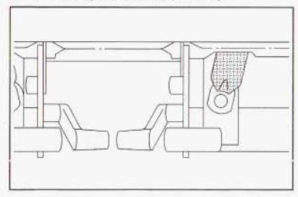
From behind the bench seat, push up the release handles at the base of the seat to release the latches from the floor pins. While holding onto the crossbar at the bottom of the seat, remove the seat by rocking it slightly toward the rear of the vehicle and then pulling it out. This should be done in one motion.
