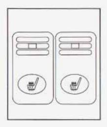
Your vehicle may have this feature. If it does, the heated seat switches are located in the instrument panel switchbank.
