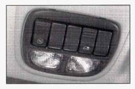
There are two reading lamps in the overhead console.
