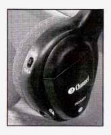
The entertainment system includes dual channel, wireless headphones. The headphones have an ON/OFF switch, a channel A/B switch and a volume control.
