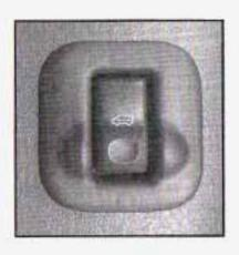
This switch is in front of the driver's or the passenger's side sliding door.
