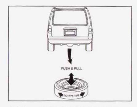
Make sure the tire is stored securely. Push, pull, and then try to rotate or turn the tire. If the tire moves, use the folding wrench to tighten the cable.
