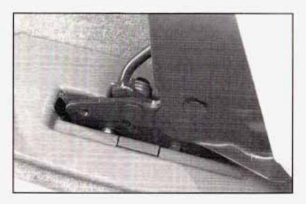
If the front latches are not attaching correctly, check that the seat is in the full rear position.
