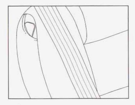
Remove the guide from its storage pocket on the side of the seatback.
