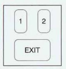
If your vehicle has this feature, the controls are located to the left of the steering column and are used to program and recall the driver's seat settings.
