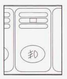
Your vehicle may have fog lamps. If it does, the fog lamps switch is located in the instrument panel switchbank. Press the fog lamp symbol on the switch to turn on the lamps. The indicator light will be lit when the fog lamps are on. Press the top part of the switch to turn them off. The indicator light will go off.
