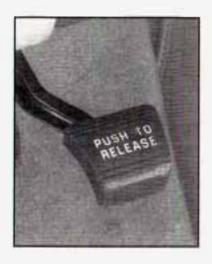
The parking brake is located on the driver's side under the instrument panel.
