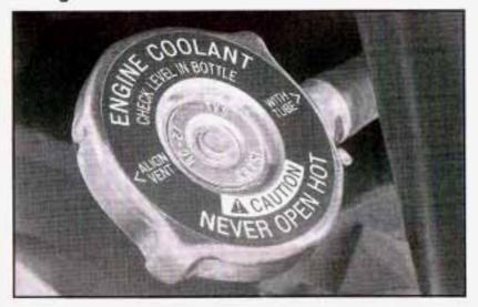
You can remove the radiator pressure cap when the cooling system, including the radiator pressure cap and upper radiator hose, is no longer hot. Turn the pressure cap slowly counterclockwise until it first stops. (Don't press down while turning the pressure cap.) If you hear a hiss, wait for that to stop. A hiss means there is still some pressure left.
