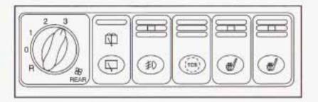
This switchbank is located in the instrument panel below the comfort controls. The switchbank may include the rear fan knob, the rear window wiper/washer, the fog lamps, the traction control and the heated seats. If your vehicle does not have some of these options, there will be a biank.
