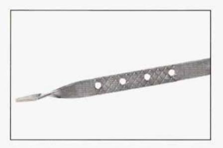
Notice: Don't add too much oil. If your engine has so much oil that the oil level gets above the cross-hatched area that shows the proper operating range, your engine could be damaged.
