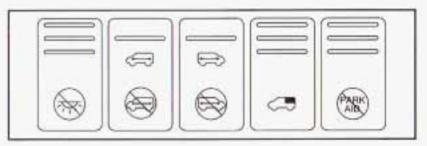
This switchbank is located in the overhead console. The switchbank may include the interior lamps override, the power sliding door(s)/override, the power rear quarter windows and the Ultrasonic Rear Parking Aid (URPA) disable switches. If your vehicle does not have some of these options, there will be a blank.
