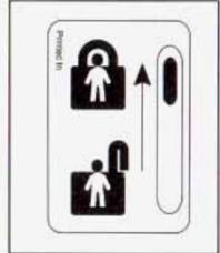
On the inside of the sliding door(s), on the front edge of the door will be a lock. Push the lever up to engage the lock.
