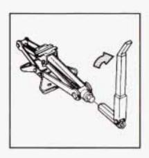
Attach the folding wrench to the jack, and turn the wrench clockwise to raise the jack head a few inches.
