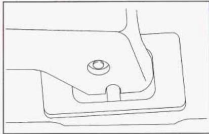
1. Hook the front latches over the front floor pins.
