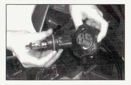
Install the new bulb through the black retainer ring and into the electrical connector. Tighten the black retainer ring in place. Push the bulb firmly enough so that the blue tabs hook over the tab on the bulb.
