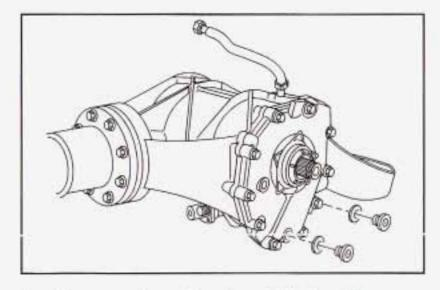
To get an accurate reading, the vehicle should be on a level surface. If the level is below the bottom of the filler plug hole, you'll need to add some lubricant. Add enough lubricant to raise the level to the bottom of the filler plug hole. A fluid loss could indicate a problem; check and have it repaired, if needed.
