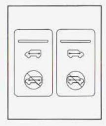
If you have the dual sliding doors, your vehicle has these switches. The left switch is for the driver's side power sliding door and the right switch is for the passenger's side sliding door. The power sliding door and the power sliding door override is one switch.
