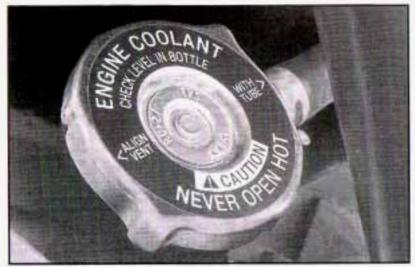
Then replace the pressure cap. At any time during this procedure if coolant begins to flow out of the filler neck, reinstall the pressure cap. Be sure the arrows on the pressure cap line up with the vent tube.
