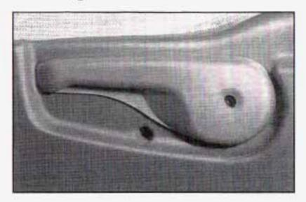
To adjust the manual seatback, pull up on the lever located on the outboard sides of both the driver's and the front passenger's seat. It is easier to recline the seat if you lean forward, taking your weight off the seatback.
