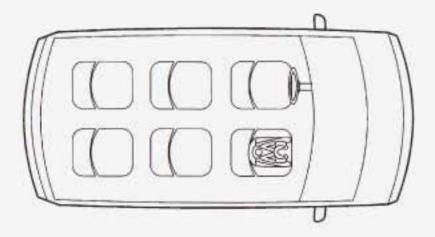
Your vehicle has a front passenger air bag. Never put a rear facing child restraint in this seat. Here's why:
