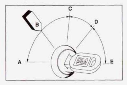
A (ACCESSORY): This is the position in which you can operate your electrical accessories. Press in the ignition switch as you turn the top of the key toward you.
