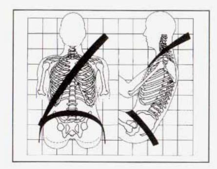
The lap part of the belt should be worn low and snug on the hips, just touching the thighs. In a crash this applies force to the strong pelvic bones. And you'd be less likely to side under the lap belt. If you slid under it, the belt would apply force at your abdomen. This could cause serious or even fatal injuries. The shoulder belt should go over the shoulder and across the chest. These parts of the body are best able to take belt restraining forces.
