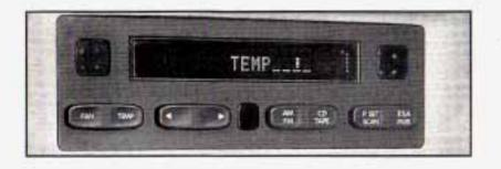
These controls are overhead, on the control panel located behind the front seats. A rear-seat passenger can use these controls to personally adjust the temperature and the fan speed for the rear-seating area.
