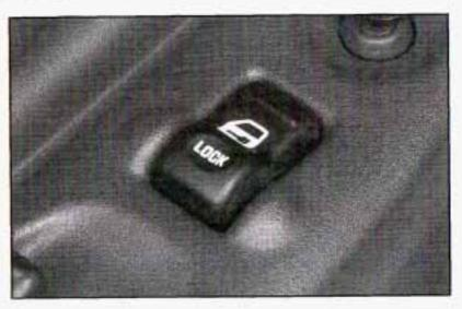
From the inside, press the front of the power door lock switch (on either front door) to unlock all doors and the liftgate. With the content theft-deterrent system, the power door lock switch will not unlock the doors until the system is disarmed. See Content Theft-Deterrent on page 2-27 for more details.
