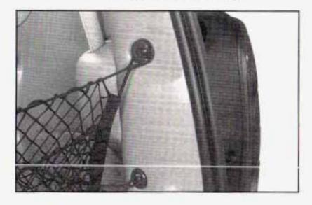
Attach the upper loops to the posts on either side of the liftgate opening. The label on the net should be in the upper left-hand corner.
