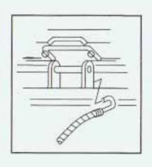
Hook the cable onto the outside portion of the liftgate hinges.
