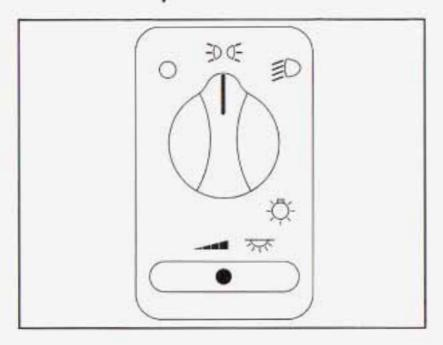
The control to the left of the steering column operates the exterior lamps.
