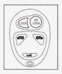
You can lock and unlock your doors and the liftgate from about 3 feet (1 m) up to 30 feet (9 m) away using the remote keyless entry transmitter supplied with your vehicle.
