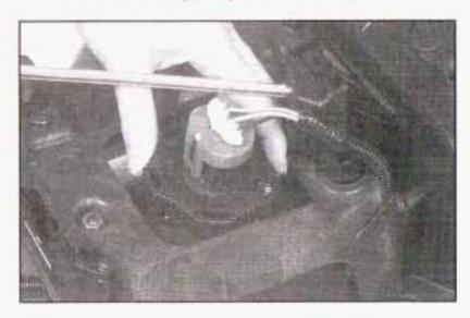
Unscrew the black retainer ring that holds the bulb assembly in place.
