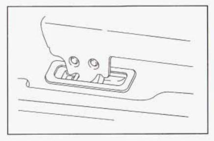
The seat can then be lifted off the front floor pins and removed from the vehicle.
