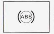
Your vehicle may have this light. If it does, the anti-lock brake system warning light should come on for a few seconds when you turn the ignition key to RUN.
