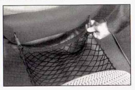
There may be a storage net that stretches between the front seats. Pull the hooks towards the passenger's seat and insert them into the holes.
