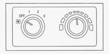
These controls are overhead, on the control panel located behind the driver's seat. A rear-seat passenger can use these controls to personally adjust the temperature and the fan speed for the rear-seating area.
