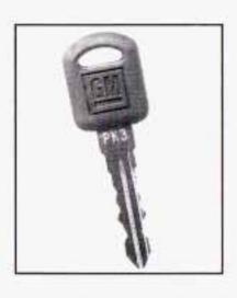
This key can be used for the ignition as well as all door locks, the liftgate lock and the storage compartments.
