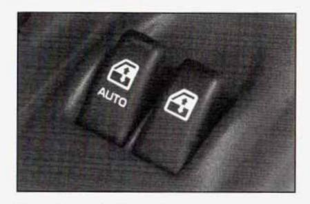
The switches on the driver's door armrest control the front windows when the ignition is in RUN, ACCESSORY or when Retained Accessory Power (RAP) is active. See "Retained Accessory Power (RAP)" under Ignition Positions on page 2-32.
