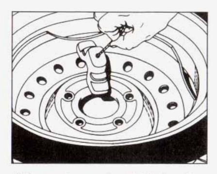
To remove the compact spare tire from the cable, tilt the retainer at the end of the cable so it can be pulled up through the wheel opening.  If your vehicle is an all-wheel-drive vehicle, after removing the compact spare tire turn the wrench clockwise to raise the cable back up.
