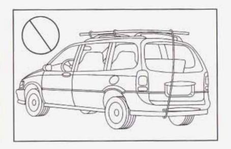
If you have the luggage carrier, you can load things on top of your vehicle. The luggage carrier has side rails attached to the roof, as well as sliding crossrails and places to use for tying things down. These let you load some things on top of your vehicle, as long as they are not wider or longer than the luggage carrier.
