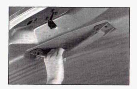
To close the liftgate, pull down on the handle, then firmly shut the liftgate. Don't drive with the liftgate open, even slightly. See Engine Exhaust on page 2-43.
