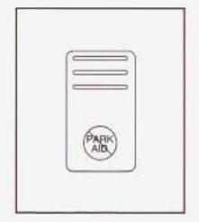
URPA can be turned off by pressing the rear park aid disable switch located in the instrument panel switchbank. When the system is disabled an indicator light will be lit on the switch. You will not see any lights on the rear display if the switch is in the off position.
