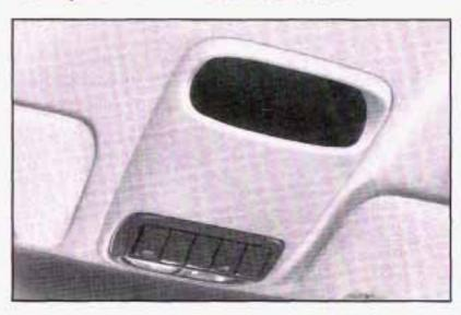
The front overhead console includes two reading lamps, a storage compartment and a switchbank.
