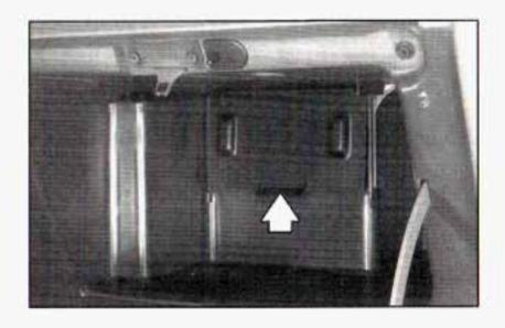
Pull the tab located on the outer access panel up and out.
