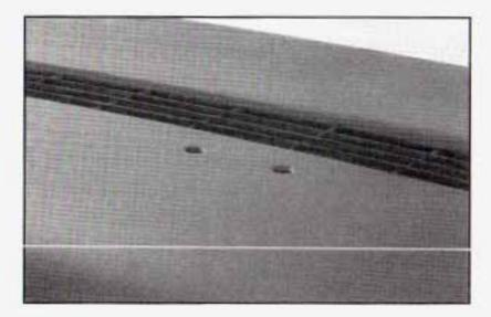
A light located on top of your instrument panel (near the center of the vehicle, next to the windshield) will flash slowly to let you know that the system has been armed.
