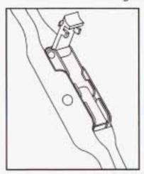
While holding the wiper arm away from the glass, push the release clip from under the blade.
