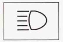
When the high beams are on, this light on the instrument panel cluster will also be on.
