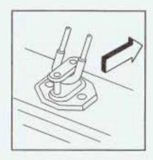
Make sure the metal tube is centered at the striker. Push the tube towards the front of the vehicle.
