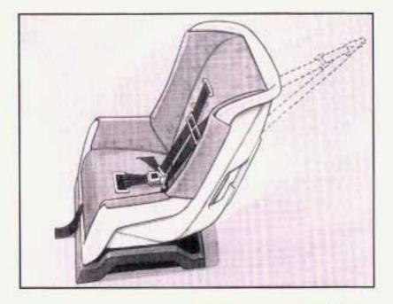
In Canada, the law requires that forward-facing child restraints have a top strap, and that the strap be anchored. In the United States, some child restraints also have a top strap. If your child restraint has a top strap, it should be anchored. Anchor the top strap to one of the following anchor points. Be sure to use an anchor point located on the same side of the vehicle as the seating position where the child restraint will be placed.
