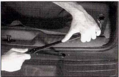
To remove the underbody-mounted spare, insert the socket end of the extension on a 45° angle downward into the hoist drive shaft hole. It is exposed when the rear gate is open and is just above the rear bumper. Be sure the socket end of the extension connects into the hoist shaft. Turn the wheel wrench counterclockwise to lower the spare tire. Keep turning the wheel wrench until the spare tire can be pulled out from under the vehicle.
