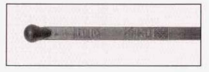
If the fluid level is in the acceptable range, push the dipstick back in all the way; then flip the handle down to lock the dipstick in place.
