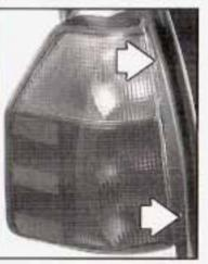
Remove the two screws from the lamp assembly. 3. Pull the assembly away from the vehicle.
