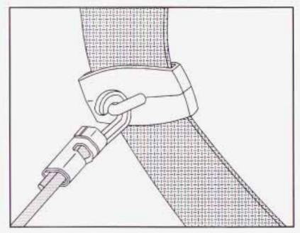
Align the sliding comfort guide, located on the shoulder belt, with the hook. Attach the hook to the loop on the sliding comfort guide.
