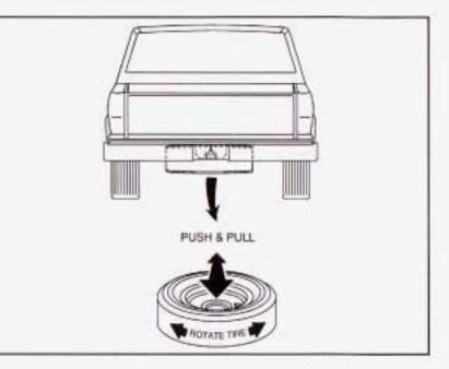
Make sure the tire is stored securely. Push, pull, and then try to rotate or turn the tire. If the tire moves, use the wheel wrench to tighten the cable. Return the jack, wheel wrench and wheel blocks to the proper location in the vehicle. Roll up the instruction label and return it to the slot in the tool kit.
