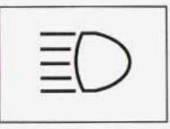
When the high beams are on, this indicator light on the instrument panel cluster will also be on.
