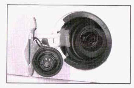
While refueling, hang the fuel cap by the tether using the hook located on the inside of the filler door.
