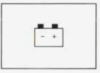
The charging system light will come on briefly when you turn on the ignition, but the engine is not running, as a check to show you it is working.
