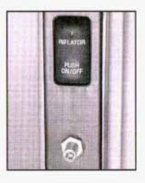
The air inflator is often located in the rear compartment on the passenger's side of the vehicle behind an access cover.
