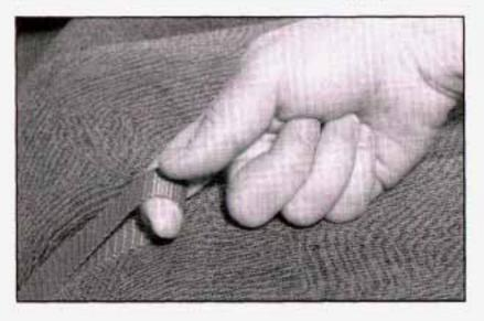
Pull up on the loop located where the seat cushion meets the seatback to fold the seat cushion up and out of the way. This will allow the seatback to fold flat and increase the cargo area.
