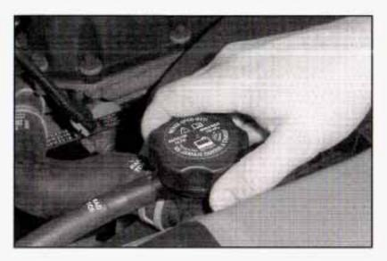
You can remove the radiator pressure cap when the cooling system, including the radiator pressure cap and upper radiator hose, is no longer hot. Turn the pressure cap slowly counterclockwise about one full turn.
