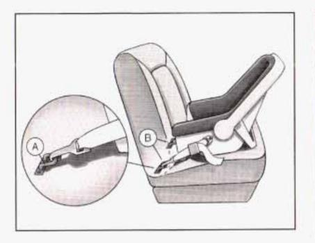
With this system, use the LATCH system instead of the vehicle's safety belts to secure a child restraint. See Securing a Child Restraint in a Rear Outside Seat Position on page 1-44.
