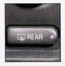
Press this button to turn the rear window defogger on or off.
