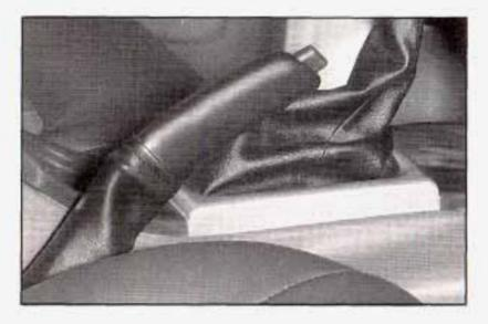
To release the parking brake, hold the regular brake pedal down. Pull the parking brake lever up until you can press in the button at the end of the lever. Hold the button in as you move the parking brake lever all the way down.
