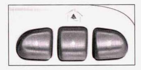
HomeLink<sup>®</sup>, a combined universal transmitter and receiver, provides a way to replace up to three hand-held transmitters used to activate devices such as gate operators, garage door openers, entry door locks, security systems and home lighting. Additional HomeLink<sup>®</sup> information can be found on the internet at www.homelink.com or by calling 1-800-355-3515.
