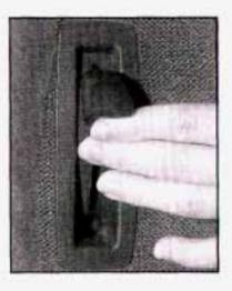
The rear seatback levers are located on the outboard side of the rear seatbacks.
