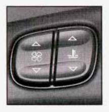
(Fan): Press the up or down arrow on this switch to increase or decrease the fan speed.
