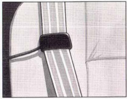
Be sure that the belt is not twisted and it lies flat. The elastic cord must be under the belt and the guide on top.
