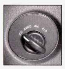
If your vehicle is equipped with the automatic transfer case, the transfer case knob is located to the right of the steering wheel on the instrument panel. Use this knob to shift into and out of four-wheel drive. 2HI (Two-Wheel High): This setting is for driving in most street and highway situations. Your front axle is not engaged in two-wheel drive. It also provides the best fuel economy.
