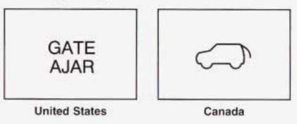
If this light comes on, your liftgate or liftglass is ajar. Try closing the liftgate or liftglass again. Never drive with the liftgate or liftglass even partially open.
