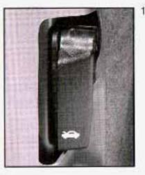
To open the hood, first pull the handle located inside the vehicle on the lower driver's side of the instrument panel.
