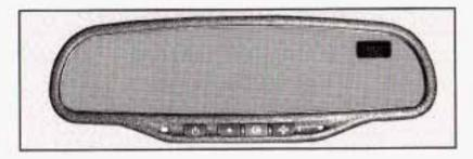
Your vehicle may have an automatic-dimming rearview mirror with a compass and the OnStar<sup>®</sup> system.
