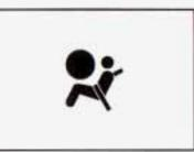
There is an air bag readiness light on the instrument panel cluster, which shows the air bag symbol.
