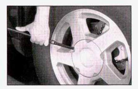
Use the chisel end of the wheel wrench to pry off the center cap.
