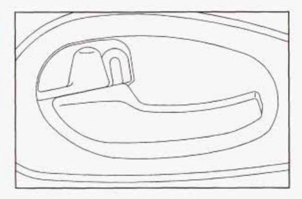
You can lock or unlock the door from the inside by sliding the manual lever forward or rearward. When the door is unlocked, you can see a red area on the lever.
