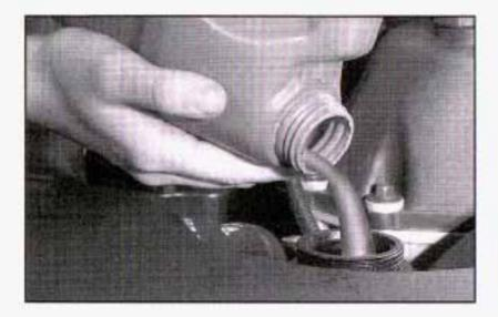
Fill the radiator with the proper DEX-COOL<sup>®</sup> coolant mixture, up to the base of the filler neck. See Engine Coolant on page 5-24 for more information about the proper coolant mixture.
