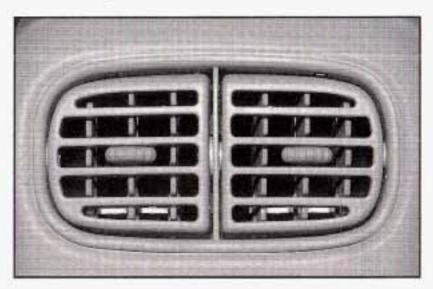
Your vehicle may have rear seat outlets that can be used to adjust the airflow toward either seating area, the floor or upward. Move the control in the center of each outlet in any direction to direct airflow.
