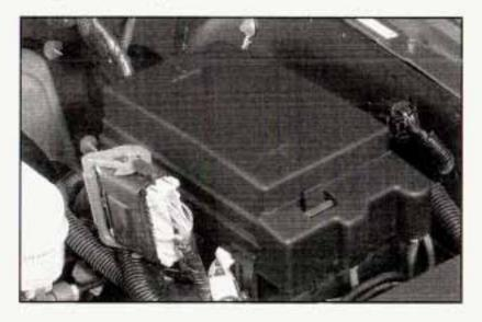
The fuse block is located under the hood in the engine compartment on the driver's side of the vehicle. See Engine Compartment Overview on page 5-12 for more information on location.
