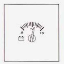
When your engine is not running, but the ignition is on (in RUN), this gage shows your battery's state of charge in DC volts.
