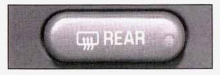
Press this button to turn the rear window defogger on or off. An indicator light in the button will come on to let you know that the rear window defogger is active. The rear window defogger will automatically turn off approximately ten minutes after the button is pressed.
