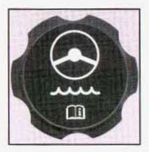
The power steering fluid reservoir is located in the engine compartment. It is on the passenger's side of vehicles with the L6 engine and is on the driver's side of vehicles with the V8 engine.
