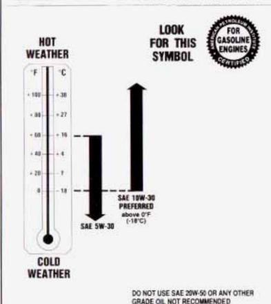
Notice: Use only engine oil with the American Petroleum Institute Certified For Gasoline Engines starburst symbol. Failure to use the recommended oil can result in engine damage not covered by your warranty.
