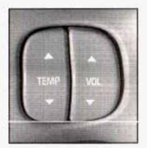
If your vehicle has this feature, you can control the temperature function by using the switch located on your steering wheel.
