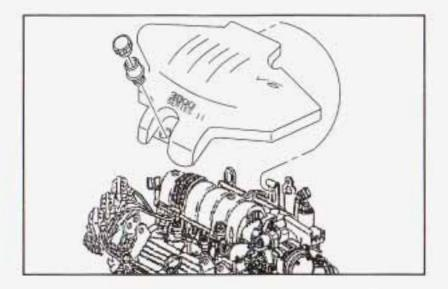
Clean the area around the engine oil fill tube and cap before removing. Twist the oil fill tube, with cap attached, counterclockwise and remove it.
