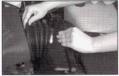
Remove the air intake hose that snaps over the throttle body by pulling the hose upward and away from the throttle body. As you are detaching the hose, remove the housing cover by pulling upward and rearward.
