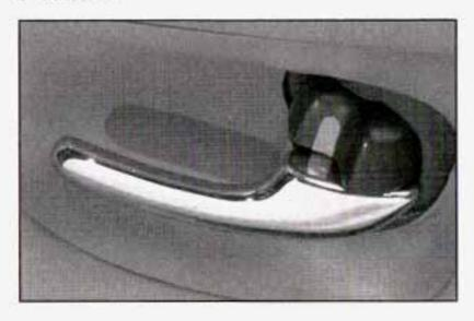
To lock or unlock the doors from the inside, move the manual lock on the door handle forward or rearward.
