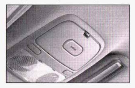
If your vehicle has this feature, the garage door opener storage area is located in the headliner near the front reading lamps. To install your garage door opener, do the following:
