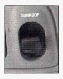
The switch for the sunroof is located on the headliner between the sun visors
