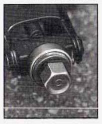
The jack has a bolt at the end. Attach the wheel wrench to the bolt to create a jack handle. Turn the wheel wrench counterclockwise to lower the jack head until it fits under the vehicle.
