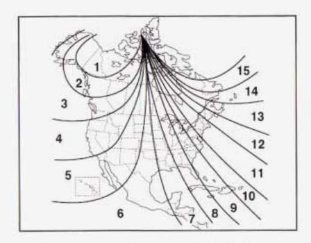
Once a zone number appears in the display, press the COMPASS button (or the on/off button for mirrors equipped with OnStar® controls) quickly until the correct zone number appears in the display. Stop pressing the button and the mirror will return to normal operation. If C appears in the compass window, the compass may need calibration. See "Compass Calibration" explained previously.
