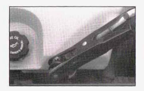
Connect the other end of the negative (-) cable at least 18 inches (45 cm) away from the dead battery, but not near engine parts that move. The electrical connection is just as good there, and the chance of sparks getting back to the battery is much less.
