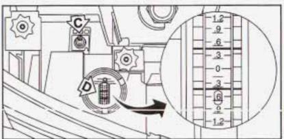
Turn the vertical aiming screw (C) until the level bubble (D) is lined up with zero.
