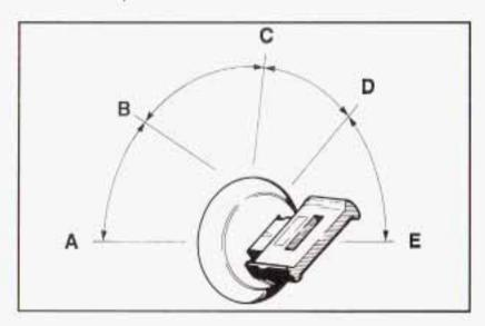
A (ACCESSORY): In this position you can operate your electrical accessories. Press in the ignition switch as you turn the top of it toward you.
