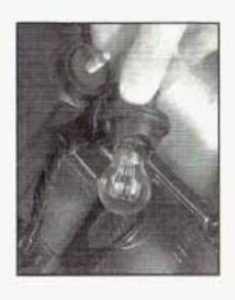
Once the socket has been removed, pull the bulb straight out to remove it from the socket.
