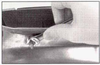
From inside the trunk compartment, remove the nuts from the studs.
