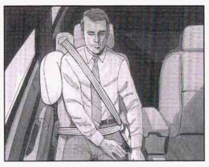
The right front passenger's side impact air bag is in the side of the passenger's seatback closest to the door.
