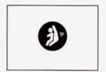
To assist you in locating the lower anchors for this child restraint system, each seating position with the LATCH system will have a label sewn into the seatback at each anchor point.
