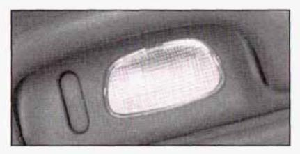
To turn on a rear reading lamp, press the button above that rear door. To turn off the reading lamp, press the button again.
