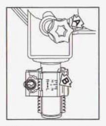
Turn the horizontal aiming screw (A) until the indicator (B) is lined up with zero.
