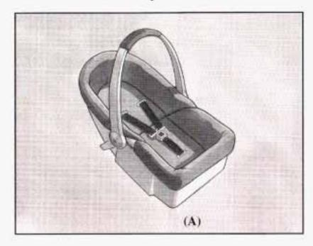
An infant car bed (A), a special bed made for use in a motor vehicle, is an infant restraint system designed to restrain or position a child on a continuous flat surface. Make sure that the infant's head rests toward the center of the vehicle.
