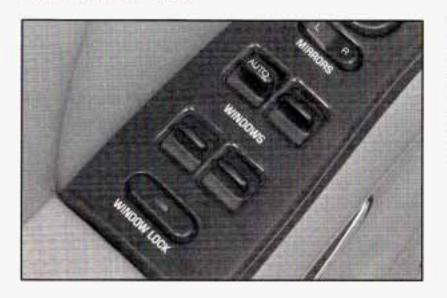
Use the switches on the driver's door armrest to control each of the windows while the ignition is on or while Retained Accessory Power (RAP) is active. See "Retained Accessory Power (RAP)" under Ignition Positions on page 2-25 for more information. In addition, each passenger door has a window switch.
