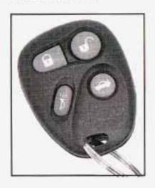
door will unlock when this button is pressed. If the unlock button is pressed again within five seconds, all the doors will unlock.
