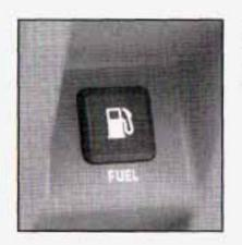
The release button for the fuel door is located to the left of the steering column.
