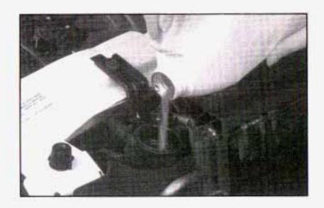
5. Fill the radiator with the proper DEX-COOL<sup>®</sup> coolant mixture, up to the base of the filler neck. See Engine Coolant on page 5-26 for more information about the proper coolant mixture.
