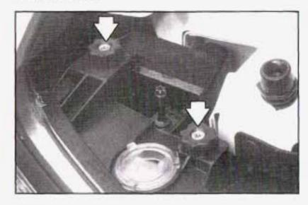
Each headlamp is attached by thumb screws.
