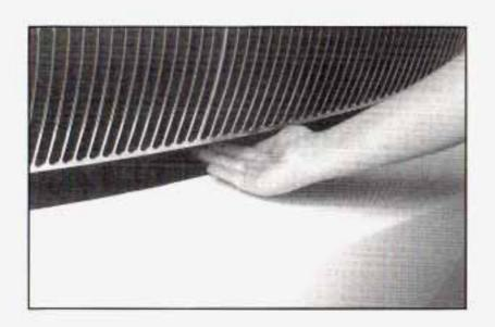
Then go to the front of the vehicle and locate the secondary hood release lever under the front edge of the grille.
