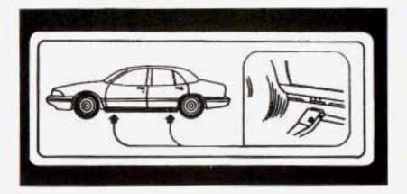
4. Near each wheel well is a notch in the plastic trim panel to position the jack head. You'll find the word JACK and an arrow stamped into the plastic near each notch. Position the jack under the vehicle and raise the jack head until it fits firmly against the sheet metal next to the word JACK. Do not raise the vehicle yet. Put the compact spare tire near you.
