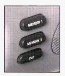
If your vehicle has this feature, the controls are located on the driver's door panel, and are used to program and recall memory settings for the driver's seating, outside mirror positions and climate controls. See Climate Controls Personalization on page 3-32 for more information.
