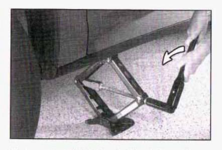
Lower the vehicle by turning the wheel wrench counterclockwise. Lower the jack completely.
