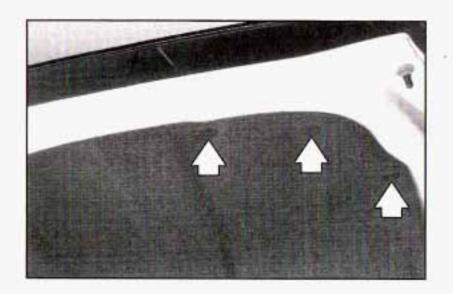
Remove the six fasteners along the top of the trunk lid (three on each side), holding the trunk trim in place.
