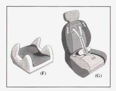
A booster seat (F-G) is a child restraint designed to improve the fit of the vehicle's safety belt system. Some booster seats have a shoulder belt positioner, and some high-back booster seats have a five-point hamess. A booster seat can also help a child to see out the window.
