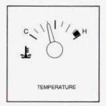
This gage measures the temperature of the vehicle's engine. If the pointer moves into the shaded area, the engine is too hot. A temperature indicator light will turn on and a chime will sound.
