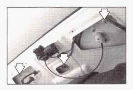
Pull the trunk trim back to expose the three remaining nuts holding the taillamp assembly in place. Remove the protective vinyl caps from the studs.
