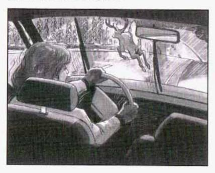
As you brake, your computer keeps receiving updates on wheel speed and controls braking pressure accordingly. Remember: Anti-lock doesn't change the time you need to get your foot up to the brake pedal or always decrease stopping distance. If you get too close to the vehicle in front of you, you won't have time to apply your brakes if that vehicle suddenly slows or stops. Always leave enough room up ahead to stop, even though you have anti-lock brakes.
