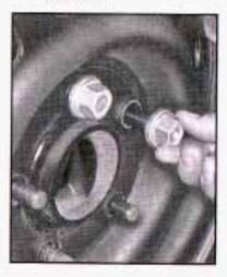
Then reinstall the wheel nuts with the rounded end of the nuts toward the wheel. Tighten each nut by hand until the wheel is held against the hub.
