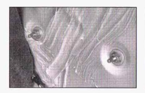
Beneath the trim panel are three nuts that secure the taillamp assembly. Remove the nuts only from the side you want to access. The turn signal and a stoplamp can now be accessed.
