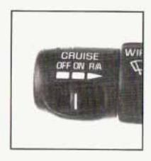
Move the cruise control switch to ON.
