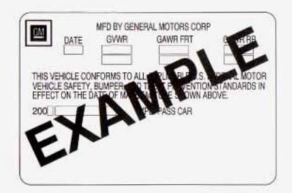
The other label is the Certification Label, found on the rear edge of the driver's door. It tells you the gross weight capacity of your vehicle, called the Gross Vehicle Weight Rating (GVWR). The GVWR includes the weight of the vehicle, all occupants, fuel and cargo. Never exceed the GVWR for your vehicle, or the Gross Axle Weight Rating (GAWR) for either the front or rear axle. And, if you do have a heavy load, you should spread it out. Don't carry more than 176 lbs (80 kg) in your trunk.
