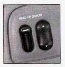
The HUD controls are located in the overhead console.
