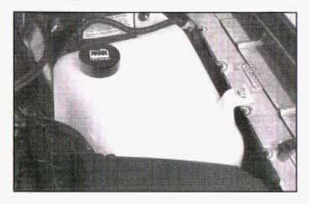
The coolant recovery tank is located in the engine compartment on the driver's side of the vehicle. See Engine Compartment Overview on page 5-12 for more information on location. The vehicle must be on a level surface. When your engine is cold, the coolant level should be at FULL COLD or a little higher. When your engine is warm, the level should be up to FULL HOT or a little higher.
