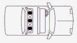
Your vehicle has the LATCH system. You'll find anchors (A) in all three rear seat positions.
