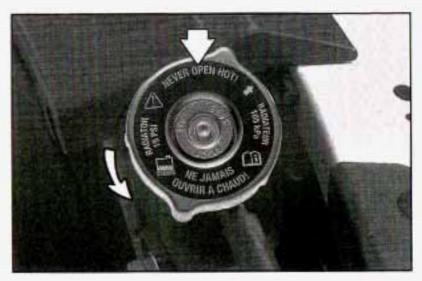
Then keep turning the pressure cap, but now push down as you turn it. Remove the pressure cap. Remove the 3800 Series II V6 engine cover shield to access the bleed valve.
