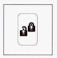
Your vehicle is equipped with rear door security locks that prevent passengers from opening the rear doors of your vehicle from the inside
