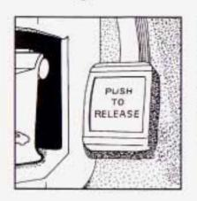
This vehicle has a PUSH TO RELEASE parking brake pedal. To set the parking brake, hold the regular brake pedal down with your right foot. Push down the parking brake pedal with your left foot.
