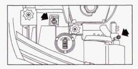
The headlamp aiming device is under the hood, directly behind the headlamps.
