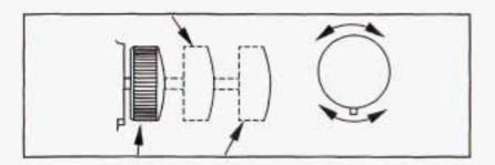
OFF: Pushing the exterior lamps control all the way in turns off all lamps and lights.
