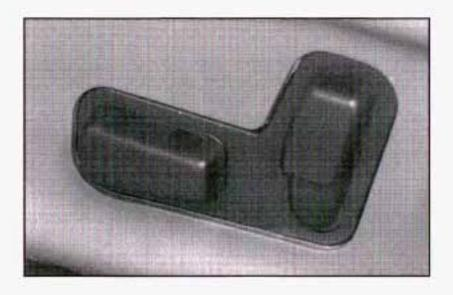
The power seat controls are located on the outboard sides of both the driver's and front passenger's seats.
