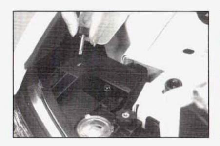
Remove the thumb screws by turning them counterclockwise.
