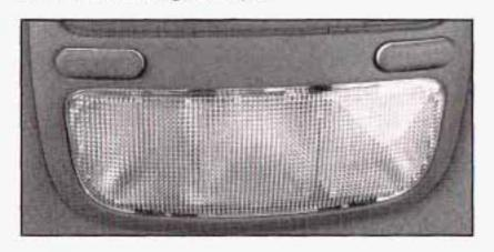
The front reading lamps, located on the headliner, and the interior courtesy lamps will come on when you open a door. They will turn off when you turn on the ignition.
