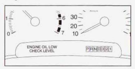
If the DIC message, ENGINE OIL LOW — CHECK LEVEL appears on the instrument cluster, it means you need to check your engine oil level right away. For more information, see *Driver Information Center (DIC) on page 3-48*.
