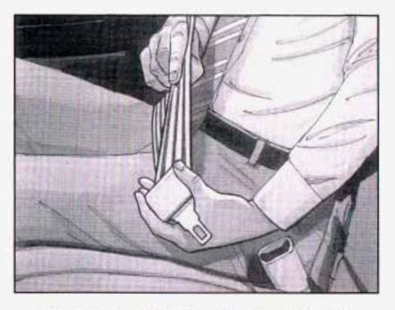
If the belt stops before it reaches the buckle, tilt the latch plate and keep pulling until you can buckle it. Pull up on the latch plate to make sure it is secure. If the belt is not long enough, see Safety Belt Extender on page 1-26.
