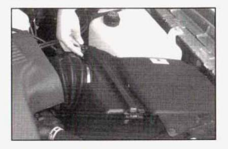
Remove the wing nuts on the engine air cleaner/filter housing cover.
