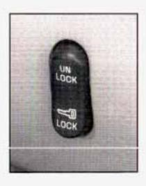
With power door locks, you can lock or unlock all doors on your vehicle using either the driver's or the front passenger's power door lock switch.
