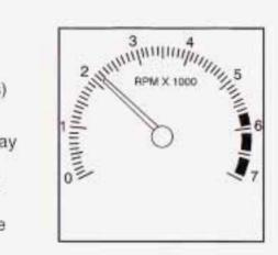
The tachometer tells you how fast the engine is running. It displays engine speed in thousands of revolutions per minute (rpm).
