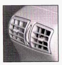
Use the thumbwheel located between the rear passenger outlets to open and close the outlets. Adjust the direction of the airflow from side to side with the levers in the center of each rear outlet.
