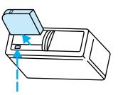
Make sure only one disc is inserted in each slot, and make sure the discs are inserted with the label surface upward. You may insert up to six CDs.
