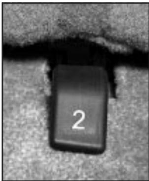
3. To unlatch the rear of the seat from the floor, pull up on the release lever labeled 2 at the rear of the seat, and lift the rear of the seat up from the floor.
