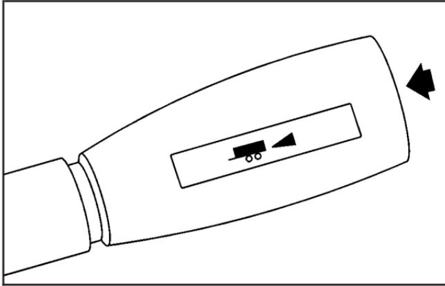
Your vehicle is equipped with a Tow/Haul mode. The button is located on the end of the column shift lever. You can use this feature to assist when towing or hauling a heavy load. See “Tow/Haul Mode” under *Towing a Trailer* on page 4-51 for more information.
