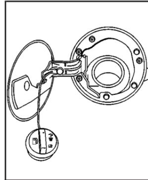
While refueling, hang the fuel cap by the tether using the hook located on the inside of the filler door.
