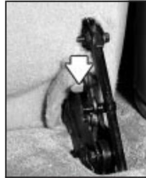
1. Pull the lever on the support rod bracket until it unlatches from the seat bracket.
