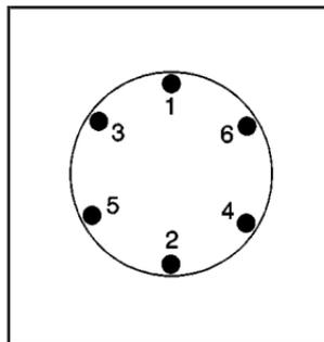
8. Tighten the nuts firmly in a crisscross sequence as shown by turning the wheel wrench clockwise.
