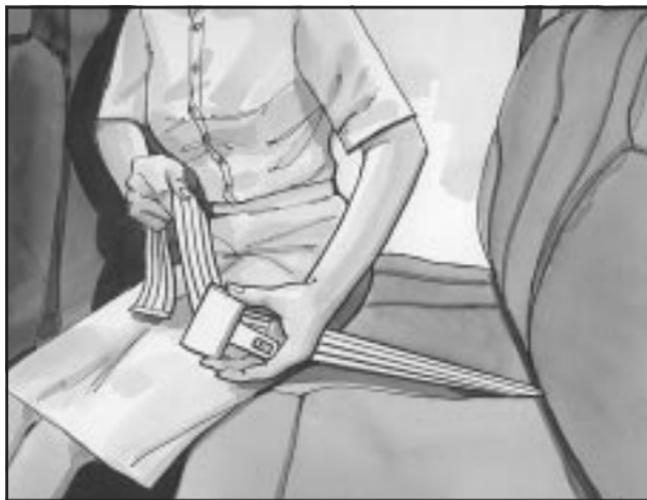
1. Make the belt as long as possible by tilting the latch plate and pulling it along the belt.
