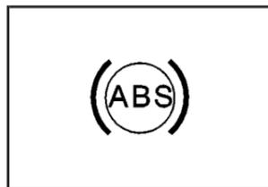
With the anti-lock brake system, this light will come on when you start your engine and may stay on for several seconds.
