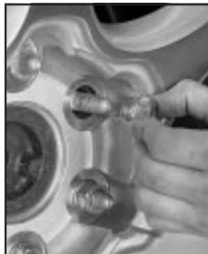
6. After mounting the spare, put the wheel nuts back on with the rounded end of the nuts toward the wheel. Tighten each wheel nut by hand. Then use the wheel wrench to tighten the nuts until the wheel is held against the hub.
