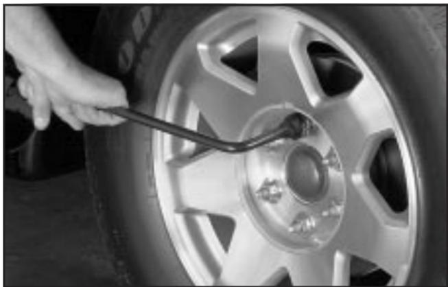
2. Use the wheel wrench to loosen all the wheel nuts. Turn the wheel wrench counterclockwise to loosen the wheel nuts. Don't remove the wheel nuts yet.
