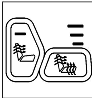
The buttons used to control this feature are located on the front doors. The engine must be running for the heated seat feature to work.
