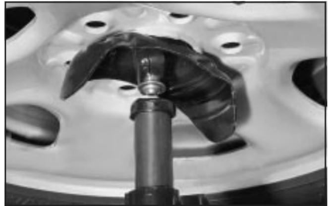
8. Attach the jack handle, extension, and wheel wrench to the jack and place it (with the wheel blocks) under the vehicle towards the front of the rear bumper. Position the center lift point of the jack under the center of the spare tire.
