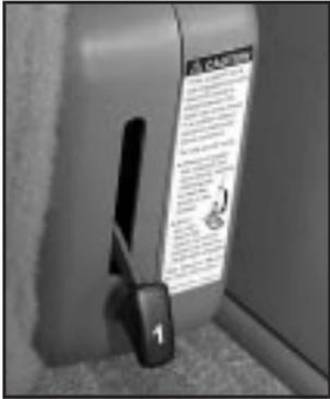
1. To return the seatback to an upright position, pull up on the release lever labeled 1 and then pull up on the seatback until it locks into the upright position.
