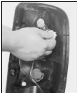
4. Pull the bulb straight out from the socket.
