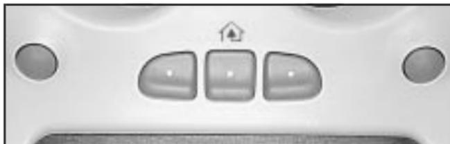
HomeLink® a combined universal transmitter and receiver, provides a way to replace up to three hand-held transmitters used to activate devices such as gate operators, garage door openers, entry door locks, security systems and home lighting. Additional HomeLink® information can be found on the internet at [www.homelink.com](http://www.homelink.com) or by calling 1-800-355-3515.
