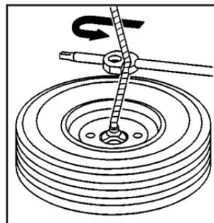
5. The wheel wrench has a hook that allows you to pull the hoist cable towards you to assist in reaching the spare tire.
