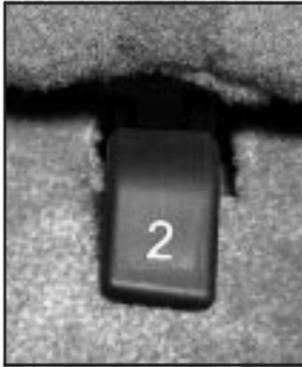
2. Unlatch the seat from the floor by pulling up on the lever labeled 2 located on the rear of the seat.
