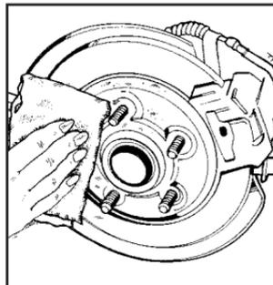
5. Remove any rust or dirt from the wheel bolts, mounting surfaces and spare wheel.
