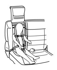
7. Insert the left and right safety belt tongues into the left and right slots of the crotch buckle. Verify that the indicator window on each tongue is green to ensure proper safety belt connections.
