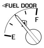
The FUEL DOOR icon and arrow indicates which side of the vehicle the fuel filler door is located.
