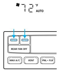
For continuous maximum cooling, push the blue button until 16°C (60°F) is shown in the display window. The EATC will continue maximum cooling (disregarding the displayed temperature) until a warmer temperature is selected by pressing the red button.
