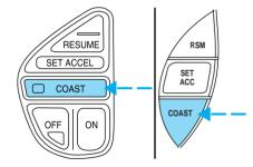
Depress the brake pedal. When the desired vehicle speed is reached, press SET ACC/SET ACCEL.
