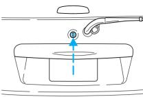
The liftgate door and window should be closed before driving your vehicle. If not, possible damage may occur to the liftgate door lift cylinders and attaching hardware.
