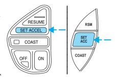
You can accelerate with the accelerator pedal at any time during speed control usage. Releasing the accelerator pedal will return your vehicle to the previously programmed set speed.
