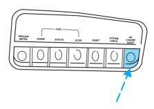
that percentage instead of 100%.) This reset procedure should be performed only after an oil change to ensure accurate oil life indications.
