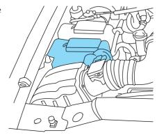
If the engine coolant has not been checked for a long period of time, the engine coolant reservoir may eventually empty. If this occurs, add engine coolant to the coolant reservoir. For more information on engine coolant maintenance, refer to *Adding engine coolant* in this chapter.
