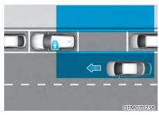
After the vehicle stops, when an approaching vehicle from the rear area is detected as soon as a passenger opens a door, Safe Exit Assist will warn the driver with a warning message and an audible warning to help prevent a collision.
