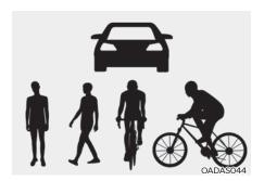
The illustration above shows the image the front view camera is capable of detecting as a vehicle, pedestrian and cyclist.
