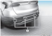
[1]: Front ultrasonic sensors,[2]: Rear ultrasonic sensors
