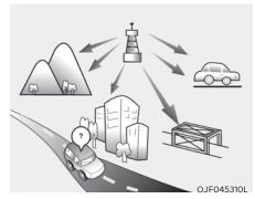
FM broadcasts are transmitted at high frequencies and do not bend to follow the earth's surface. Because of this, FM broadcasts generally begin to fade at short distances from the station. Also, FM signals are easily affected by buildings, mountains, or other obstructions. These can result in certain listening conditions which might lead you to believe a problem exists with your radio.
