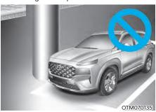
Remote Smart Parking Assist performance may reduce when there is a pillar or pillar surrounded by objects such as a fire extinguisher near the parking space.  Parking in a parking space with a vehicle on one side only
