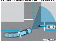
Junction Turning function will help avoid a collision with an oncoming vehicle in an adjacent lane when turning left at a crossroad with the turn signal on by applying emergency braking.
