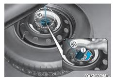
6. Draw out the retainer guide (1) the through the center hole of spare tire.
