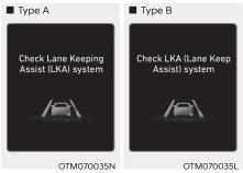
When Lane Keeping Assist is not working properly, the 'Check Lane Keeping Assist (LKA) system' (or 'Check LKA (Lane Keeping Assist) system') warning message will appear and the yellow indicator light will illuminate on the cluster. If this occurs, we recommend that the system be inspected by an authorized HYUNDAI dealer.
