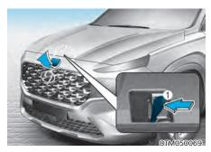
Go to the front of the vehicle, raise the hood slightly, push up the secondary latch (1) inside of the hood center and lift the hood.
