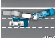
When changing lanes by detecting the lane ahead, if the system judges that there is a collision risk with an approaching vehicle in the blind spot, the system will help avoid a collision by applying the brake.
