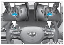
The paddle shifter is available when the shift button is in the D (Drive) position or the manual shift mode.
