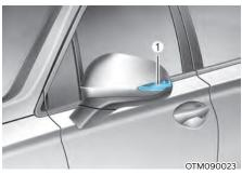
If the LED lamp (1) does not operate, we recommend that the system be inspected by an authorized HYUNDAI dealer.
