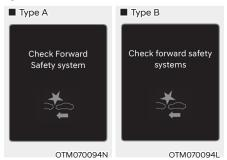
When Forward Collision-Avoidance Assist is not working properly, the 'Check Forward Safety system(s)' warning message will appear, and the 🛬 and marning lights will illuminate on the cluster. We recommend that the system be inspected by an authorized HYUNDAI dealer.
