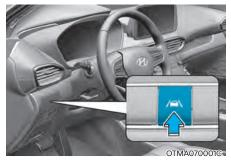
With the engine on, press and hold the Lane Safety button located on the instrument panel to turn on Lane Keeping Assist. The white Assist. The will illuminate on the cluster.
