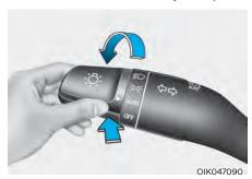
High Beam Assist will automatically adjust the headlamp range (switches between high beam and low beam) depending on the brightness of detected vehicles and certain road conditions.
