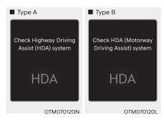
When Highway Driving Assist or Highway Lane Change function is not working properly, the 'Check Highway Driving Assist (HDA) system' (or 'Check HDA (Motorway Driving Assist) system') warning message will appear, and the A warning light will illuminate on the cluster. We recommend that the system be inspected by an authorized HYUNDAI dealer.
