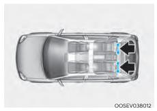
LATCH anchors have been provided in the left and right outboard rear seating positions. Their locations are shown in the illustration. There are not LATCH anchors provided for the center rear seating position.
