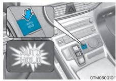
With the driver's door, engine hood and liftgate (vehicle equipped with shift button) closed, then press the AUTO HOLD switch. The white AUTO HOLD indicator will come on and the system will be in the standby position.
