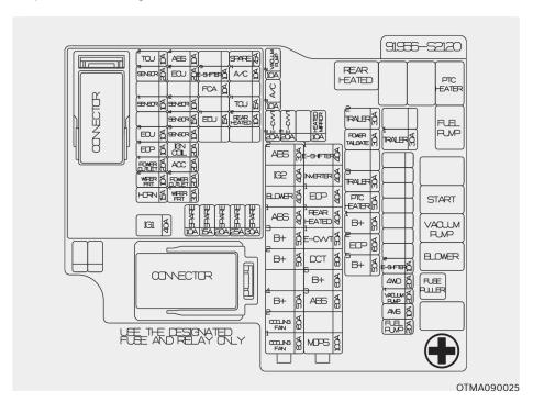
Engine compartment fuse panel (Engine room junction block)
