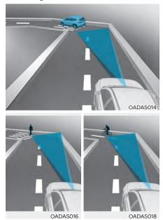
Forward Collision-Avoidance Assist may not detect other vehicles, pedestrians or cyclists in front of you on curved roads adversely affecting the performance of the sensors. This may result in no warning or braking assist when necessary.
