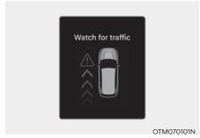
Collision warning when exiting vehicle
