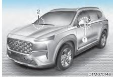
[1], [2]: SVM-side view camera (camera located at bottom of the mirror)
