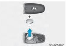
If the Smart Key is not working properly, try replacing the battery with a new one. Remove the smart key cover by turning the screwdriver clockwise by inserting the screwdriver (-) into the hole.
