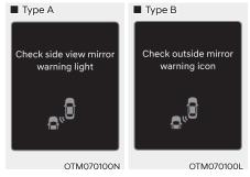
When the side view mirror warning light is not working properly, the 'Check side view mirror warning light' (or 'Check outside mirror warning icon') warning message will appear on the cluster. We recommend that the system be inspected by an authorized HYUNDAI dealer.
