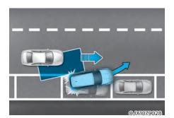
When you are driving forward out of a parking space, if the system judges that there is a collision risk with an approaching vehicle in the blind spot, the system will help avoid a collision by applying the brake.
