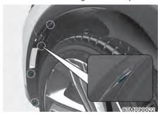
2. Remove wheel guard clips (under the front bumper: 4 pieces).
