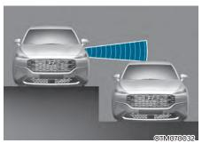
Blind-Spot Safety system may not operate properly when driving where the heights of the lanes are different. The system may not detect the vehicle on a road with different lane heights (underpass joining section, grade separated intersections, etc.). Always pay attention to road and driving conditions while driving.
