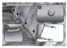
[A] : Lower Anchor Position Indicator (Type A- ( ,Type B- ),
