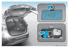
Your vehicle is equipped with the emergency liftgate safety release lever located on the bottom of the liftgate inside the vehicle.
