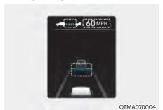
If you want to speed up temporarily when Smart Cruise Control is on, depress the accelerator pedal. While the speed is increasing, the set speed, distance level and target distance will blink on the cluster.
