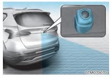
The rear view camera is used as a detecting sensor to detect pedestrians. If the camera lens is covered with foreign material, such as snow or rain, it may adversely affect camera performance and Reverse Parking Collision-Avoidance Assist may not operate normally. Always keep the camera lens clean.
