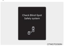
When Blind-Spot Safety system is not working properly, the 'Check Blind-Spot Safety system(s)' warning message will appear on the cluster, and the system will turn off automatically or the system will be limited. We recommend that the system be inspected by an authorized HYUNDAI dealer.
