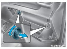
2. Remove the stoppers on both sides to allow the glove box to hang freely on the hinges.
