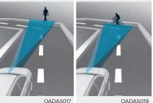
Forward Collision-Avoidance Assist may detect a vehicle, pedestrian or cyclist in the next lane or outside the lane when driving on a curved road.
