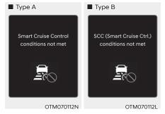
If the Driving Assist button, + switch, - switch or [] switch is pushed when the system's operating conditions are not satisfied, the 'Smart Cruise Control conditions not met' (or SCC (Smart Cruise Ctrl. conditions not met') will appear on the cluster, and an audible warning will sound.
