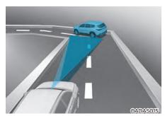
Your vehicle speed can be reduced due to a vehicle in the adjacent lane. Apply the accelerator pedal and select the appropriate set speed. Check to be sure that the road conditions permit safe operation of the Smart Cruise Control.
