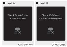
When Smart Cruise Control is not working properly, the 'Check Smart Cruise Control system' (or 'Check SCC (Smart Cruise Control) system') warning message will appear, and the \(\triangle \) warning light will illuminate on the cluster. We recommend that the system be inspected by an authorized HYUNDAI dealer.
