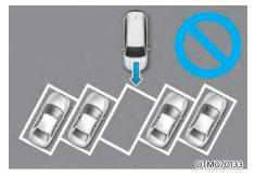
Remote Smart Parking Assist does not provide diagonal parking. Even if your vehicle was able to enter the parking space, do not use the system because the system cannot operate normally.
