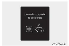
When Highway Driving Assist is operating, your vehicle will stop if the vehicle ahead of you stops. Also, if the vehicle ahead of you starts moving within 30 seconds after the stop, your vehicle will start as well. In addition, after the vehicle has stopped and 30 seconds have passed, the 'Use switch or pedal to accelerate' message will appear on the cluster. Depress the accelerator pedal or push the + switch, - switch or II'D switch to start driving.
