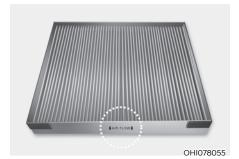
Install a new cabin air filter in the correct direction with the arrow symbol (\*) facing downwards, to prevent noise and improve effectiveness.
