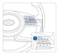
Select the Driving Assist mode by pressing the VIEW MODE 1 button on the steering wheel to display tire pressure.
