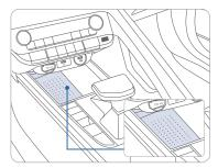
There is a wireless cellular phone charging system inside the front console. The system will operate when all doors are closed, and the ignition switch is in the ACC/ON position. The wireless charging pad is equipped with a cooling fan to help prevent overheating while charging.
