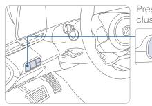
Press - or + to adjust instrument cluster illumination brightness.
