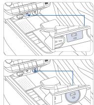
The USB data port can be used to connect an external audio device and listen to it through the audio system in your vehicle.
