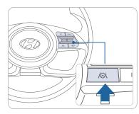
Lane Following Assist detects lane markers on the road using the front view camera mounted on the front windshield. LFA helps to assist the driver steering to help keep the vehicle centered in the lane.
