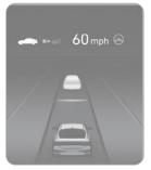
Press the Vehicle distance button to set and maintain the vehicle distance without pressing the accelerator or brake pedal. The vehicle distance will automatically activate previous setting value when you activate SCC.
