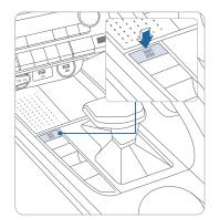
The mode changes, as below, whenever the DRIVE MODE selection switch is toggled up and down. An indicator will illuminate on the instrument cluster when the vehicle is in sport mode or smart mode. When the vehicle is in normal mode, it is not displayed on the instrument cluster.
