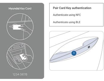
To lock/unlock your vehicle using the NFC key card, hold the key card up to the center of the door handle A.
