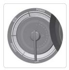
The power gauge indicates whether the current driving condition is fuel efficient or not.
