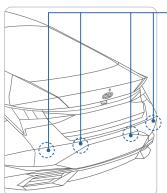
Reverse Parking Distance Warning can warn the driver if an obstacle is detected when the vehicle is moving forward or backward at low speeds.
