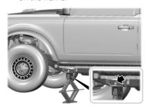
11. Use the rear axle tube for the rear jacking point.
