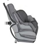
While holding the shoulder and lap belt portions together, route the tongue through the child restraint according to the child restraint manufacturer's instructions. Make sure you did not twist the belt webbing.
