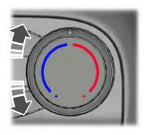
Turn the temperature control counterclockwise for cooler temperature settings.
