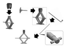
Do not use the extension block when you are changing a flat tire on the rear of the vehicle. Assemble the jack handle using the extensions as shown to operate the jack when placing under the rear axle.
