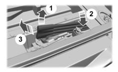
Remove the lug wrench from the tool bag. Turn the spare tire fasteners counterclockwise starting with the lowest first, and remove the spare tire from the rear of the vehicle.
