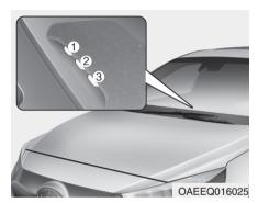
When charging the high voltage battery, the charge level can be checked from outside the vehicle.
