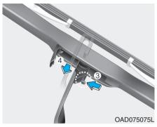
3. While pushing the lock (3), pull down the wiper blade (4).
