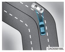
Forward Collision-Avoidance Assist system may recognize a vehicle or pedestrian or cyclist in the next lane or outside the lane when driving on a curved road.
