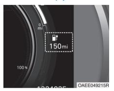
The distance to empty is displayed differently according to the selected drive mode in the Drive Mode Integrated Control System.
