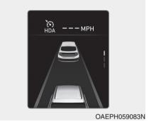
**Temporary deactivation** The A indicator light changes from green to white when the steering wheel control is temporarily deactivated. Even if the steering wheel is not controlled, the distance between the vehicle ahead will be maintained. (For more information of steering wheel control, refer to "Lane Following Assist (LFA)" in this chapter.)
