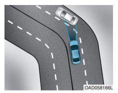
Your vehicle speed can be reduced due to a vehicle in the adjacent lane. Apply the accelerator pedal and select the appropriate set speed. Check to be sure that the road conditions permit safe operation of Smart Cruise Control.
