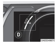
When the system is turned on from the User Settings mode, but the front radar doesn't recognize the vehicle in front, 'AUTO' is displayed in white.
