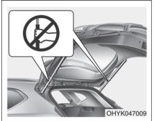
Do not hold the part (gas lifter) that supports the liftgate. Be aware that the deformation of the part may cause vehicle damage and a risk of safety accident.
