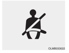
As a reminder to the driver, the seat belt warning light will illuminate and warning chime will sound for approximately 6 seconds each time you turn the POWER button ON if the seat belt is unfastened.
