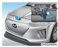
3. Go to the front of the vehicle, raise the hood slightly, push up the secondary latch (1) inside of the hood center and lift the hood (2).
