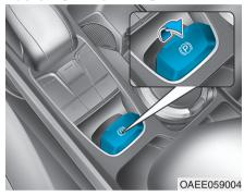
To apply the EPB (Electronic Parking Brake):
