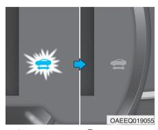
Check if the "= " indicator is turned OFF on the instrument cluster.
