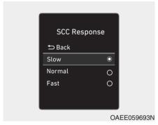
The sensitivity of vehicle speed when following the front vehicle to maintain the set distance can be adjusted. Select 'User Settings  $\rightarrow$  Driver Assistance  $\rightarrow$  SCC Response  $\rightarrow$  Slow/Normal/Fast' in the cluster LCD display.
