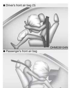
After complete inflation, the air bag immediately starts deflating, enabling the driver to maintain forward visibility and the ability to steer or operate other controls.
