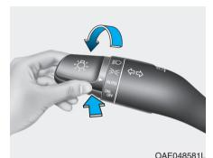
High Beam Assist is a system that automatically adjusts the headlamp range (switches between high beam and low beam) according to the brightness of other vehicles and road conditions.
