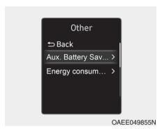
The driver can activate the Aux. Battery Saver+ function by placing the POWER button to the ON position and by selecting:
