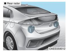
The rear corner radars are located inside the rear bumper for detecting the side and rear areas. Always keep the rear bumper clean for proper operation of the system.
