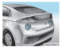
The rear radars are located inside the rear bumper for detecting the side and rear. Always keep the rear bumper clean for proper operation of the system.
