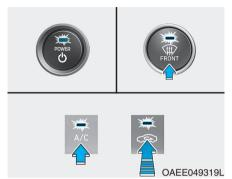
To reduce the probability of fogging up the inside of the windshield, the air intake or air conditioning are controlled automatically according to certain conditions such as or mostition. To cancel or return the defogging logic, do the following.
