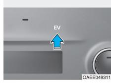
Push the EV button to enter the EV mode on the infotainment system screen.
