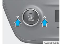
Press the temperature control button to the desired temperature. If the temperature is set to the lowest setting (Lo), the air conditioning system will operate continuously. To turn the automatic operation off, select any button of the following:
