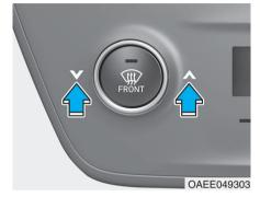
Press the button to increase/ decrease the fan temperature and airflow.
