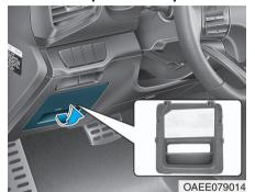
Inside the fuse/relay box cover, you can find the fuse/relay label describing fuse/relay name and capacity.
