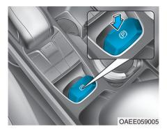
To release EPB (Electronic Parking Brake):
