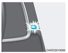
When there are 4~5 gauge bars (near the "L (Low)" area) on the SOC gauge, the warning lamp turns ON to alert you of the battery level.
