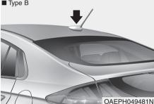
The roof antenna receives both AM and FM broadcast signals, SXM signals (only type B). Rotate the roof antenna in a counterclockwise direction to remove it. Rotate it in a clockwise direction to reinstall it.
