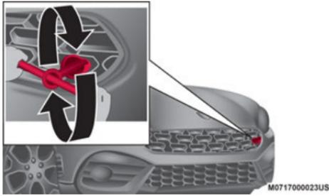
Abarth Installing Front Towing Eye
