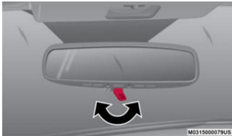
**Mirror Adjustment Lever****Automatic Dimming Mirror – If Equipped**
