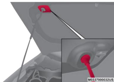
**Inserting Support Rod Into Hole**
