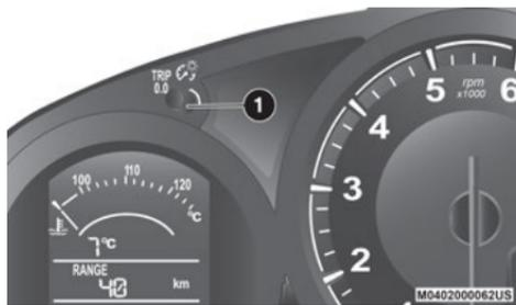
**Odometer/Trip Reset Button**
