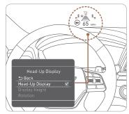
The Head-Up display is a transparent display which projects an image of selected information of the instrument cluster and navigation onto the windshield glass. To activate the head up display, select
