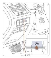
NOTE: LKA Settings can be adjusted in the User Settings page of the instrument cluster under Driving Assist.
