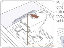
Plug in a USB cable, Auxiliary cable, or other media device to connect an external audio device and listen to it through the audio system in your vehicle.
