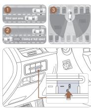
The Blind-Spot Collision Warning (BSW) uses a radar sensor when in Reverse gear to alert the driver of oncoming vehicle(s).
