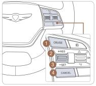
The cruise control system allows you to program the vehicle to maintain a constant speed without holding the accelerator pedal.
