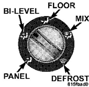
The mode control allows you to choose from several patterns of air distribution. You can select either a primary mode, as identified by the symbols, or a blend of two of these modes. The closer the control is to a particular mode, the more air distribution you receive from that mode.
