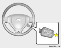
The cruise control system provides automatic speed control for your comfort when driving on freeways, tollroads, or other noncongested highways. This system is designed to function above approximately 25 mph (40 km/h).
