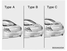
In addition to the lower-mounted rear stoplights on either side of the car, the high mounted rear stoplight in the center of the rear window or inserted in the rear spoiler also lights when the brakes are applied.
