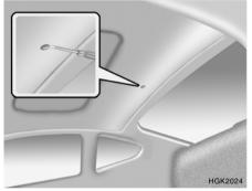
1. Remove the cap located in the rear roof panel by using a coin or screw driver.
