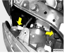
4. Disconnect the power cord from the bulb base in the back of the headlight.
