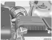
To change the filter, unsnap the clips around the cover. When this is done, the cover can be lifted off, the old filter removed and the new filter put in its place. Genuine Hyundai Replacement Parts are recommended.
