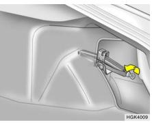
The jack is located behind the right side of luggage trim. Remove the jack cover by unscrewing the bolts. Turn the jack end counterclockwise to lower the jack height by using a screw driver or wrench bar and remove it from the bracket.
