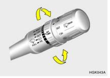
To use the intermittent wiper feature, place the wiper switch in the "INT" position. With the switch in this position, the interval between wipes can be varied from 2 to 10 seconds by turning the interval adjuster barrel.
