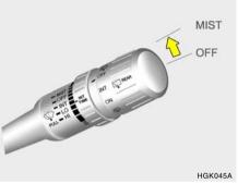
If a single wipe is desired in mist, move the windshield wiper and washer control lever up.
