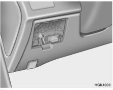
The fuse box for the lights and other electrical accessories will be found low on the dashboard on the driver's side. Inside the box you will find a list showing the circuits protected by each fuse.
