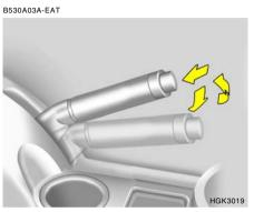
The parking brake must always be set when the vehicle is to be left unattended. When the parking brake is applied, and the ignition key is at the "ON" position, the parking brake warning lamp will be illuminated. Before driving the vehicle, the parking brake must be fully released and the warning lamp extinguished.
