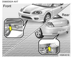
For emergency towing when no commercial tow vehicle is available, attach a tow cable, chain or strap to one of the towing hooks under the front /rear of your car. Do not attempt to tow your vehicle in this manner on any unpaved surface. This could result in serious damage to your car.
