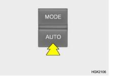
The FATC (Full Automatic Temperature Control) system automatically controls heating and cooling as follows:
