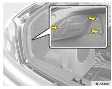
To remove the cover of the rear luggage trim, turn the knob by hand to the counterclockwise.
