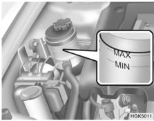
The power steering fluid level should be checked regularly. To check the power steering fluid level, be sure the engine is "OFF", then check to make certain that the power steering fluid level is between the "MAX" and "MIN" level markings on the fluid reservoir.
