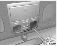
1. Remove the cover with a flat-blade screwdriver.
