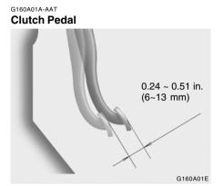
With the engine off, press lightly on the clutch pedal until you feel a change in resistance. This is the clutch pedal free-play. The free-play should be within the limits specified in the illustration. If it is not, have it inspected by your Hyundai dealer and adjusted or repaired if necessary.
