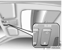
The sunroof can be electrically opened or closed with the ignition key in the "ON" position. The sunroof is moved to its fully open position by pushing the " $\uparrow$ " switch, and to stop at the desired position, push in any switches ( $\uparrow$ ),  $\clubsuit$ , Up, Down). To close, press and hold the " $\clubsuit$ " button. Release the button when the sunroof reaches the desired position.
