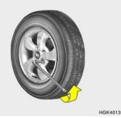
The wheel nuts should be loosened slightly before raising the car. To loosen the nuts, turn the wrench handle counterclockwise. When doing this, be sure that the socket is seated completely over the nut so it cannot slip off. For maximum leverage, position the wrench so the handle is to the left as shown in the drawing. Then, while holding the wrench near the end of the handle, push down on it with steady pressure. Do not remove the nuts at this time. Just loosen them about one-half turn.
