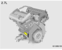
The engine number is stamped on the engine block as shown in the drawing.
