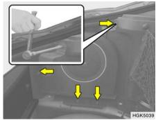
3. Extract the mounting screws (10mm) around the woofer speaker with a spaner.
