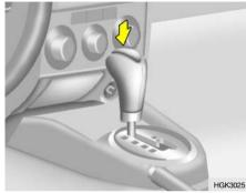
Park the car on level ground with the parking brake engaged. When the transaxle fluid level is checked, the transaxle fluid should be at normal operating temperature and the engine idling.
