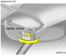
Your Hyundai is equipped with sun visors to give the driver and front passenger either frontal or sideward shade. To reduce glare or to shut out direct rays of the sun, turn the sun visor down. A vanity mirror is provided on the back of the sun visor for the front passenger.
