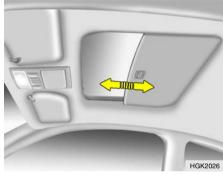
The sunshade can be opened and closed by sliding it forward or rearward when the sunroof is closed. The sunshade will open automatically when the sunroof is opened, but it must be closed manually.
