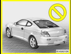
For the safety of all passengers, luggage or other cargo should not be piled higher than the top of the seatback. In addition, do not place objects on the rear shelf as they may move forward during braking or in an accident and strike vehicle passengers.
