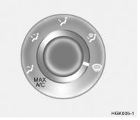
This is used to direct the flow of air. Air can be directed to the floor, instrument panel outlets, or windshield. Five symbols are used to represent Face, Bi-Level, Floor, Floor-Defrost and Defrost air position. The MAX A/C mode is used to cool the inside of the vehicle faster.
