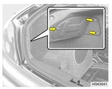
5. To remove the cover of the rear luggae trim, turn the knob by hand to the counterclock-wise.
