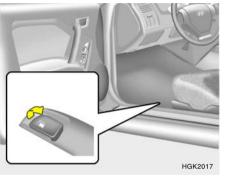
The fuel-filler lid may be opened from inside the vehicle by pulling up on the fuel-filler lid opener located on the front floor area on the left side of the vehicle.
