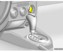
The highly efficient Hyundai automatic transaxle has four forward speeds and one reverse speed. The individual speeds are selected automatically, depending on the position of the speed selector lever. The selector lever has 2 gates; the main gate and the manual gate.
