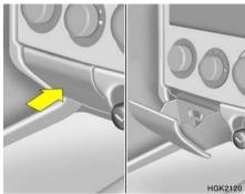
The front ashtray may be opened by pushing and releasing the ashtray door at its top edge. To remove the ashtray in order to clean it, the metal ash receptacle should be lifted out from the ashtray door. Do not attempt to remove the entire ashtray door assembly or damage will result. To reinstall it, place it in the proper position and press it down in the ashtray door. The ashtray lamp will only illuminate when the exterior body lights are switched on.
