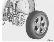
Loosen the wheel nuts and remove them with your fingers. Slide the wheel off the studs and lay it flat so it cannot roll away. To put the wheel on the hub, pick up the spare tire, line up the holes with the studs and slide the wheel onto them. If this is difficult, tip the wheel slightly and get the top hole in the wheel lined up with the top stud. Then jiggle the wheel back and forth until the wheel can be slid over the other studs.
