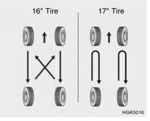
Tires should be rotated every 6,000 miles (10,000 km). If you notice that tires are wearing unevenly between rotations, have the car checked by a Hyundai dealer so the cause may be corrected.
