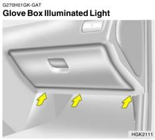
1. Remove the mounting screws on the downside of the glove box.
