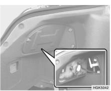
6. Remove the nut (8mm) with a wrench.
