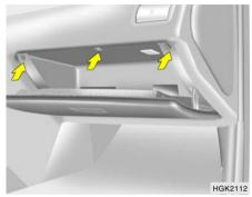
2. Open the glove box and remove the mounting screws on the upside of the glove box.
