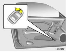
To open the tail gate without using the key, pull up the lid release lever located on the driver's door panel.
