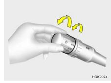
To operate the headlights, turn the barrel on the end of the multi-function switch. The first position turns on the parking lights, sidelights, tail lights and instrument panel lights. The second position turns on the headlights.
