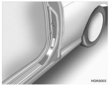
Tire label located on the driver's side of the center pillar outer panel gives the cold tire pressures recommended for your vehicle with the original tire size, the number of people that can be in your vehicle and vehicle capacity weight.
