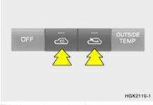
This is used to select fresh outside air or recirculation inside air.
