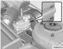
The fluid level in the brake fluid reservoir should be checked periodically. The level should be between the "MIN" and "MAX" marks on the side of the reservoir. If the level is at or below the "MIN" mark, carefully add fluid to bring it up to "MAX". Do not overfill. G120E02A-AAT
