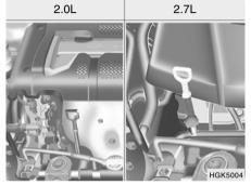
Before checking the oil, warm up the engine to the normal operating temperature and be sure your car is parked on level ground. Turn the engine off.
