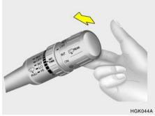
To use the windshield washer, pull the wiper/ washer lever toward the steering wheel. When the washer lever is operated, the wipers automatically make two passes across the windshield. The washer continues to operate until the lever is released.
