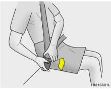
The seat belt is released by pressing the release button in the locking buckle. When it is released, the belt should automatically draw back into the retractor.
