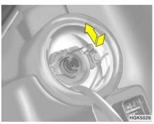
7. Push the bulb spring to remove the headlight bulb.
