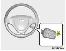
The vehicle will automatically resume the speed set prior to cancellation when you push the control switch upward to "RESUME (ACCEL)" position and release it, providing the vehicle speed is above 25 mph (40 km/h).
