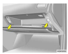
3. Remove the glove box by pulling strongly.
