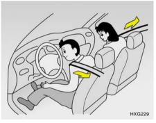
When the vehicle stops suddenly, or if the occupant tries to lean forward too quickly, the seat belt retractor will lock into position. In certain frontal collisions, the pre-tensioner will activate and pull the seat belt into tighter contact against the occupant's body.
