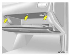
2. Open the glove box and remove the mounting screws on the upside of the glove box.
