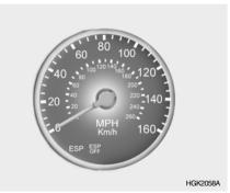
Your Hyundai's speedometer is calibrated in miles per hour (on the outer scale) and kilometers per hour (on the inner scale).
