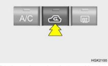
This is used to select fresh outside air or recirculating inside air.
