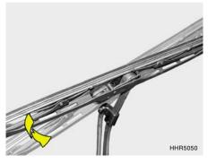
1. Put a new wiper blade onto the wiper arm and lower the wiper blade at the level of the wiper arm as shown in the drawing.
