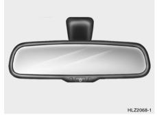
The electric type day/night inside rearview mirror automatically controls the glare of headlights of the car behind you.
