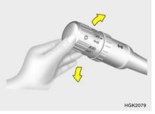
To indicate a lane change, move the lever up or down to a point where it begins flashing. The lever will automatically return to the center position when released.
