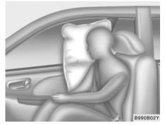
Your Hyundai is equipped with a side impact airbag in each front seat. The purpose of the airbag is to provide the vehicle's driver and/or the front passenger with additional protection than that offered by the seat belt alone. The side impact airbags are designed to deploy only during certain side-impact collisions, depending on the crash severity, angle, speed and point of impact. The side impact airbags are not designed to deploy in all side impact situations.
