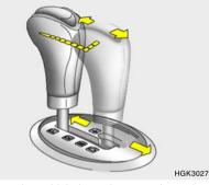
Whether the vehicle is stationary or in motion, sports mode is selected by pushing the selector lever from the "D" position into the manual gate. To return to "D" range operation, push the selector lever back into the main gate.
