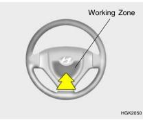
Press the pad on the steering wheel to sound the horn.
