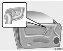
The doors can be locked without a key. To lock the doors first push the inside lock switch to the "LOCK" position so that the red mark on the switch is not visible, then close the door.
