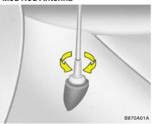
Your car uses a fixed rod antenna to receive both AM and FM broadcast signals. This antenna is a removable type. To remove
