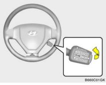
To disengage the cruise control system, pull the control switch toward the steering wheel to "CANCEL" position.
