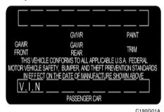
The compliance label is located on the driver's side of the center piller outer panel.
