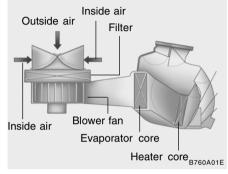
The climate control air filter is located in front of the blower uniit behind the glove box. It operates to decrease the amount of pollutants
