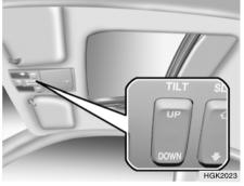
The sunroof can be tilted by pushing the "UP" button with the sunroof closed. Release the button when the sunroof reaches the desired position. To close the sunroof, press the "DOWN" button.
