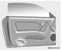
A red light comes on when the front door is opened. The purpose of this light is to assist when you get in or out and also to warn passing vehicles.
