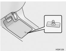
When using a floor mat on the front floor carpet, make sure it attaches to the floor mat anchor in your vehicle. This keeps the floor mat from sliding forward.
