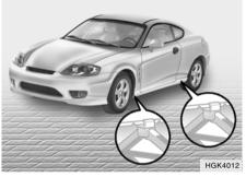
The base of the jack should be placed on firm, level ground. The jack should be positioned as shown in the drawing.
