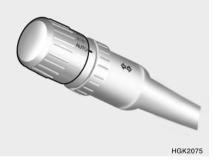
To operate the automatic light feature, turn the barrel on the end of the multi-function switch. If you set the multi-function switch to "AUTO", the tail lights and headlights will be turned automatically on or off according to external illumination.
