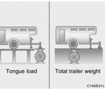
Tongue loads can be increased or decreased by redistributing the load in the trailer. This can be verified by checking the total weight of the loaded trailer and then checking the load on the tongue.
