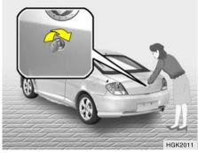
To open the tail gate, insert the key and turn it clockwise to unlock. The tail gate compartment light illuminates when the tail gate is opened.
