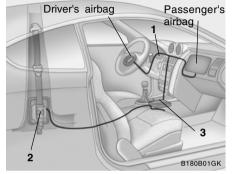
The seat belt pre-tensioner system consists mainly of the following components.
