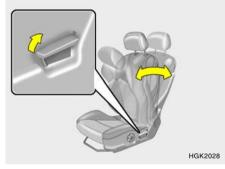
To recline the seatback, lean forward to take your weight off it, then pull up on the recliner control lever at the outside edge of the seat. Now lean back until the desired seatback angle is achieved. To lock the seatback into position, release the recliner control lever.
