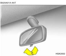
Your Hyundai is equipped with a day/night inside rear view mirror. The "night" position is selected by flipping the tab at the bottom of the mirror toward you. In the "night" position, the glare of headlights of cars behind you is reduced.
