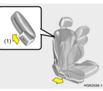
By pulling up the walk in device lever (1) at the right-upper side of the passenger side seatback, the seatback will tilt forward. Then push the seat forward to allow the occupants to enter.
