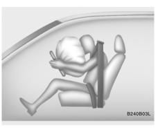
A fully inflated airbag in combination with a properly worn seat belt slows the driver's or the passenger's forward motion, thus reducing the risk of head and chest injury.
