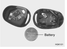
2. Remove the old battery from the case and note the polarity. Make sure the polarity of the new battery is the same(+side facing up), then insert it in the transmitter.
