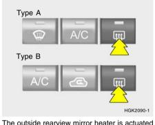
In control of the rearview mirror neater is actuated in connection with the rear window defroster. To heat the outside rearview mirror glass, push in the switch for the rear window defroster. The rearview mirror glass will be heated for defrosting or defogging and will give you improved rear vision in inclement weather conditions. Push the switch again to turn the heater off. The outside rearview mirror heater automatically turns itself off after 15 minutes.
