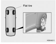
Block the wheel that is diagonally opposite from the flat to keep the vehicle from rolling when the car is raised on the jack.
