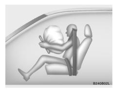
The airbag modules are located both in the center of the steering wheel and in the front passenger's panel above the glove box. When the SRSCM detects a considerable impact to the front of the vehicle, it will automatically deploy the airbags.
