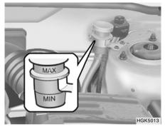
CHECKING THE CLUTCH FLUID
