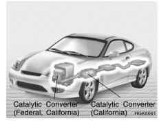
All Hyundai vehicles are equipped with a monolith type three-way catalytic converter to reduce the carbon monoxide, hydrocarbons and nitrogen oxides contained in the exhaust gas. Exhaust gases passing through the catalytic converter may cause it to operate at a very high temperature. The introduction of large amounts of unburned gasoline into the exhaust may cause the catalytic converter to overheat and create a fire hazard. This risk may be reduced by observing the following:
