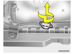
Turn the radiator cap counterclockwise without pressing down on it, until it stops. This relieves any pressure remaining in the cooling system. And remove the radiator cap by pushing down and turning counterclockwise.
